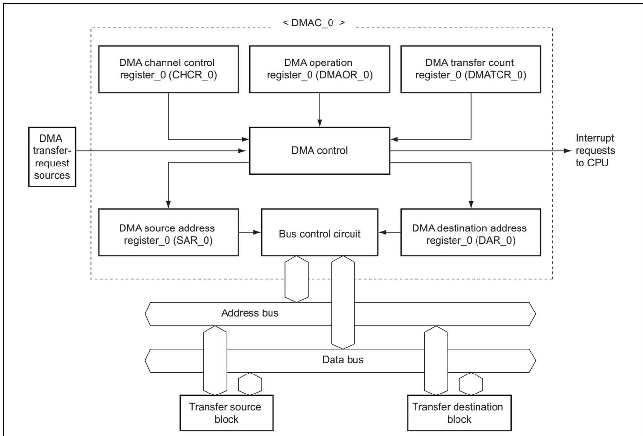
Figure 2 DMAC Block Diagram (ch0)
