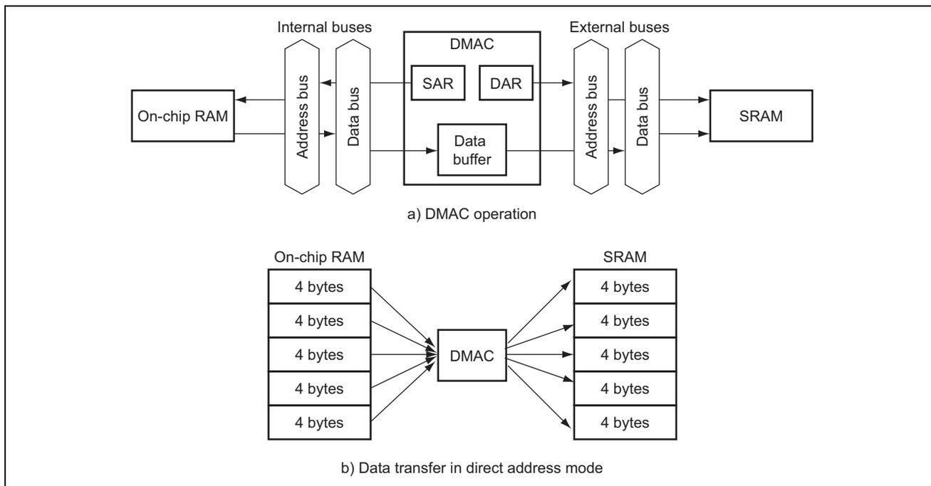
**Figure 1 Data Transfer Using DMAC**
