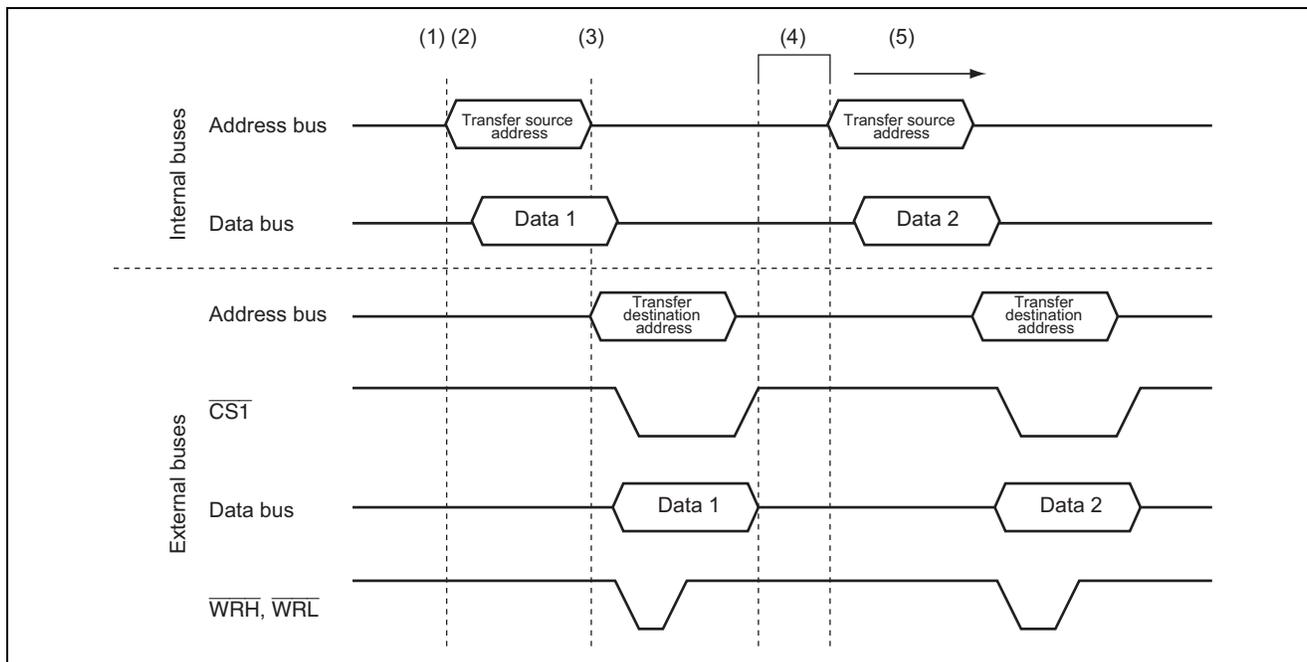
**Figure 3 Operation by Direct Address Transfer in Dual Address Mode**
