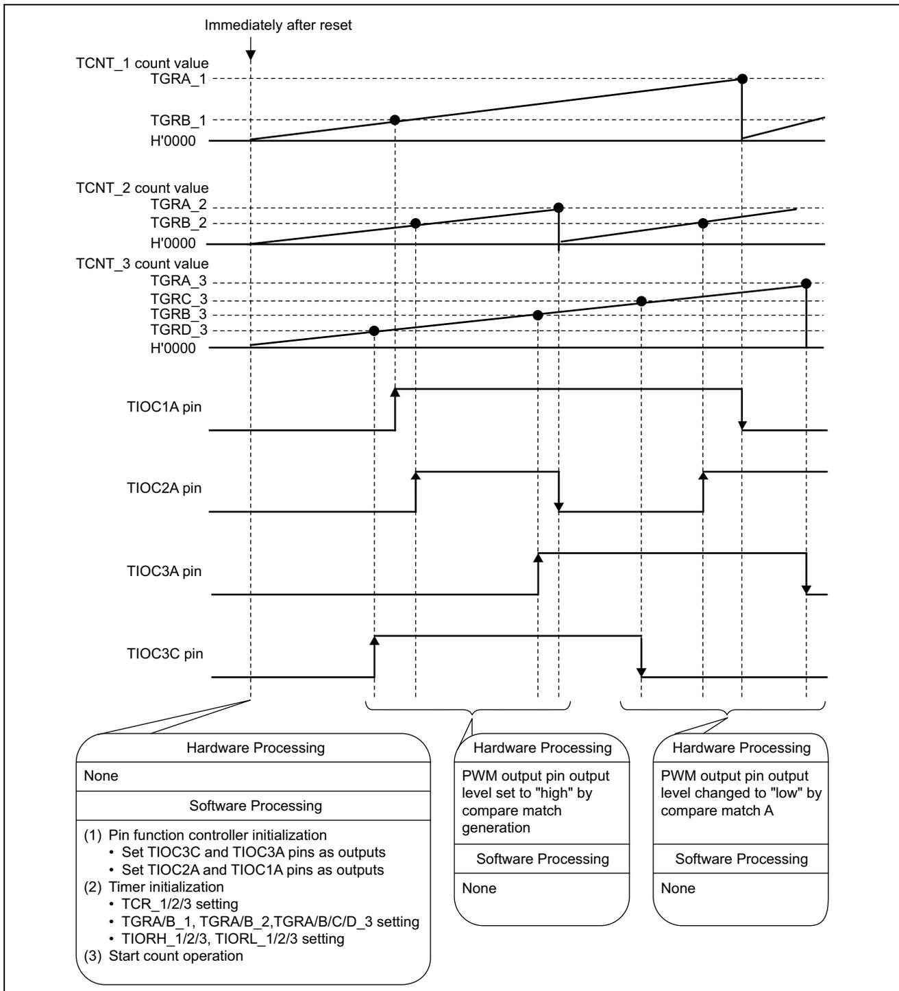
Figure 3 Principles of Operation of PWM Waveforms
