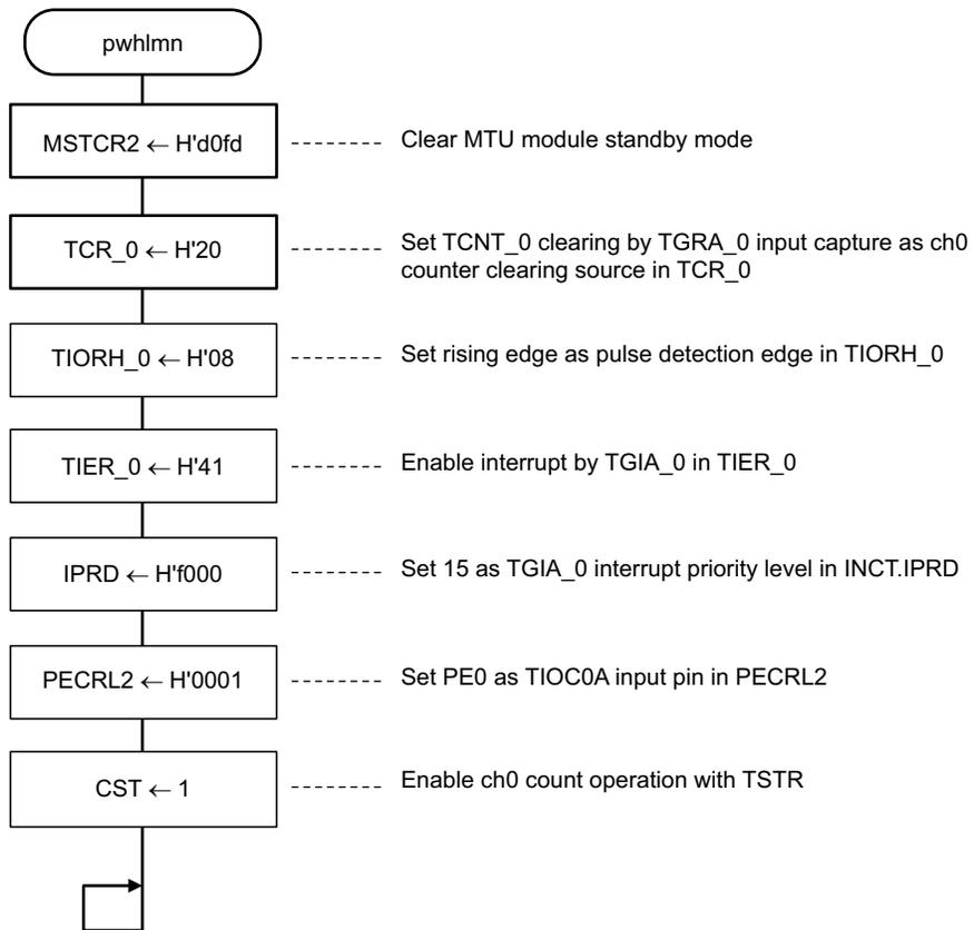
(2) Pulse high and low width measurement
