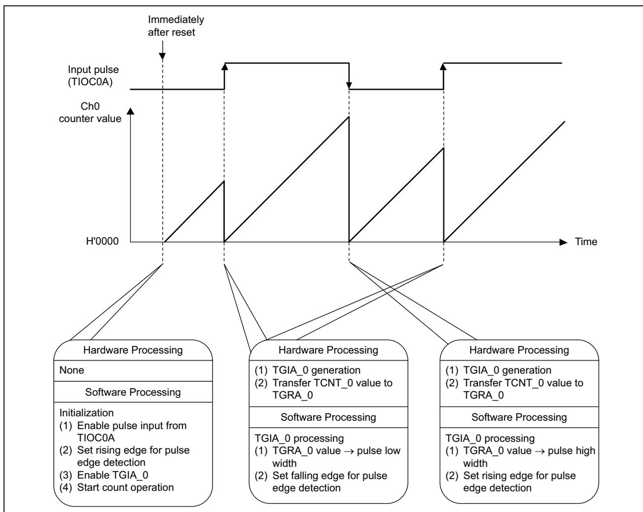
**Figure 3 Principles of Operation of Pulse Width Measurement**
