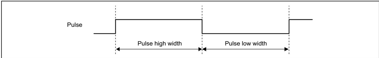
Figure 1 Pulse Width Measurement Timing
