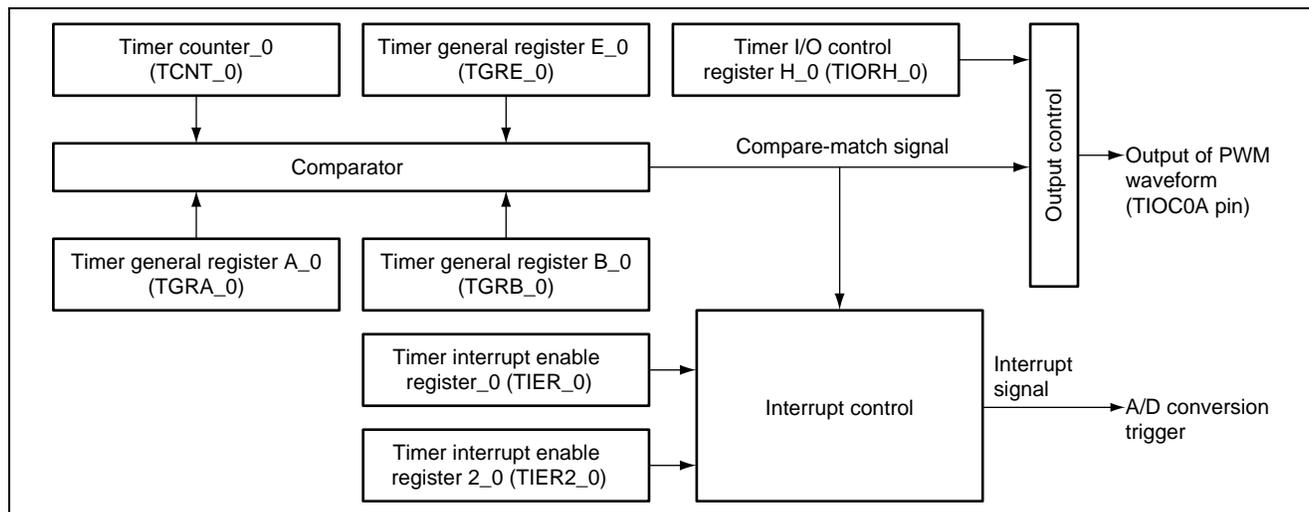
**Figure 3 Block Diagram of MTU2 ch0**
