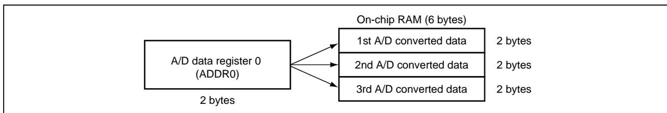
**Figure 2 Storing A/D Converted Data to On-chip RAM**
