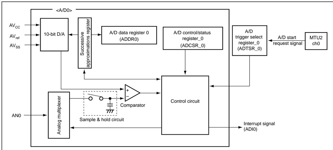
**Figure 4 Block Diagram of A/D Module 0**
