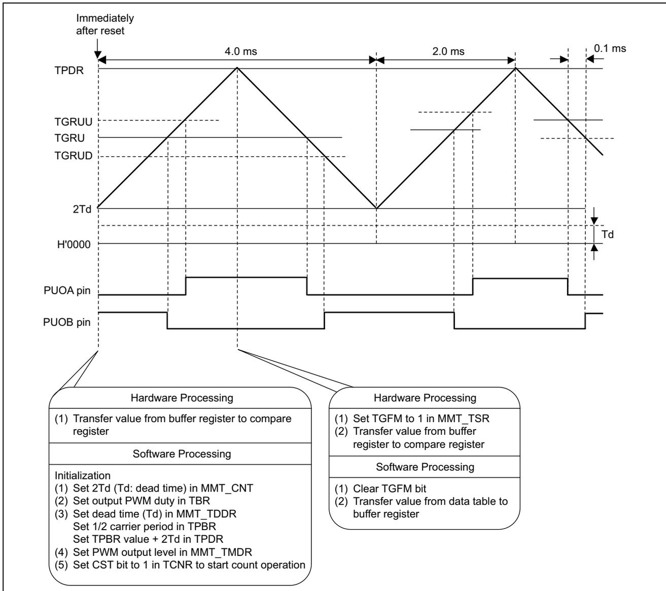
**Figure 3 Principles of Operation of Complementary PWM Waveform Output**
