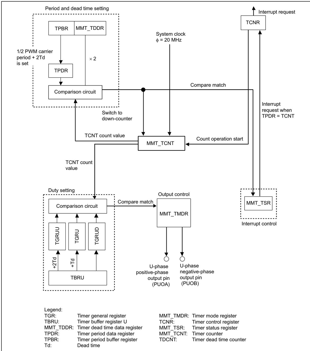
Figure 2 MTU U-Phase Block Diagram
