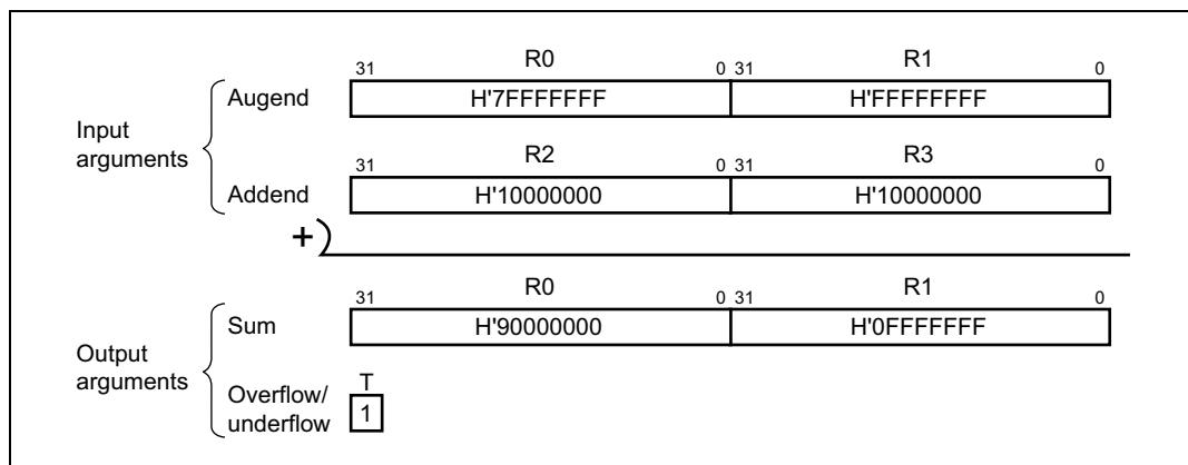
Figure 1 Software ADDS64 Execution Example
