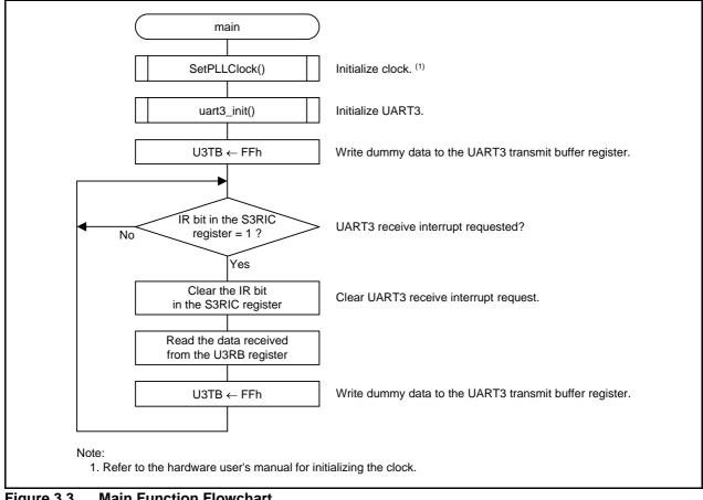
Figure 3.3 **Main Function Flowchart**
