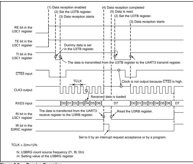
Figure 3.2 Receive Operation
