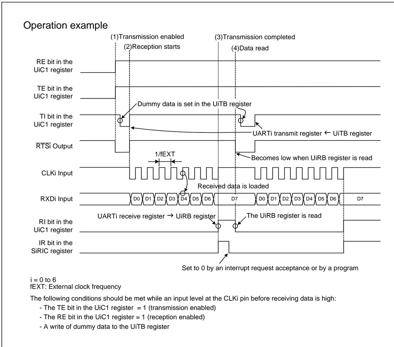
Figure 3.2 Receive Operation Timing
