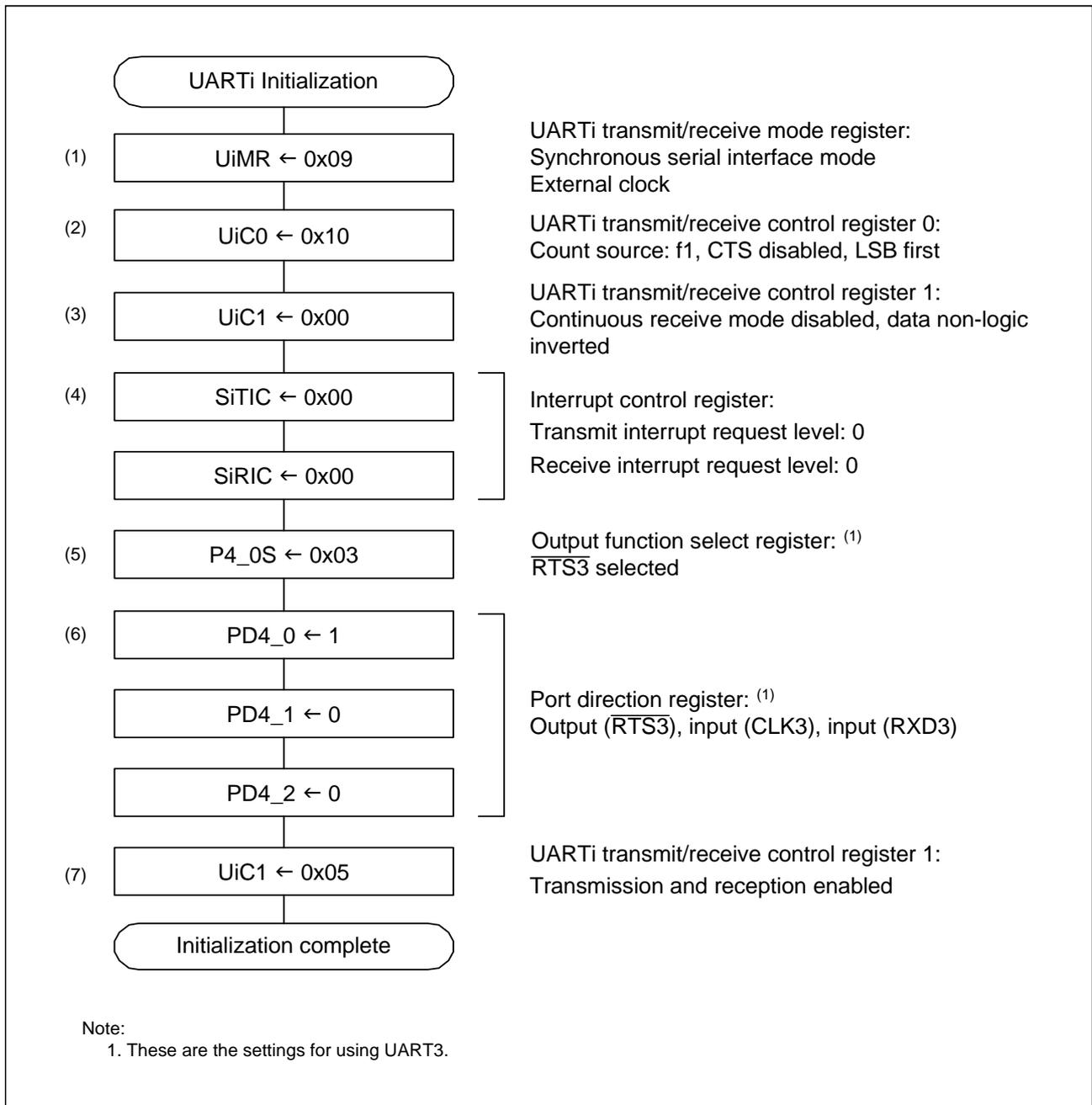
Figure 3.4 UARTi Initialization Process Flowchart (i = 0 to 6)
