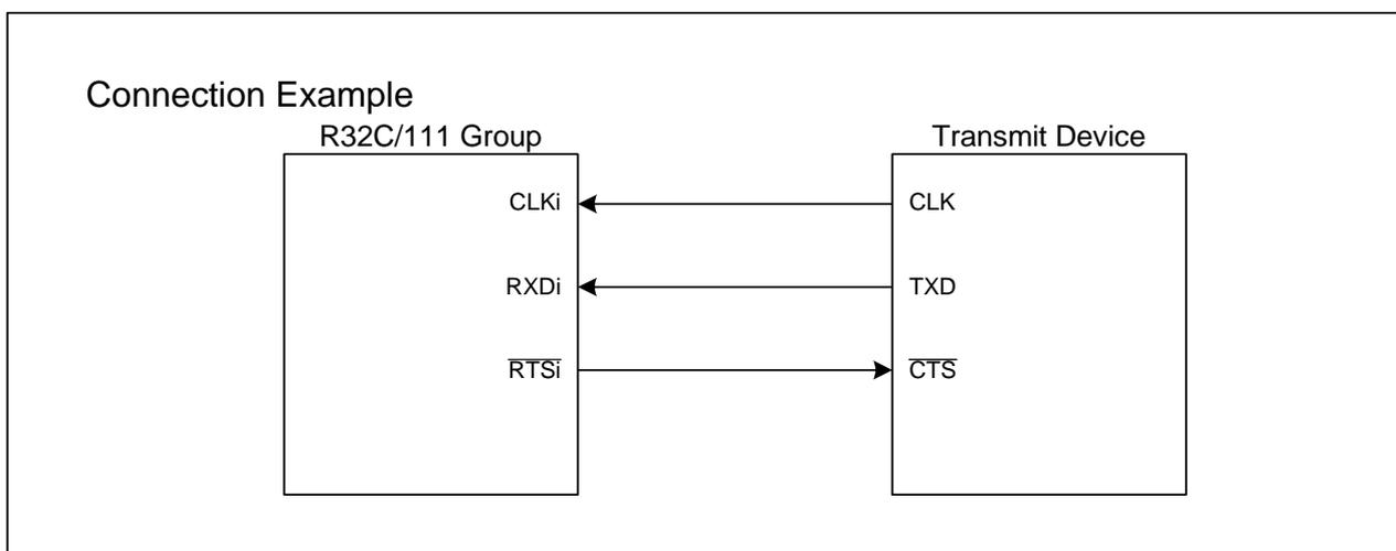
**Figure 3.1** Receive Connection Example
