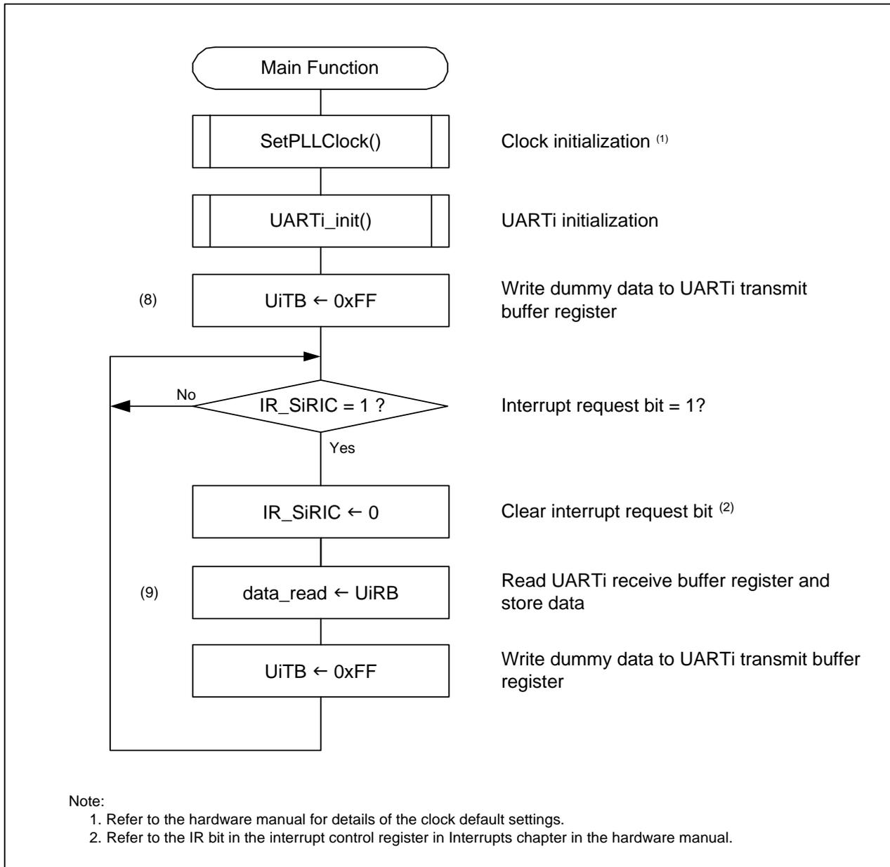
Figure 3.3 Main Process Flowchart (i = 0 to 6)
