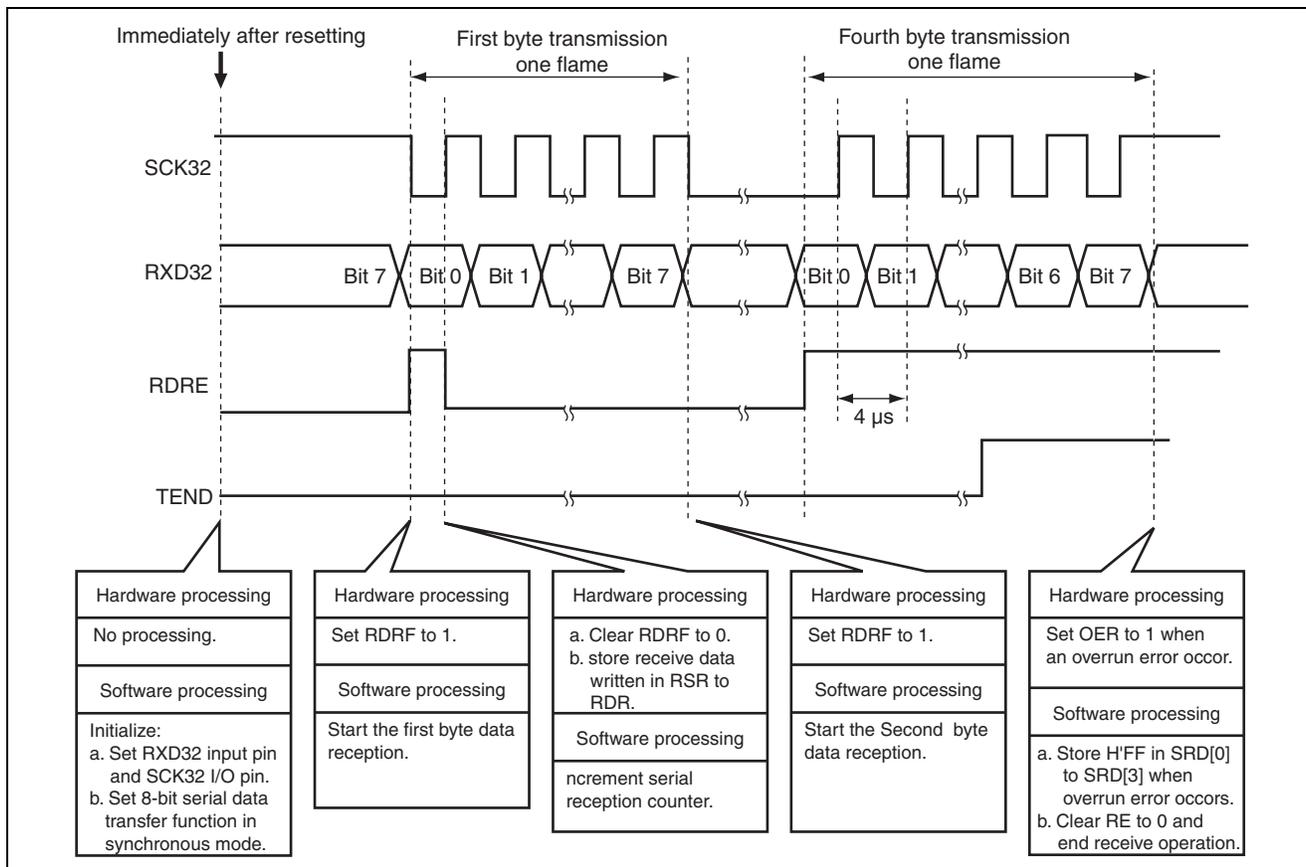
Figure 3.1 Operation Principle of Serial Data Reception in Synchronous mode
