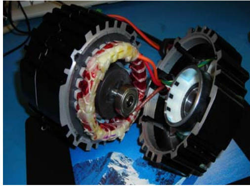
Figure 14 A physical BLDC motor for parameter tuning
