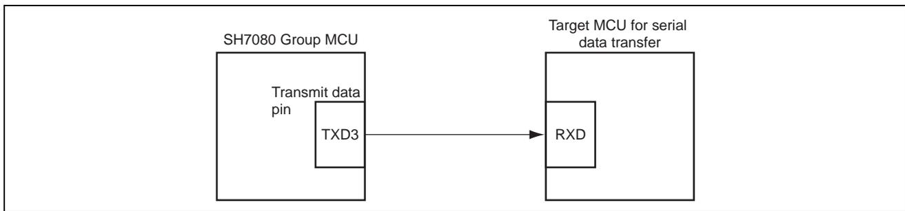
**Figure 1 Asynchronous Serial Data Transmission with FIFO**
