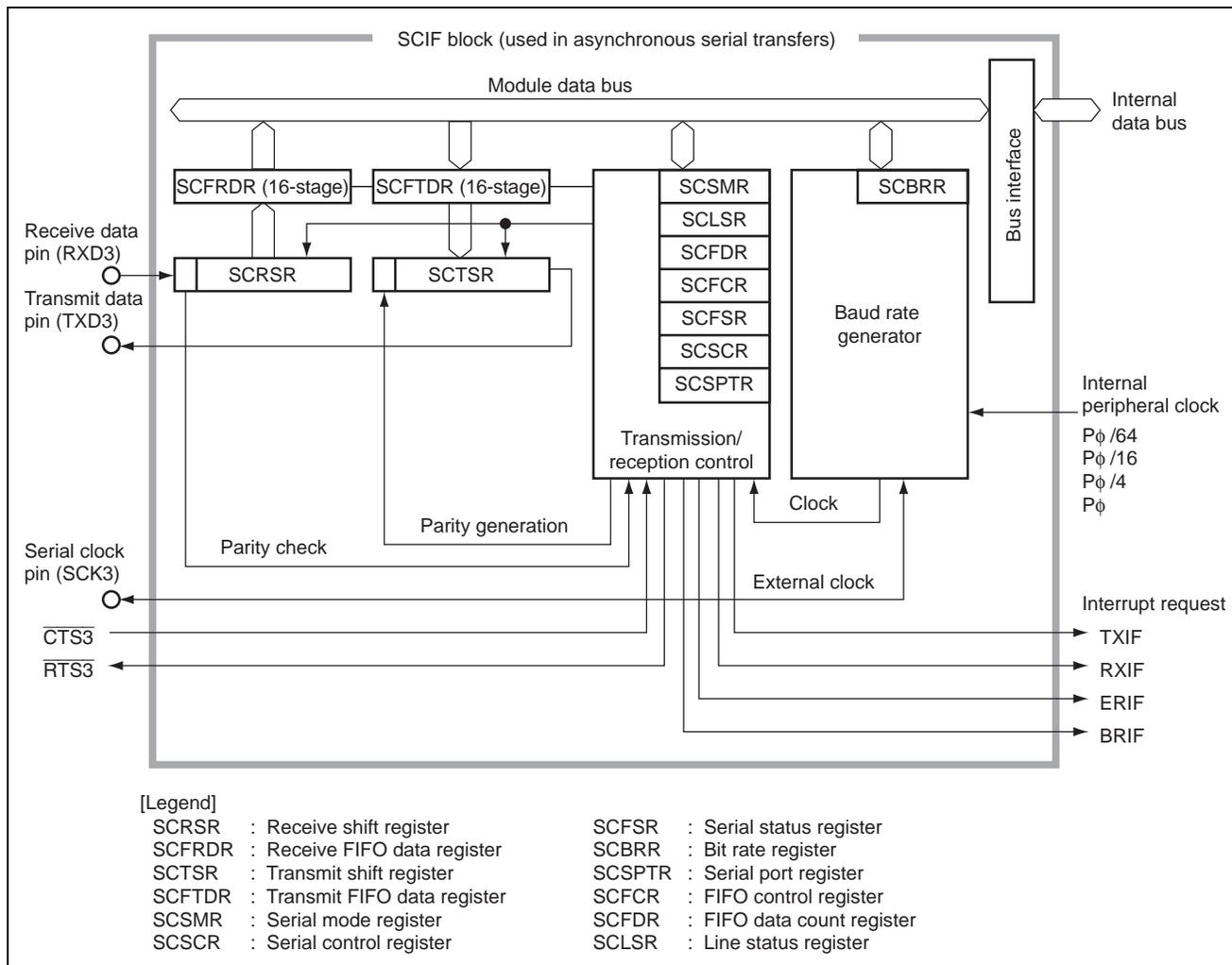
**Figure 2 Block Diagram of SCIF (Serial Communication Interface with FIFO)**
