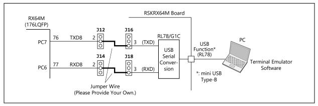
Figure 5.1 Jumper Setting for RSKRX64M Board (Overview)
