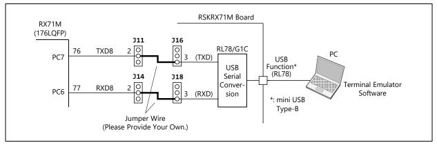
Figure 5.2 Jumper Setting for RSKRX71M Board (Overview)
