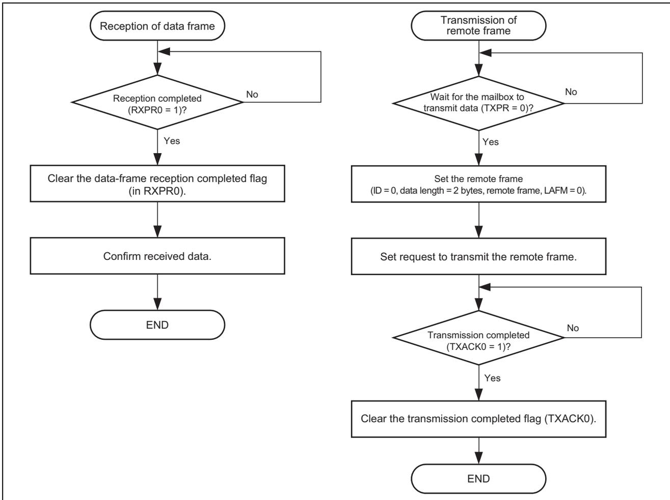
Figure 7 Example of Flow of Processing by the Sample Program (2)
