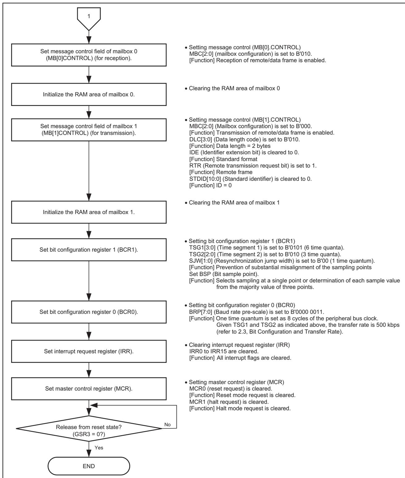
**Figure 3 Example of Initialization Flow for the RCAN-ET Module (2)**
