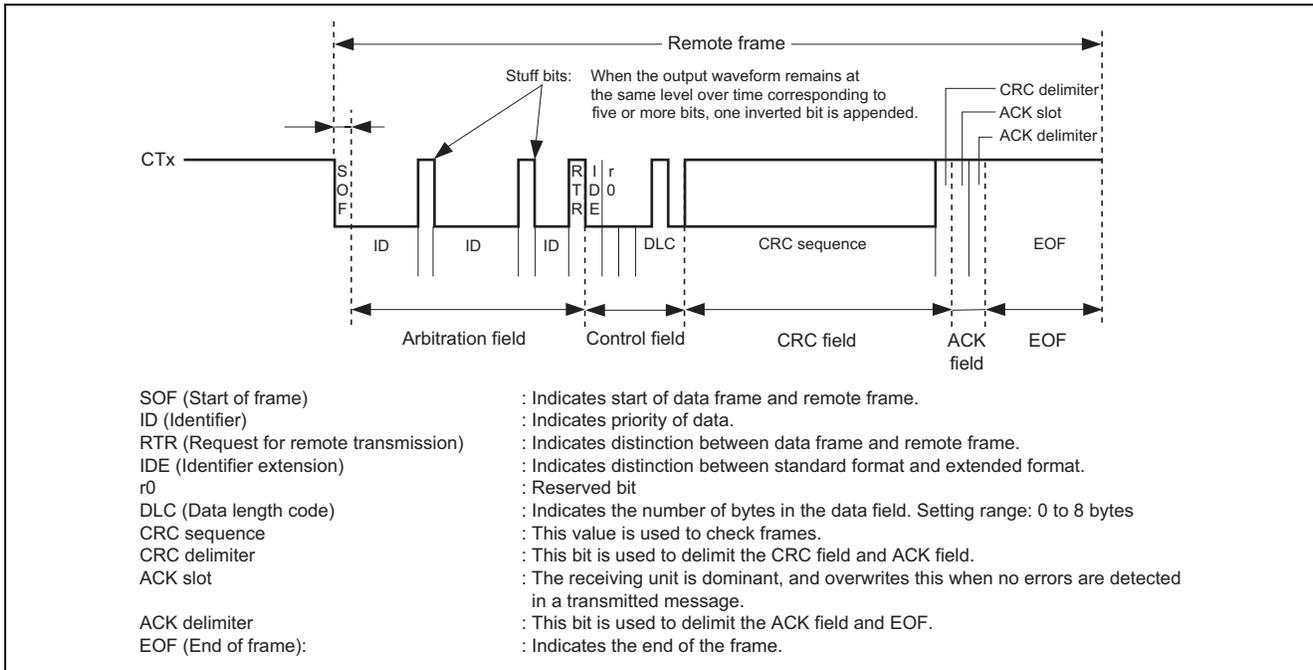
**Figure 5 Waveform for Remote Frame Transmission by the RCAN-ET**
