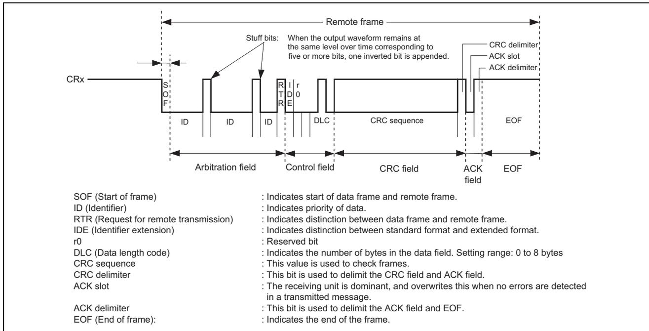
Figure 5 Waveform for Remote Frame Reception by the RCAN-ET
