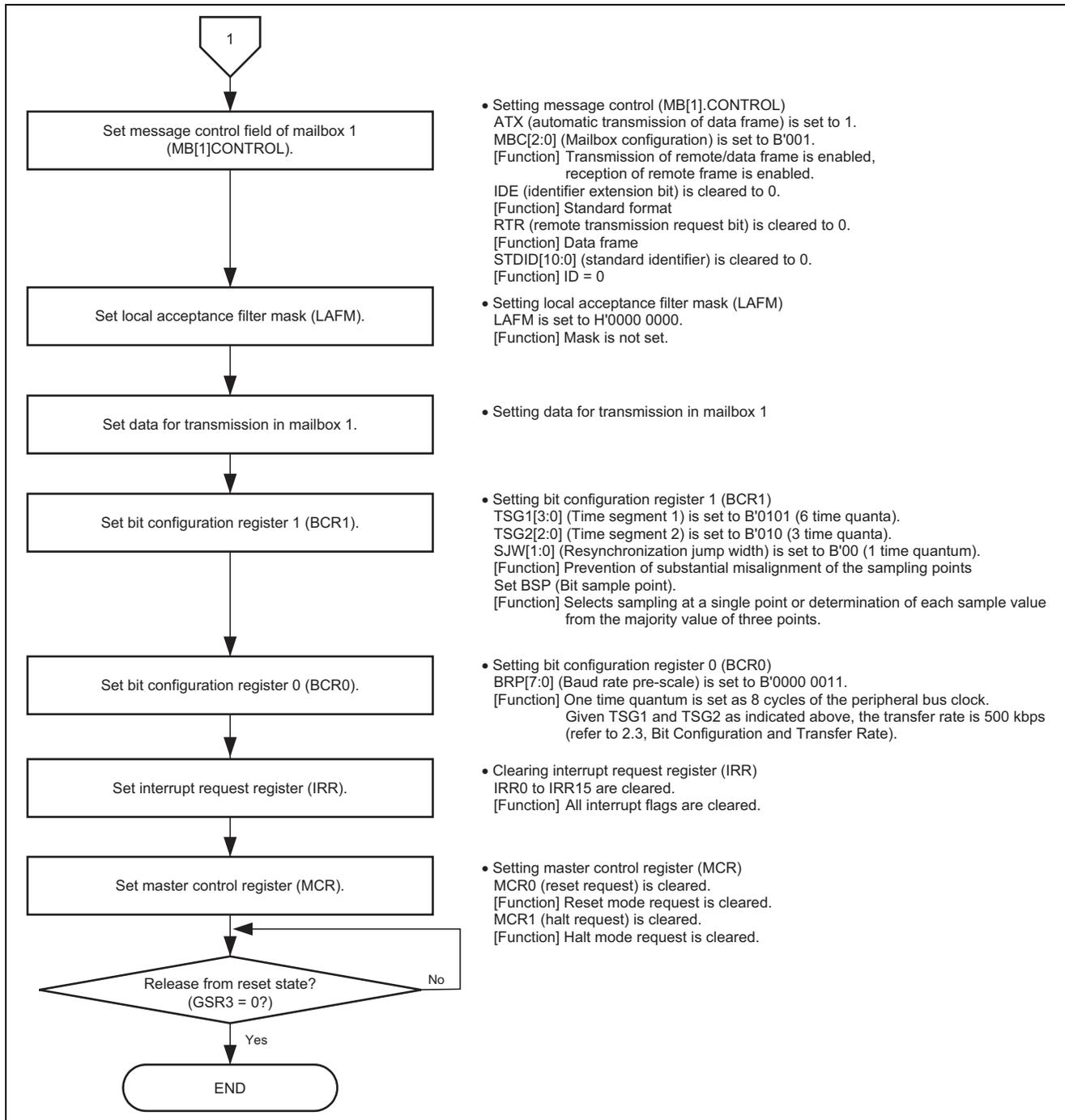
**Figure 3 Example of Initialization Flow for the RCAN-ET Module (2)**
