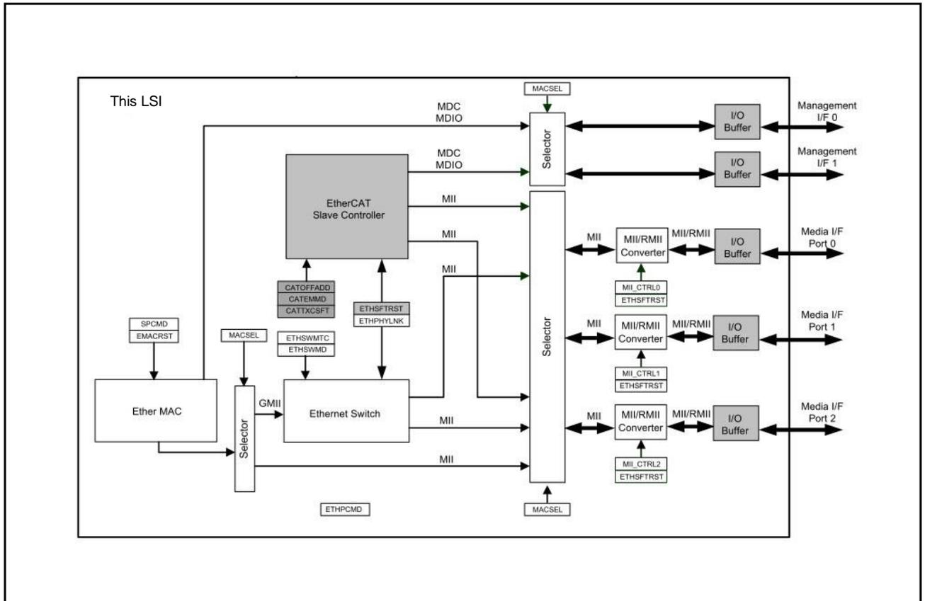
Figure 4.1 Diagram of Blocks Involved in Ethernet Communications
