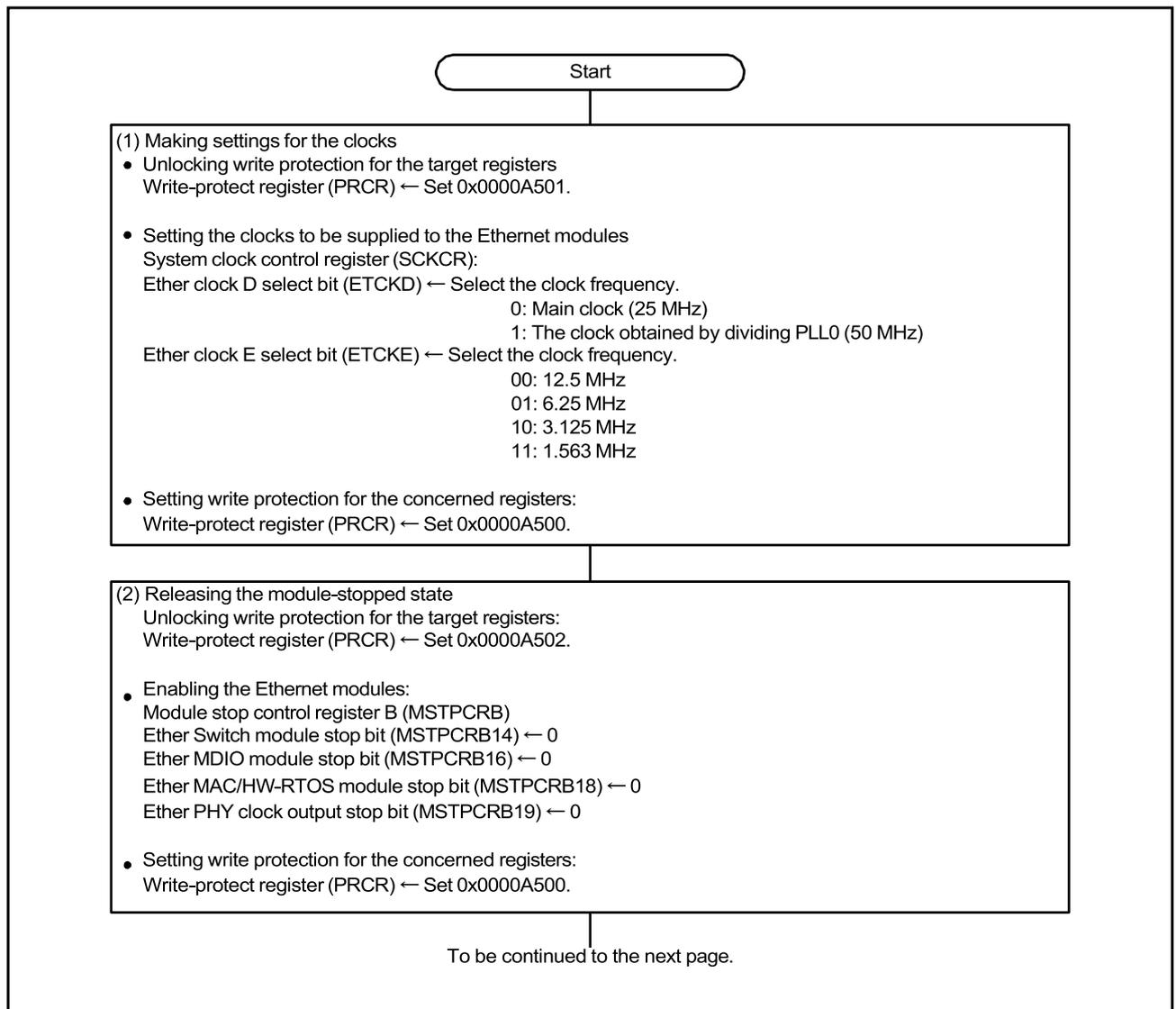
**Figure 5.1 Flow of Initialization of the Ethernet MAC (1)**
