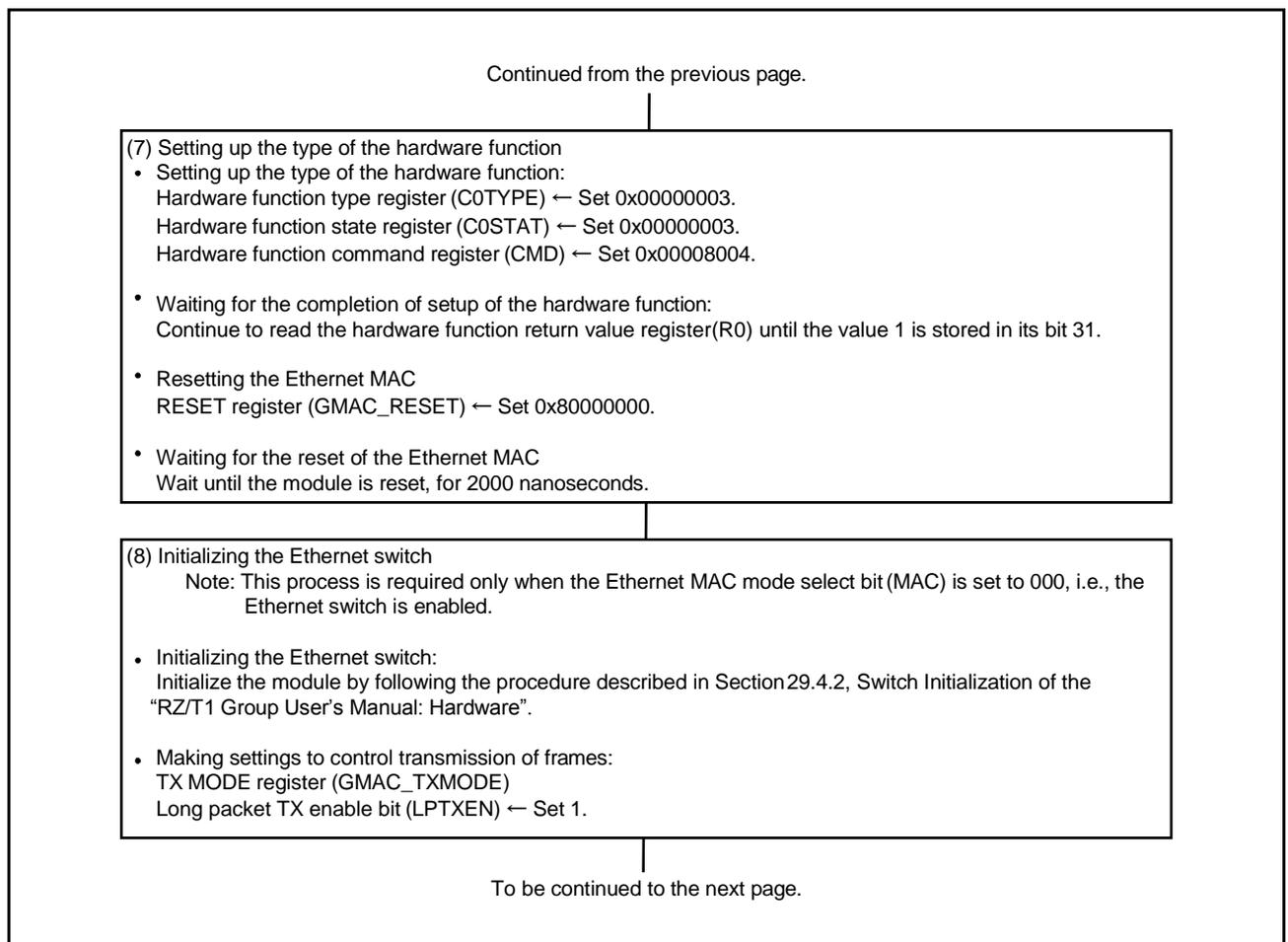
**Figure 5.4** Flow of Initialization of the Ethernet MAC (4)
