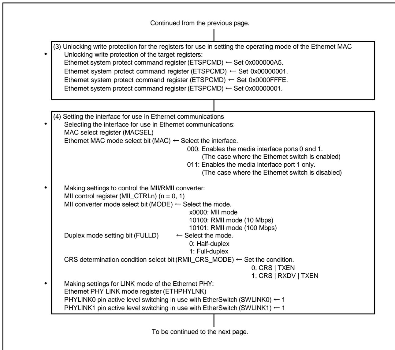
**Figure 5.2 Flow of Initialization of the Ethernet MAC (2)**
