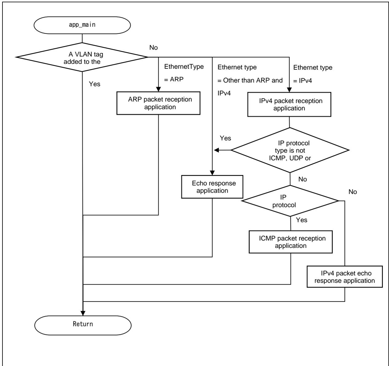
Figure 6.3 Main Processing for the Ethernet Frame Reception Application (app\_main)
