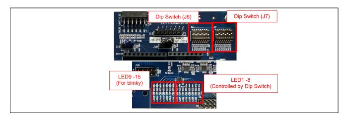
When the sample application is executed, LED9 - LED15 blink. LED1 – LED8 are turned ON/OFF depending on the state of Dip Switch (J6).
