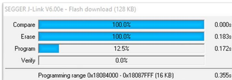
Once the SPI flash has been reprogrammed the new code will be executed on device reset. The boot loader will determine if the user code needs to be relocated into RAM or executed in place from SPI as this is specified in the linker file. Details on the boot loader application can be found in the following document (QSPI Flash Boot Loader) found on the product website.
