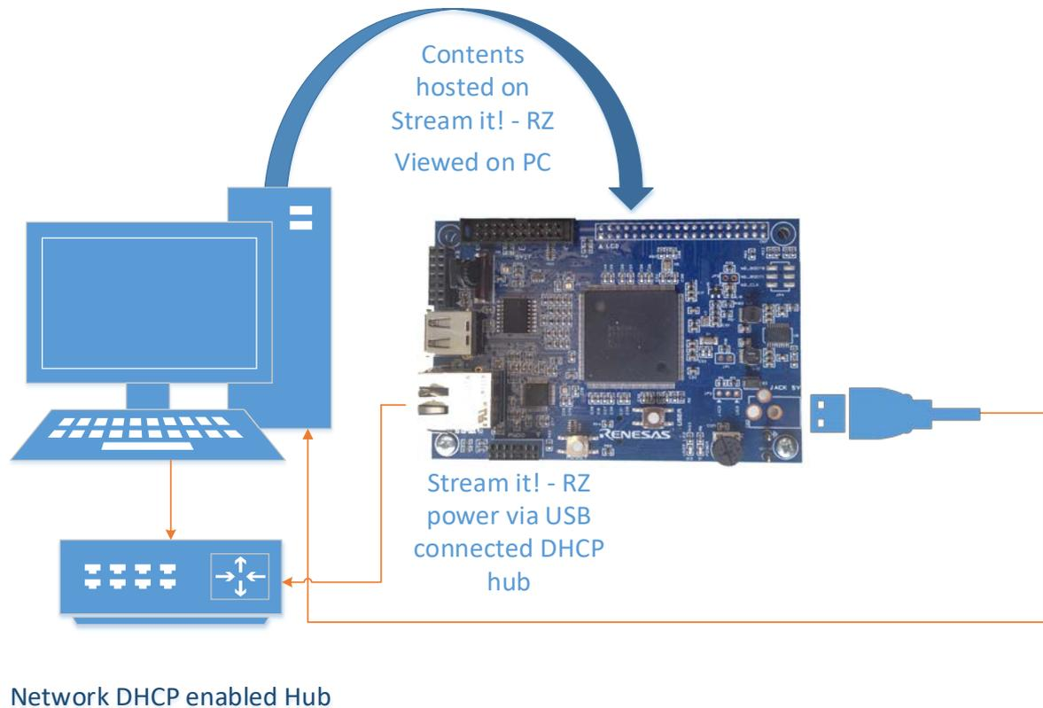
**Figure 1 Hardware configuration of the Stream it! - RZ**
