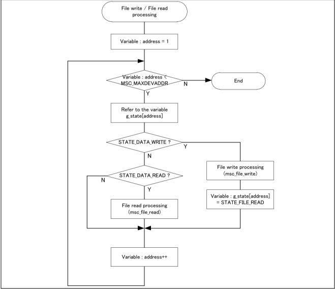
Figure 9-2 File read/write processing
