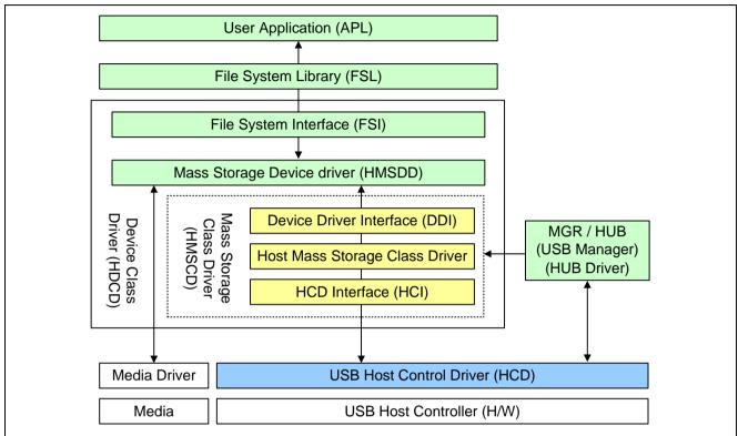
Figure 2-1 Software Block Diagram
