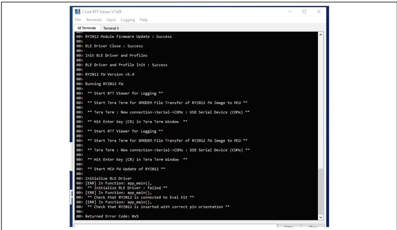
Figure 25. Init BLE Driver Failed
