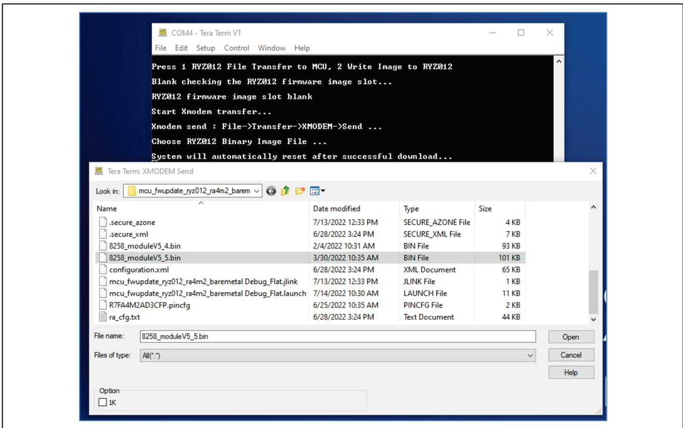
Figure 14. Tera Term – Select File XMODEM to Send
