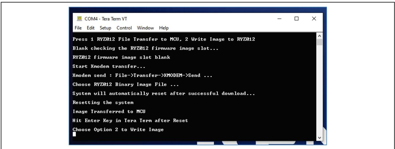
Figure 17. Tera Term – XMODEM Image Transferred to MCU
