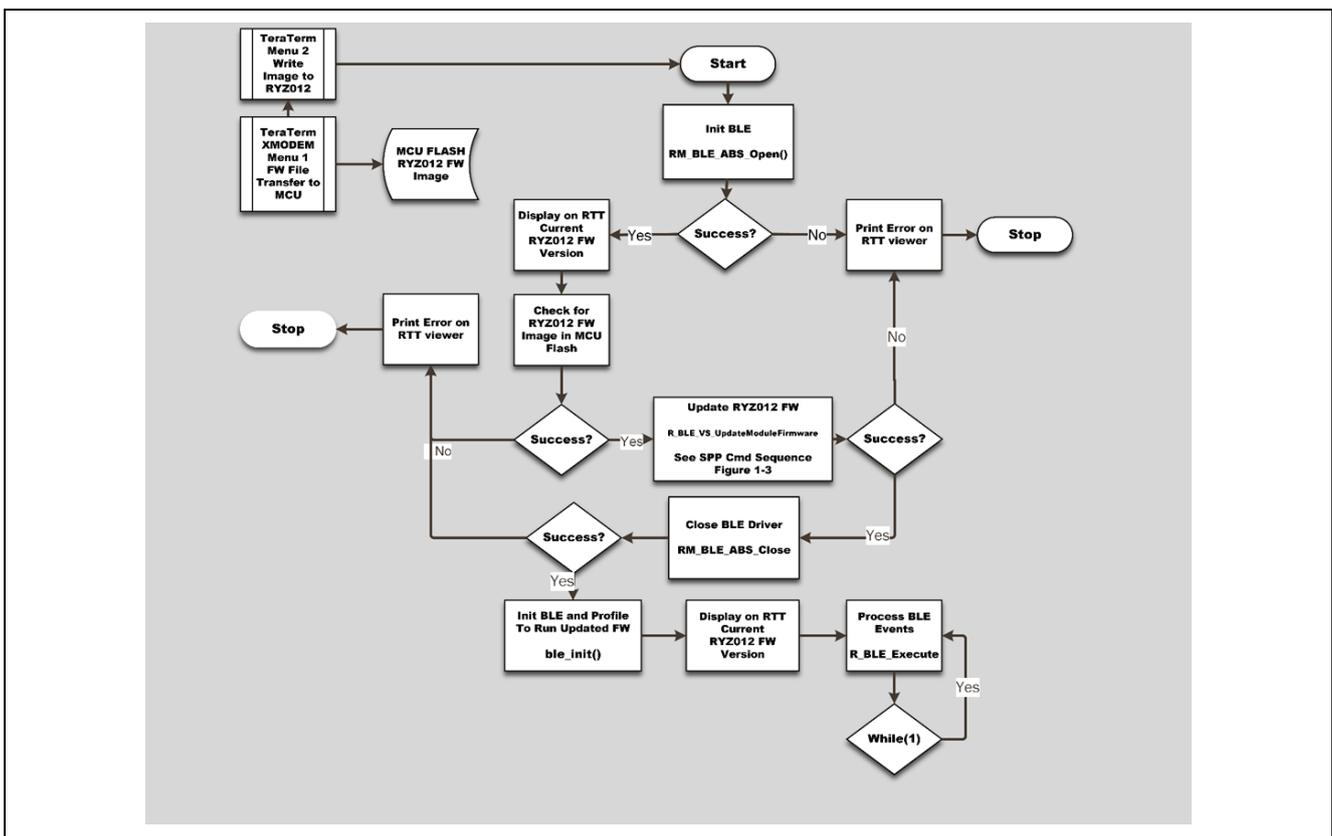
Figure 2. MCU User Application Flow Diagram
