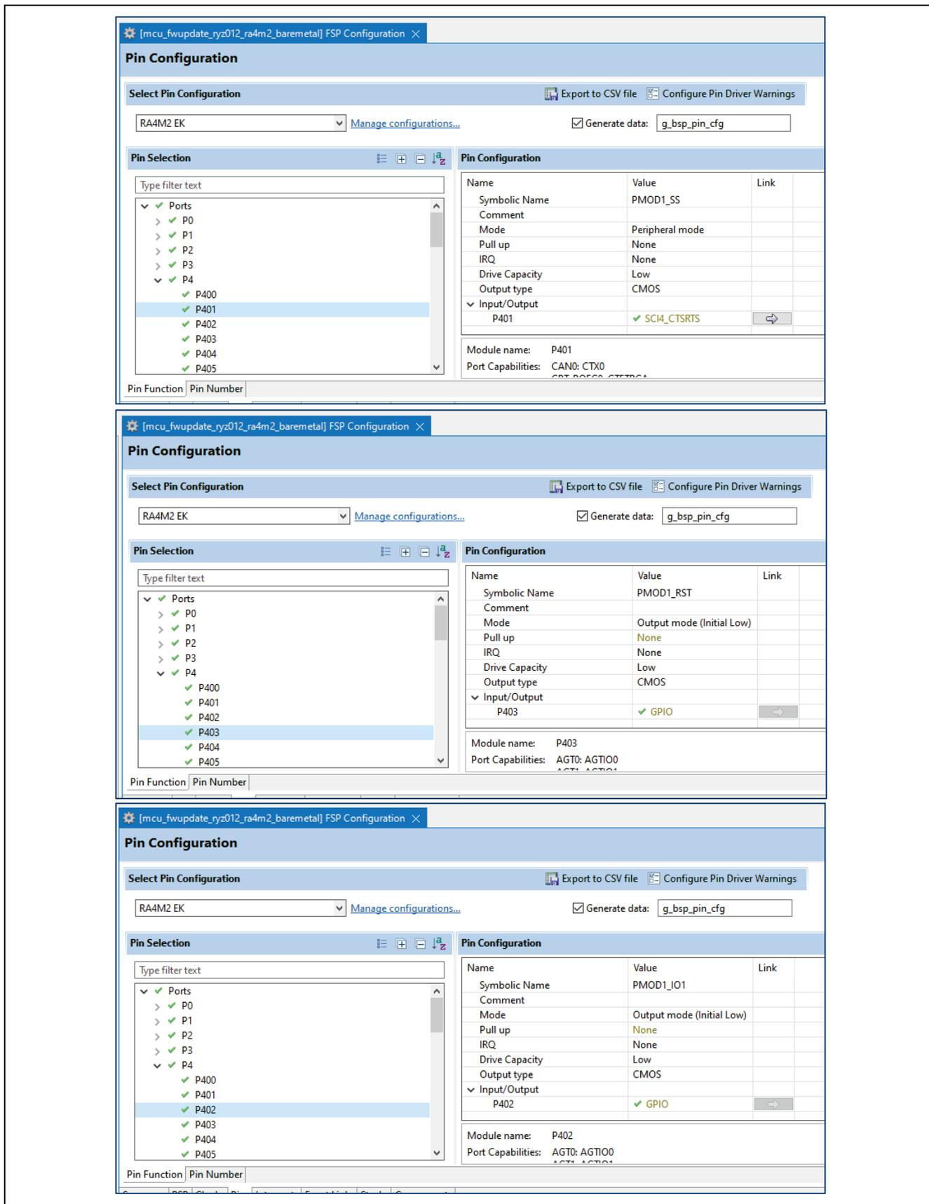
Figure 35. Pin Configuration > Ports
