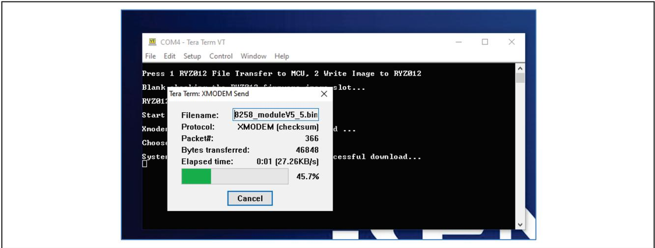
Figure 15. Tera Term – XMODEM File Send in Progress
