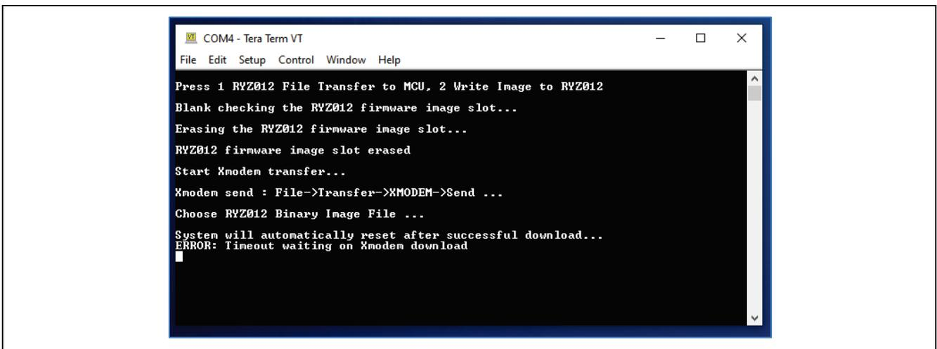
Figure 16. Tera Term – XMODEM Timeout Waiting on File
