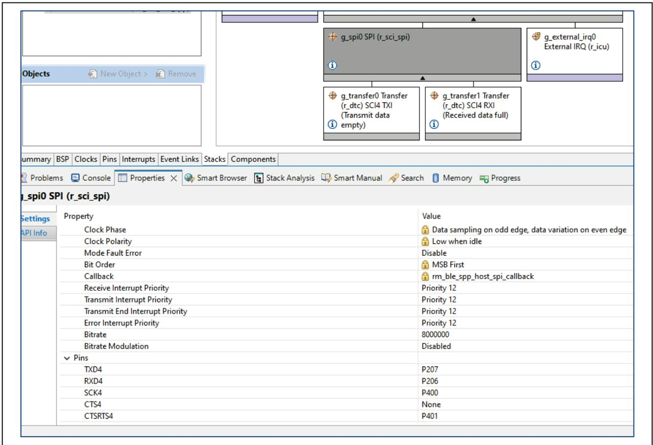
Figure 33. SPI Module Properties – Pin Assignments
