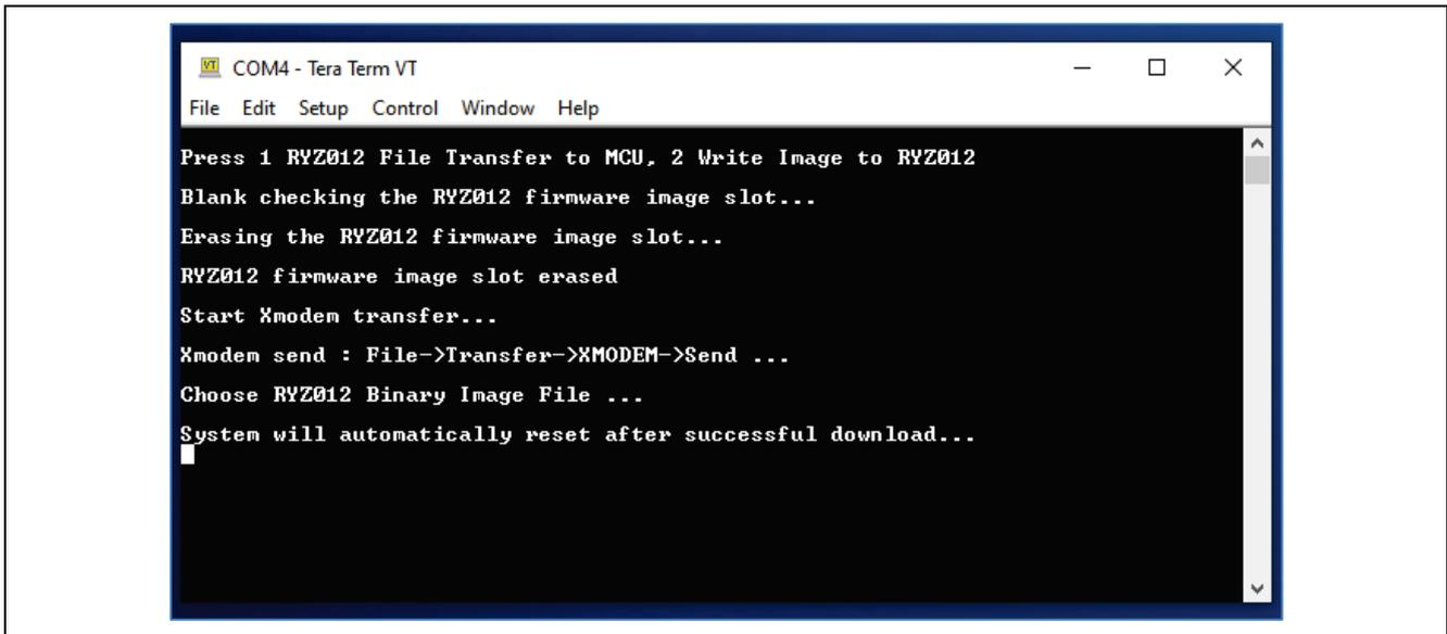
Figure 13. Tera Term – Press 1 File Transfer to MCU
