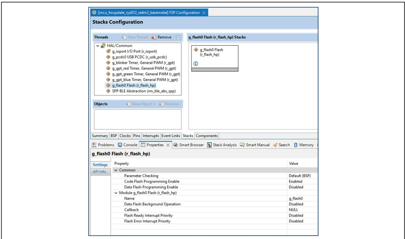
Figure 37. Stack Configuration > g\_flash0 Flash (r\_flash\_hp)
