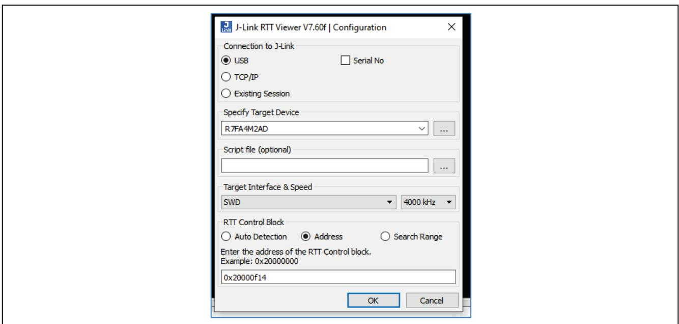
**Figure 8. J-Link RTT Viewer Configuration**
