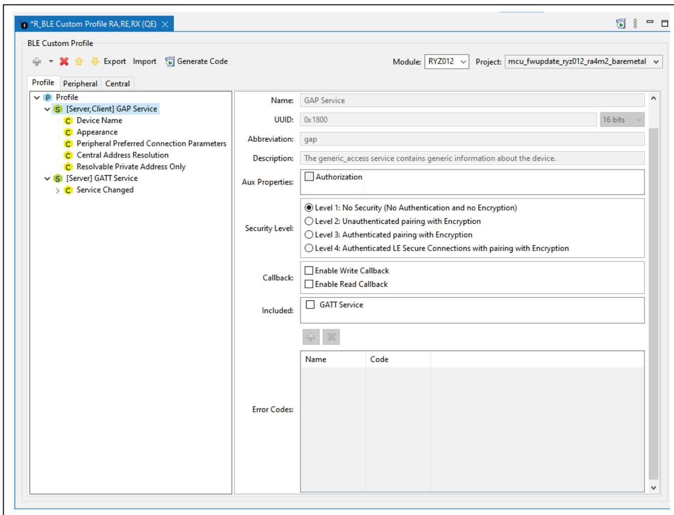
**Figure 39. Creating BLE Profile with QE for BLE**
