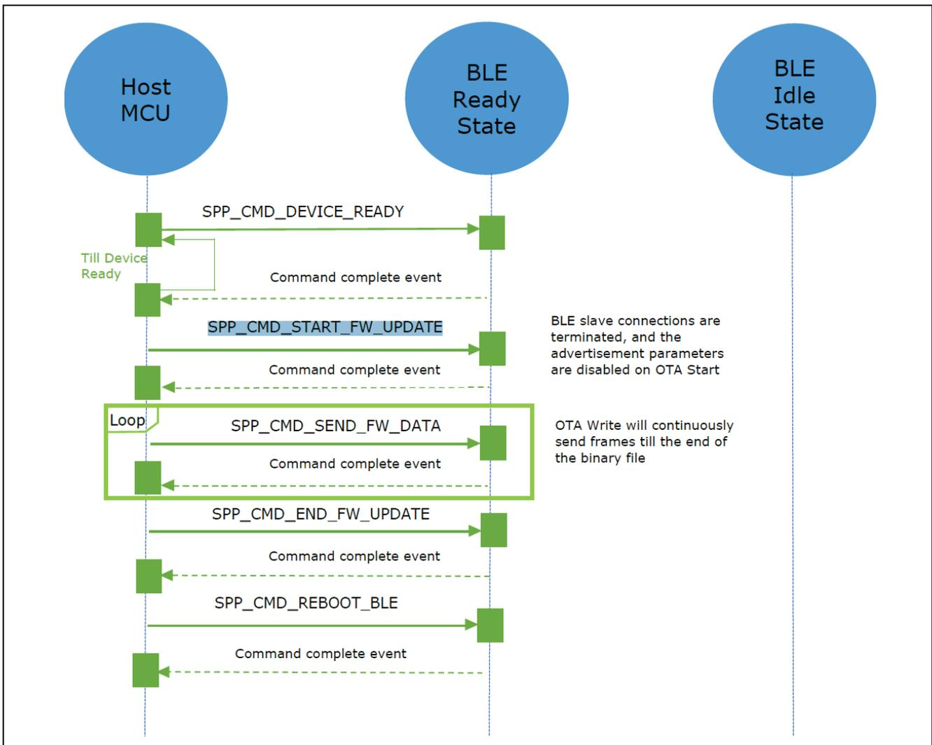
**Figure 3. SPP Command Sequence for RYZ012 Firmware Update**
