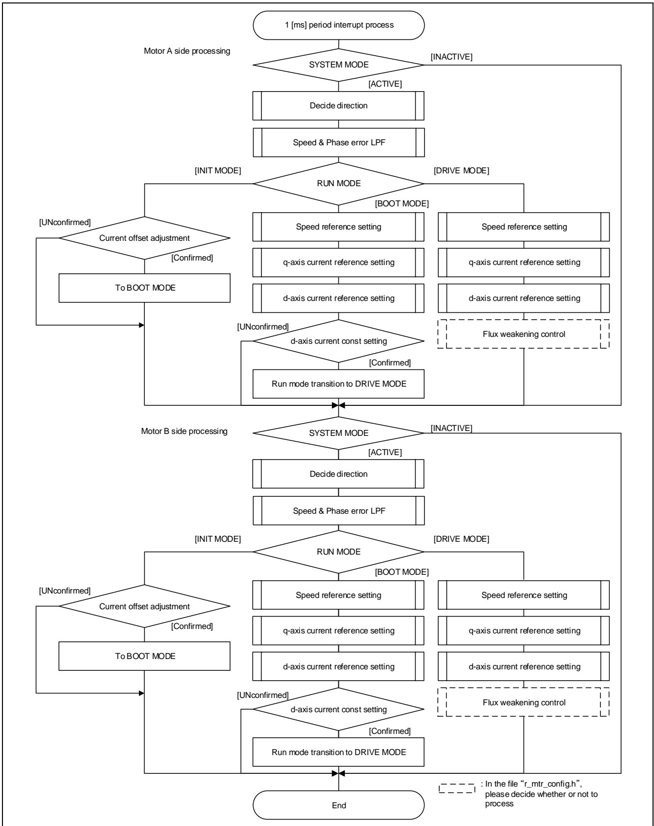
Figure 3-11 1[ms] Period Interrupt Process Flowchart
