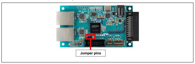
Figure 2.2 Setting up Jumper Pins
