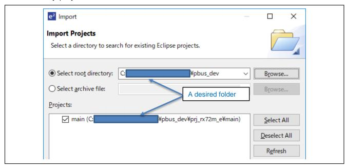
Check "main (C:<desired folder>\text{\*pbus\_dev\*prj\_rx72m\_e\*main})" under the [Projects] label and select [Next]. The project will be imported into the workspace.
