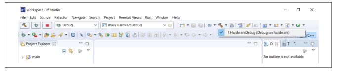
(2) e<sup>2</sup> studio will build the project. After the build is completed, select the arrow next to the debug button (bug icon). You can start debugging by selecting [Debug Configurations...].
