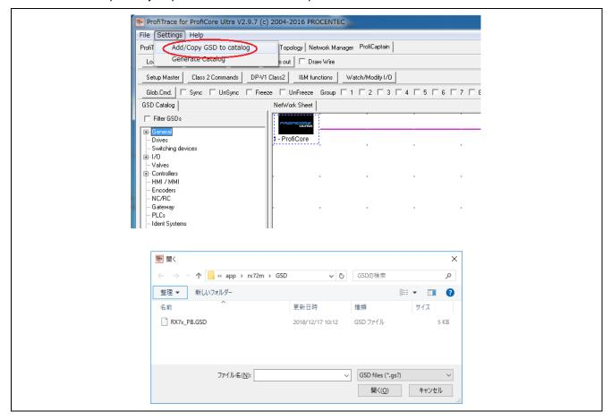
(5) Select [DP Slave] from the items under "I/O" in the [GSD Catalog] view and drag-and-drop it onto the location shown below to register the slave.
