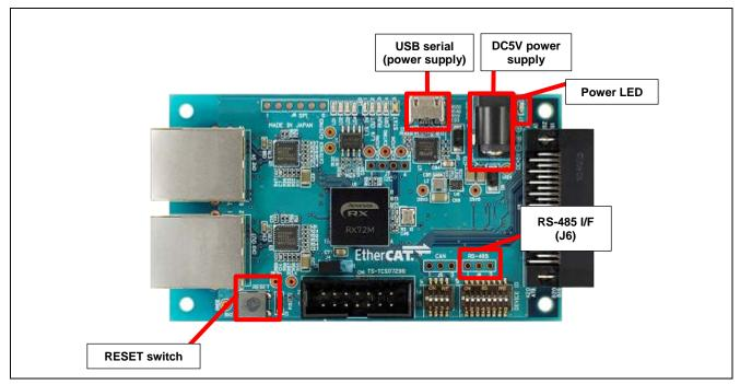
Figure 2.1 Configuration of the RX72M Communications Board
