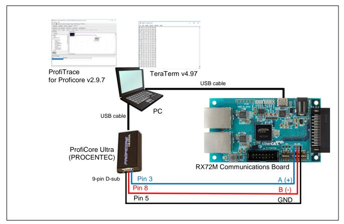
Figure 7.1 Configuration of Connections
