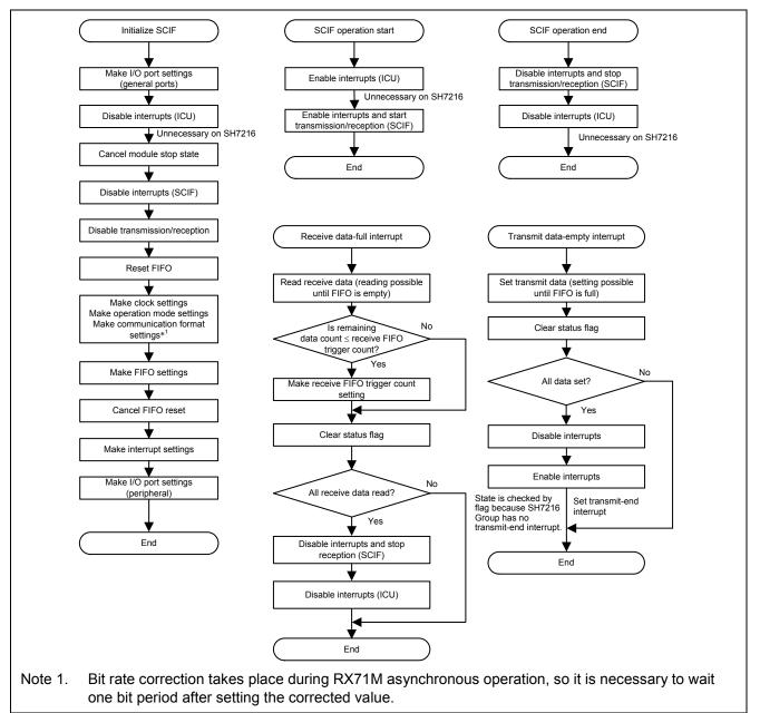
Figure 2.32 Example Flowcharts of SCIF Processing
