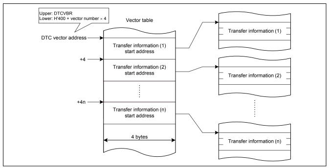
Figure 2.11 DTC Vector Configuration on SH7216 Group
