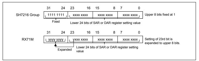
Figure 2.13 Transfer Source and Transfer Destination Addresses in Short Address Mode
