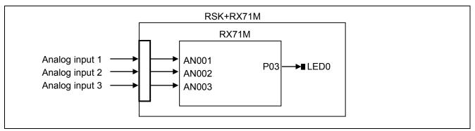
Figure 2.48 Operation Specifications for A/D Conversion in Continuous Scan Mode
