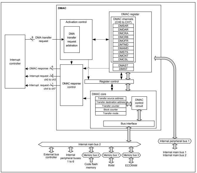
Figure 2.18 RX71M DMACAa Block Diagram
