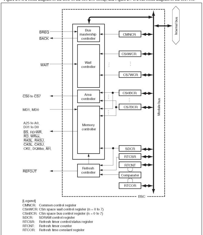
Figure 2.6 SH7216 Group Bus Block Diagram
