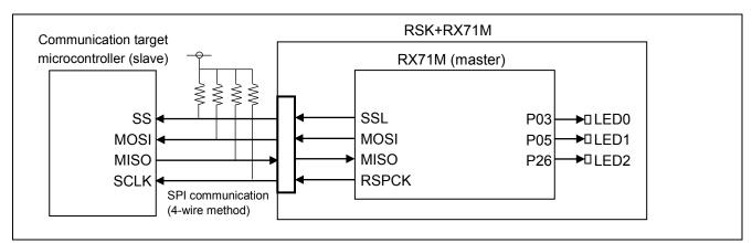
Figure 2.35 SPI Master Transmission and Reception Connection Example
