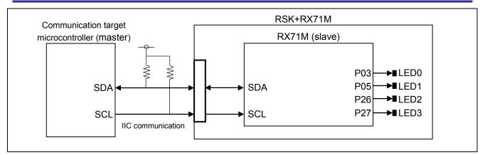
Figure 2.45 IIC Slave Transmission and Reception Connection Example
