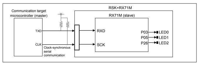
Figure 2.34 Clock-Synchronous Slave Receive Connection Example
