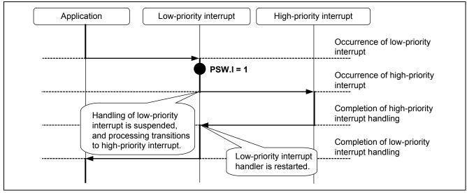
Figure 1.26 RX71M Interrupt Sequence (Controlled by PSW.I Bit)
