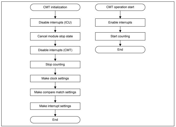
Figure 2.56 Example Flowcharts of CMT Processing
