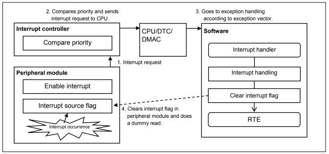
Figure 1.20 SH7216 Group Peripheral Module Interrupt (Edge Detection)
