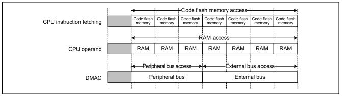
Figure 2.20 RX71M Parallel Bus Operation
