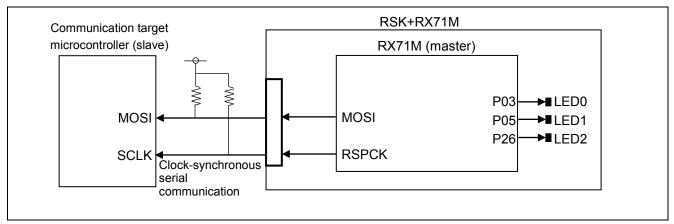
Figure 2.37 Clock-Synchronous Master Transmission Connection Example
