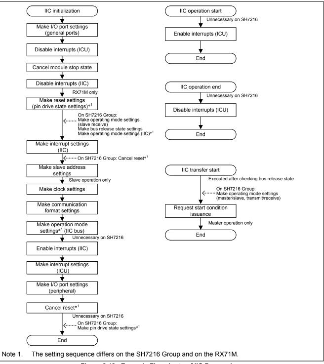
Figure 2.42 Example Flowcharts of IIC Processing
