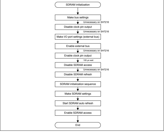
Figure 2.9 External Bus (SDRAM) Processing Flowchart
