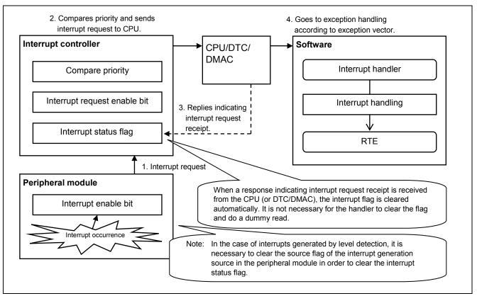
Figure 1.21 RX71M Peripheral Module Interrupt (Edge Detection)
