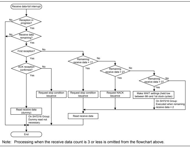
Figure 2.44 Example Flowchart of IIC Receive Data-Full Interrupt Handling (Master Operation)
