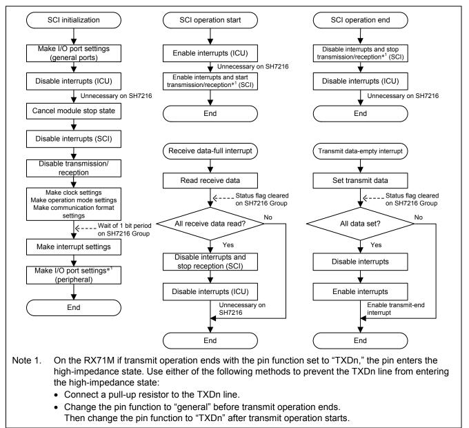
Figure 2.27 Example Flowcharts of SCI Processing
