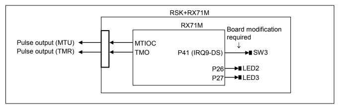
Figure 2.58 Low-Power-Consumption Mode Transition Connection Example
