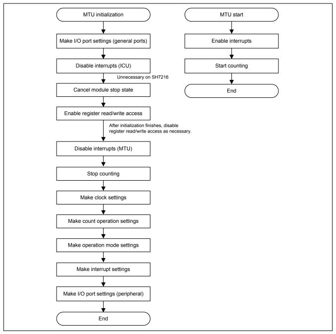
Figure 2.24 Example Flowcharts of MTU Processing
