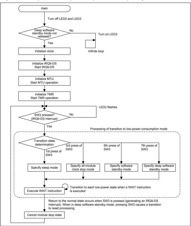
Figure 2.59 Example Flowchart of Low-Power-Consumption Mode Transition Processing
