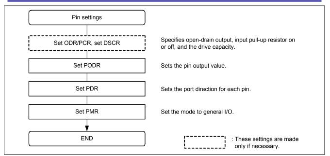
Figure 2.3 RX71M Pin General I/O Setting Flowchart
