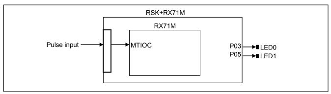
Figure 2.25 Input Capture Pulse Width Measurement Connection Example
