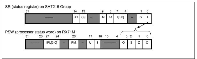
Figure 1.3 Differences Between SR (SH7216 Group) and PSW (RX71M)
