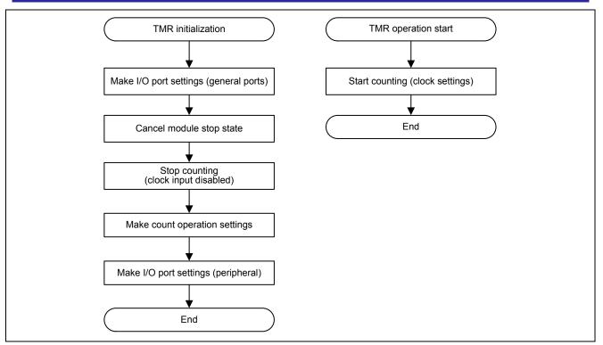
Figure 2.60 Example Flowcharts of TMR Processing
