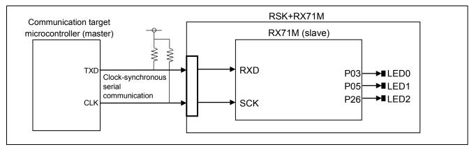
Figure 2.30 Clock-Synchronous Slave Receive Connection Example
