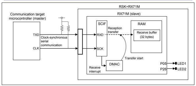
Figure 2.21 Connection Example for Data Transfer between SCIF and On-Chip RAM
