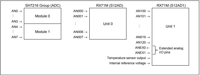
Figure 2.47 Comparison of A/D Converter Configurations
