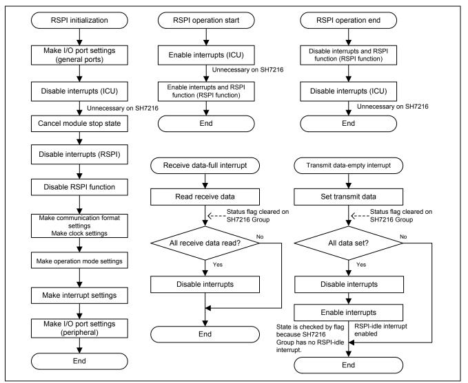
Figure 2.36 Example Flowcharts of RSPI Processing
