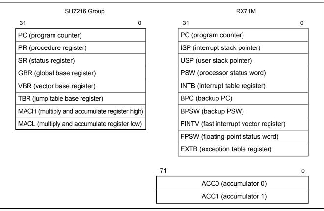
Figure 1.2 Points of Difference Between CPU Registers (Excluding General-Purpose Registers)
