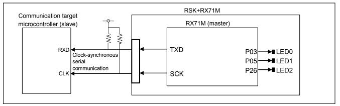
Figure 2.29 Clock-Synchronous Master Transmit Connection Example
