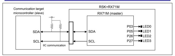
Figure 2.41 IIC Master Transmission and Reception Connection Example
