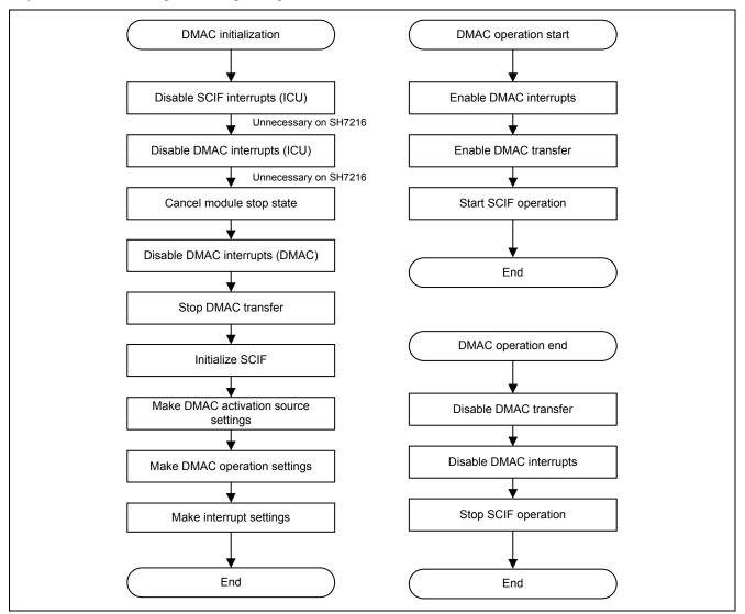
Figure 2.22 Example Flowcharts of DMAC Processing
