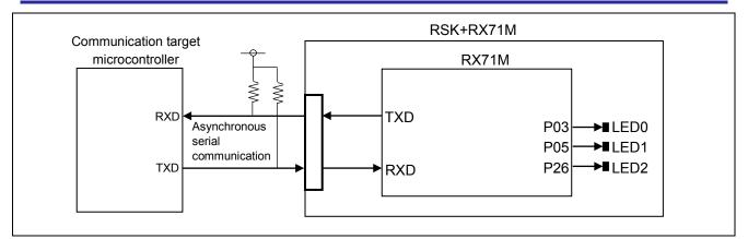
Figure 2.26 Asynchronous Transmit/Receive Connection Example
