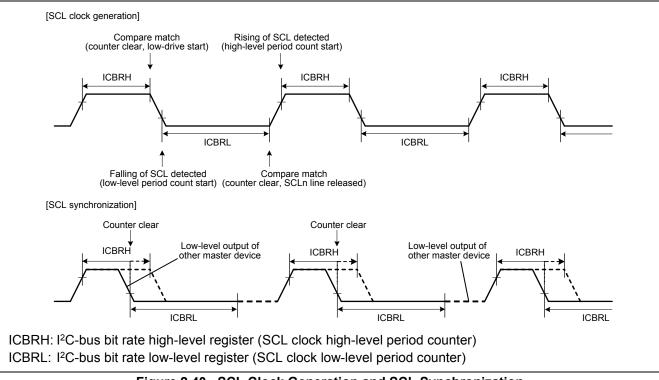
Figure 2.40 illustrates SCL clock generation and SCL synchronization on the RX71M.
