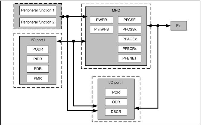
Figure 2.2 I/O Settings on the RX71M
