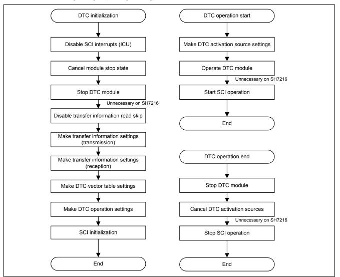
Figure 2.16 Example Flowcharts of DTC Processing
