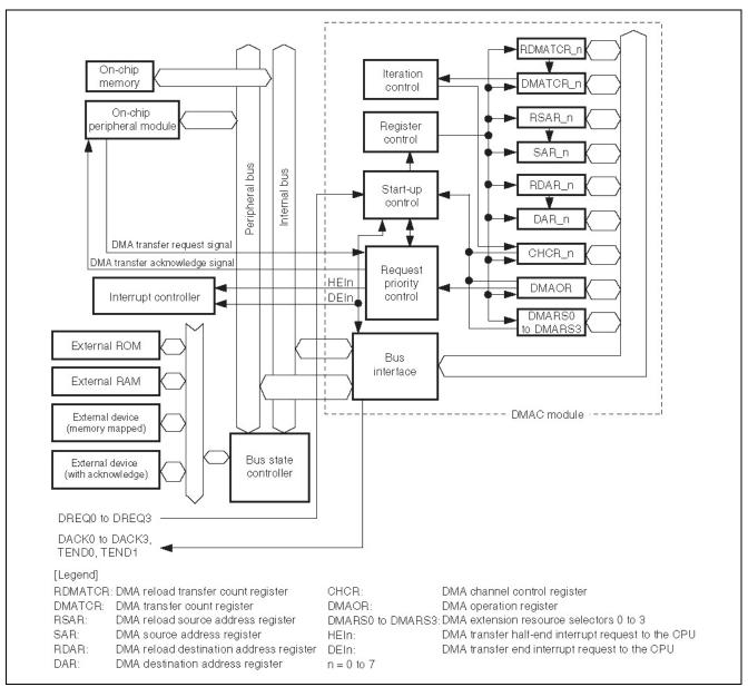
Figure 2.17 SH7216 Group DMAC Block Diagram
