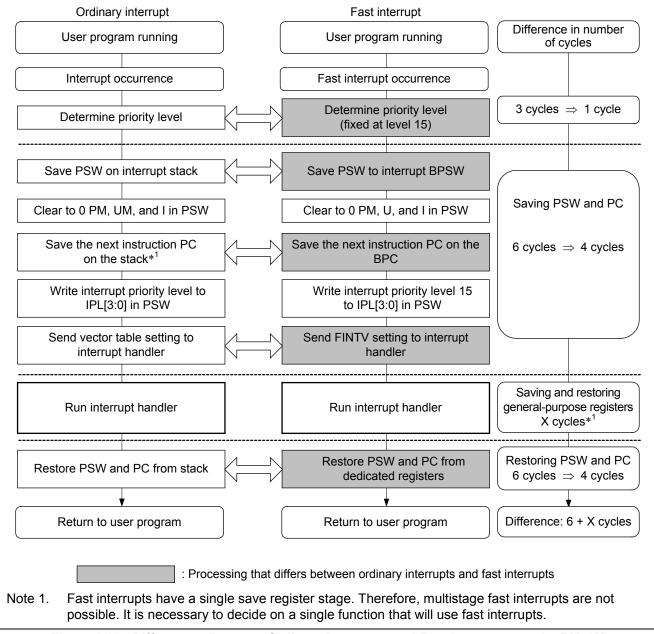
Figure 1.22 Differences Between Ordinary Interrupts and Fast Interrupts on the RX71M
