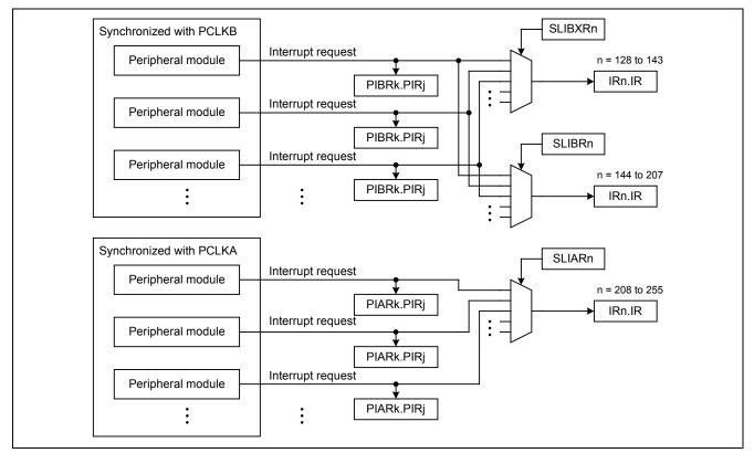
Figure 1.28 Software Configurable Interrupt Configuration on the RX71M
