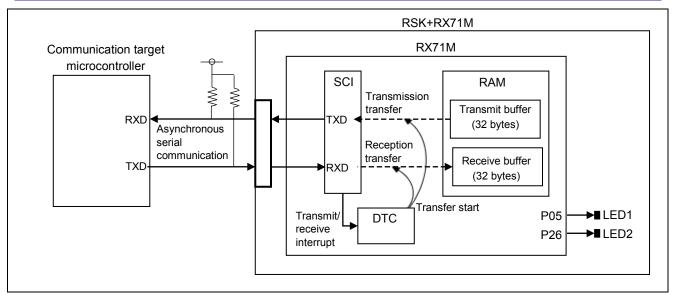
Figure 2.15 Connection Example for Data Transfer between SCI and On-Chip RAM
