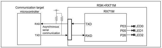
Figure 2.31 Asynchronous Transmit/Receive Connection Example
