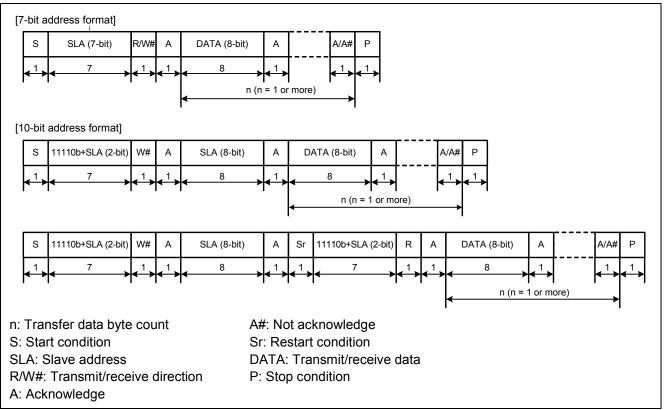
Figure 2.39 RX71M I<sup>2</sup>C Bus Format
