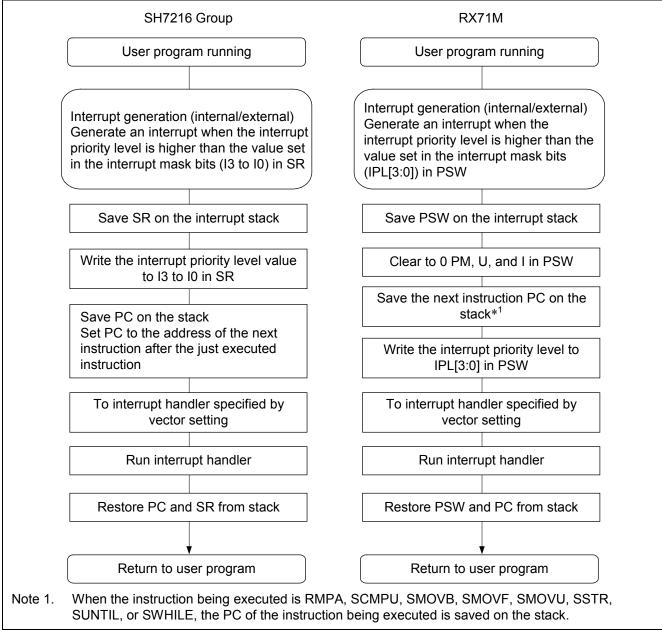
Figure 1.17 Interrupt (Internal/External) Processing Sequence
