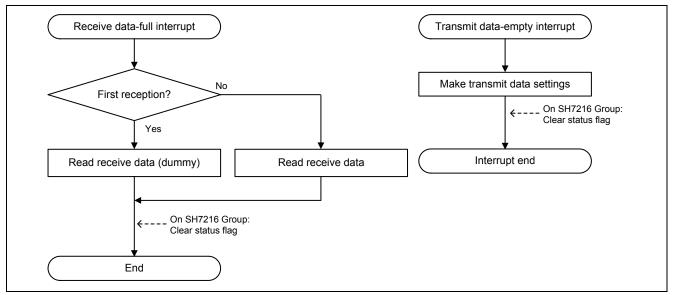
Figure 2.46 Example Flowcharts of IIC interrupt Handling (Slave Operation)
