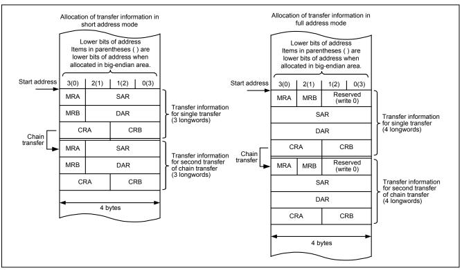
Figure 2.14 shows the allocation of DTC transfer information on the SH7216 Group and RX71M.
