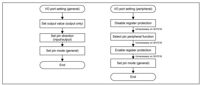
Figure 2.5 Example Flowcharts of I/O Port Setting
