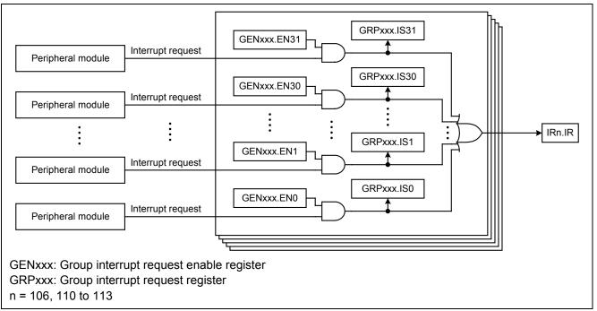
Figure 1.27 Group Interrupt Configuration on the RX71M
