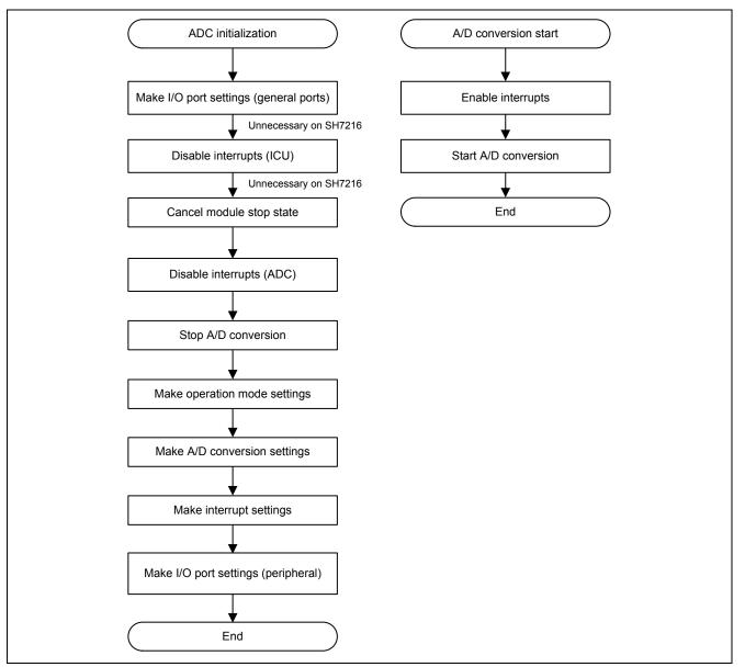
Figure 2.49 Example Flowcharts of ADC Processing
