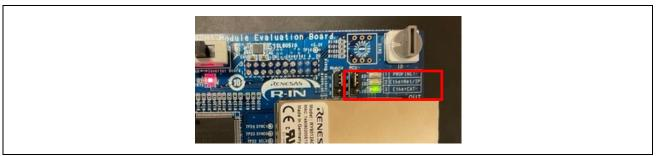
Figure 3-56 Protocol LED: EtherCAT
