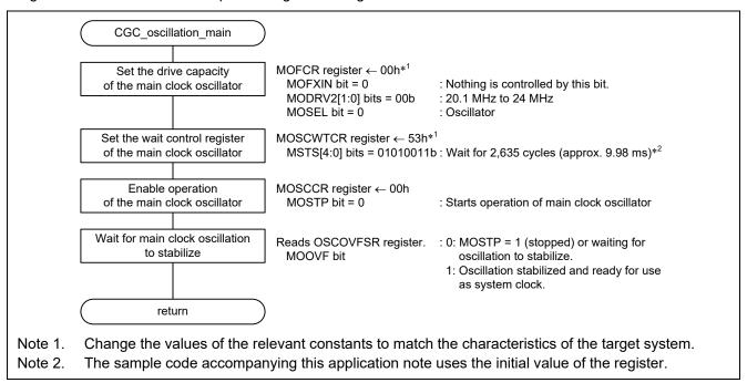
Figure 3.6 Main Clock Oscillation Enable
