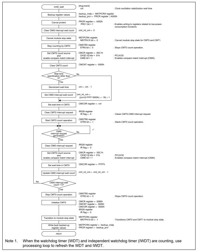
Figure 3.12 Software Wait Cycles Using CMT0
