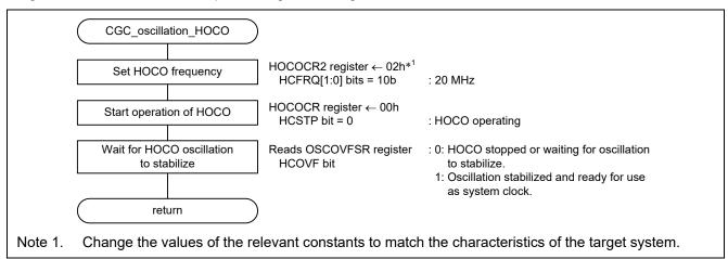
Figure 3.8 HOCO Clock Oscillation Enable
