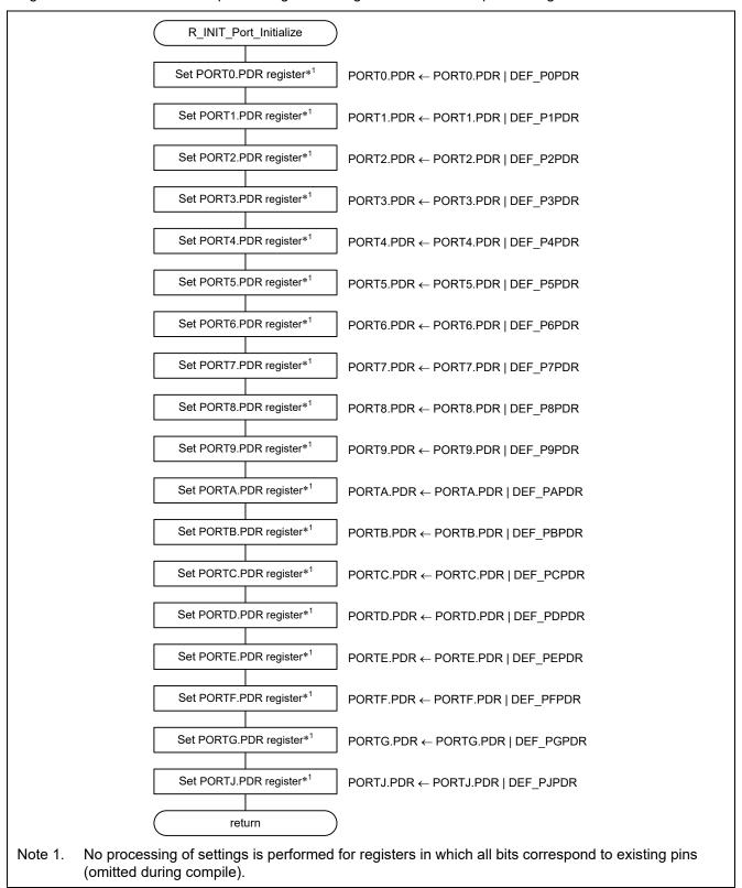
Figure 3.3 Initial Nonexistent Port Settings
