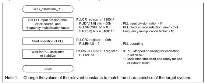
Figure 3.7 PLL Clock Oscillation Enable
