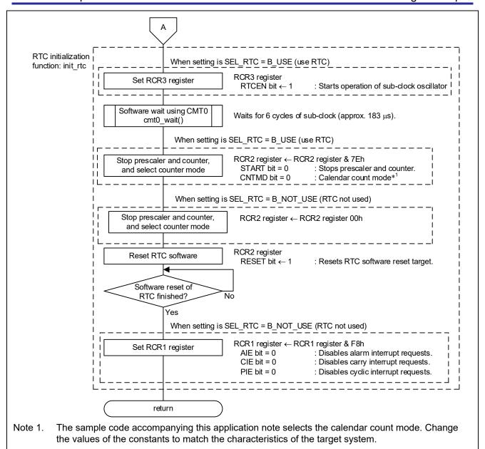
Figure 3.10 Sub-clock Oscillation Enable (2/2)
