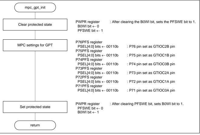
Figure 4.9 MPC Initial Settings Function for GPT
