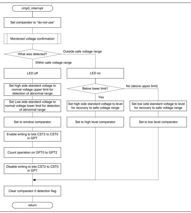
Figure 4.14 Comparator Interrupt Function
