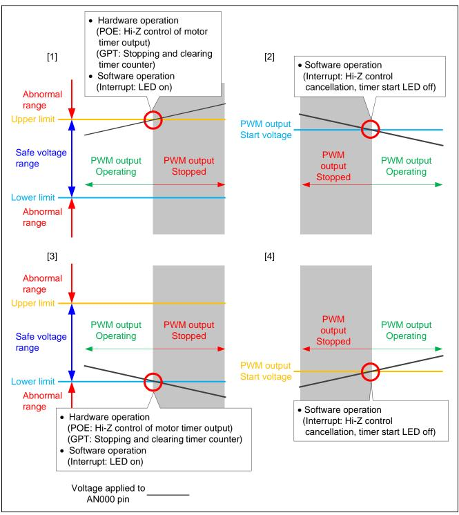
Figure 4.1 Operation Example of POE PWM Output Cutoff by Comparator Detection
