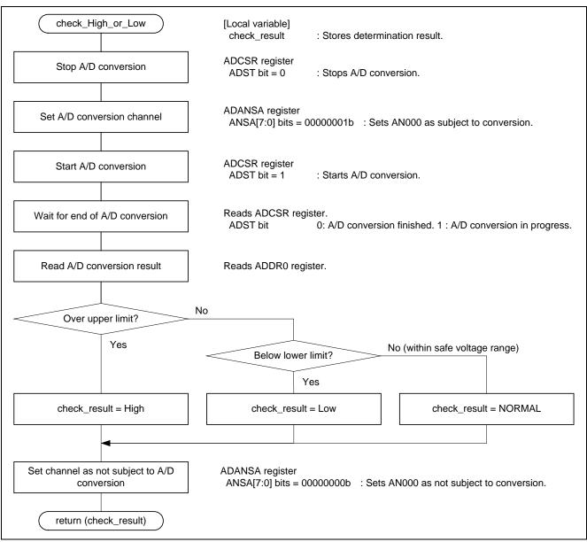
Figure 4.13 Monitored Voltage Confirmation Function
