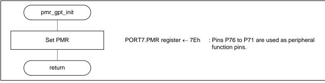
Figure 4.12 PMR Initial Settings Function for GPT
