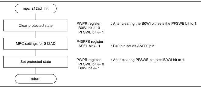
Figure 4.10 MPC Initial Settings Function for S12AD
