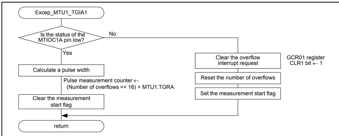
Figure 5.18 MTU1 Input Capture A Interrupt Handler
