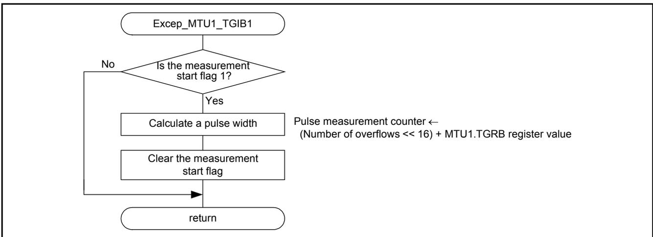
Figure 5.9 MTU1 Input Capture B Interrupt Handler
