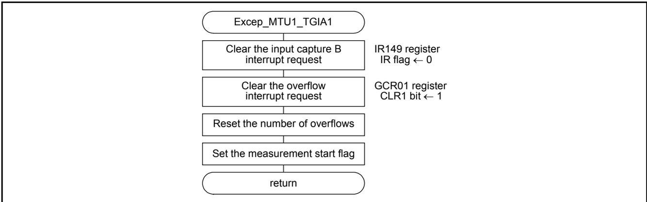
Figure 5.8 MTU1 Input Capture A Interrupt Handler
