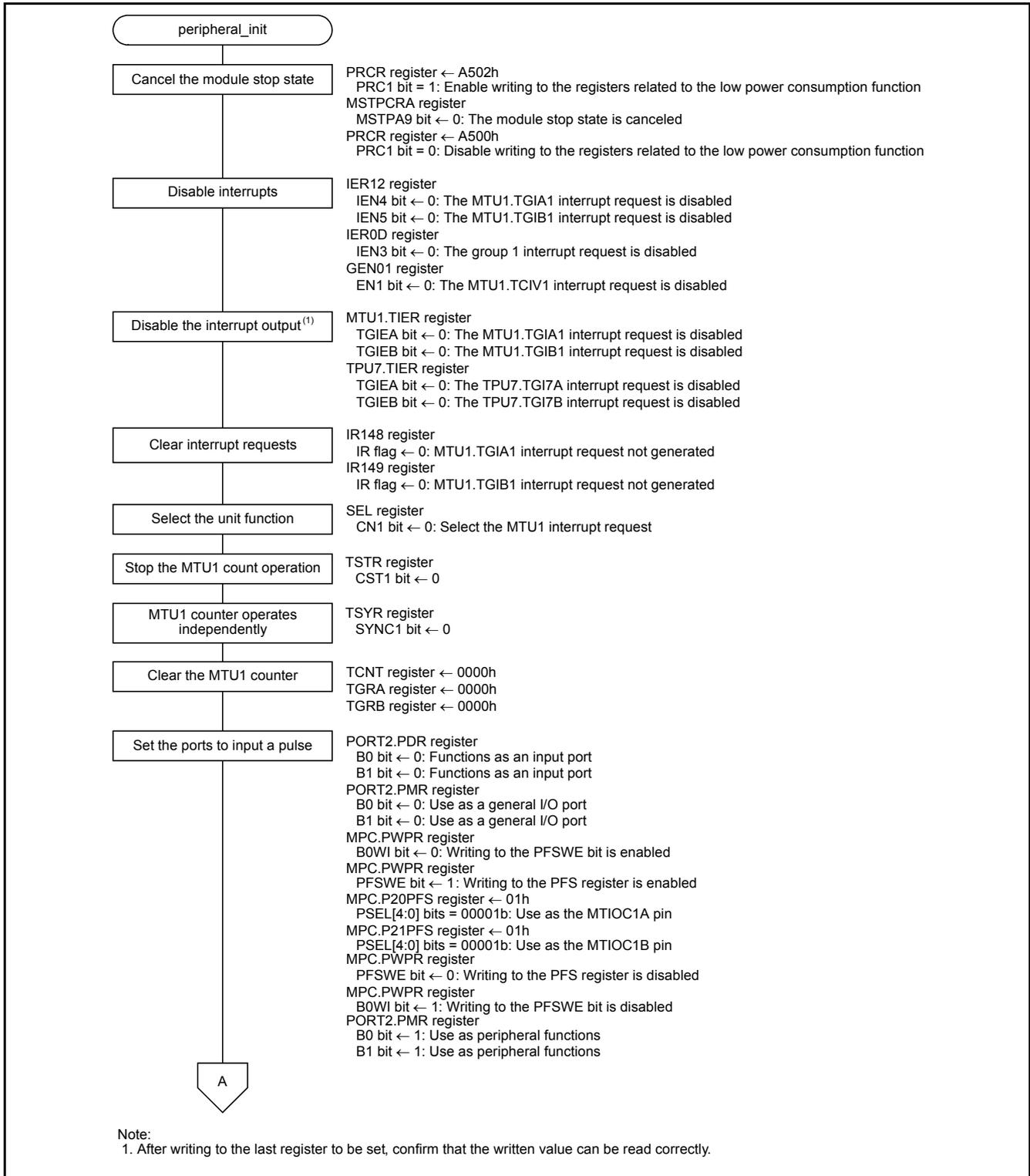
Figure 5.5 Peripheral Function Initialization (1/2)
