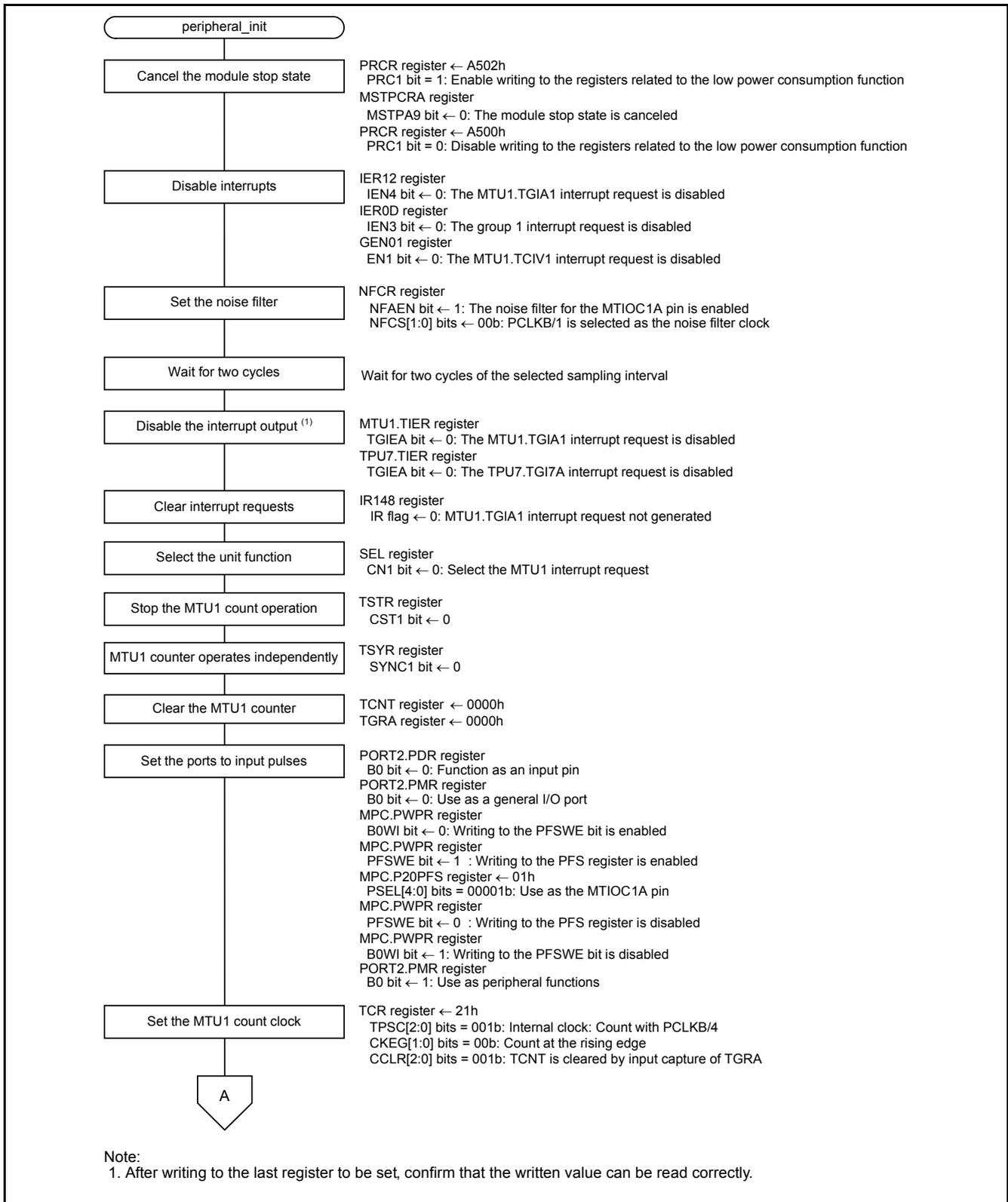
Figure 5.15 Peripheral Function Initialization (1/2)
