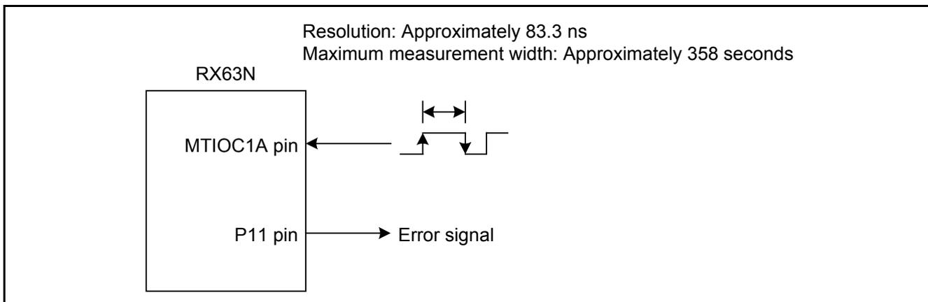
**Figure 1.2 Connection Diagram of Sample Code 2**
