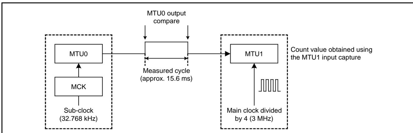
**Figure 1.1 Block Diagram**
