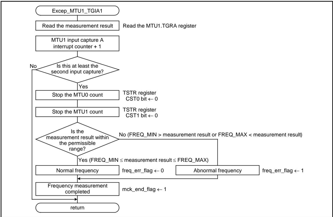
Figure 4.5 MTU1 Input Capture A Interrupt Handling
