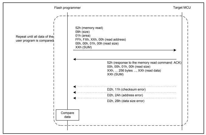
Figure 5.13 Procedure to Confirm Data in the User Area
