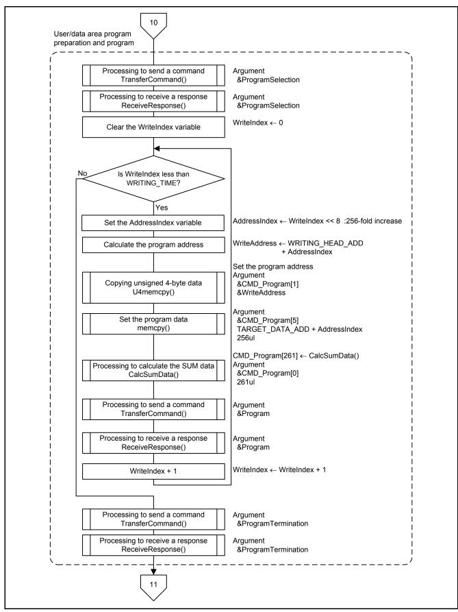
Figure 5.26 Main Processing and Communication Protocol Control (11/13)
