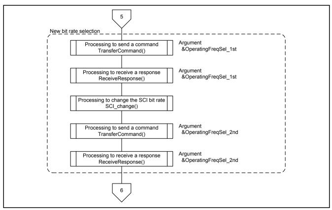
Figure 5.21 Main Processing and Communication Protocol Control (6/13)
