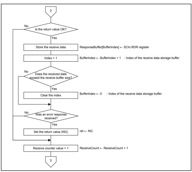
Figure 5.42 Processing to Receive a Response
