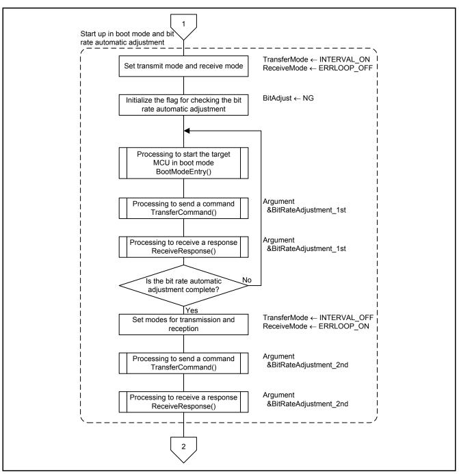
Figure 5.17 Main Processing and Communication Protocol Control (2/13)
