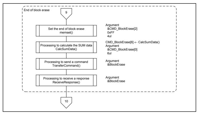
Figure 5.25 Main Processing and Communication Protocol Control (10/13)
