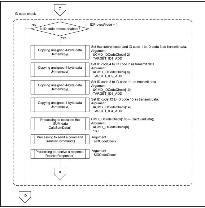
Figure 5.23 Main Processing and Communication Protocol Control (8/13)
