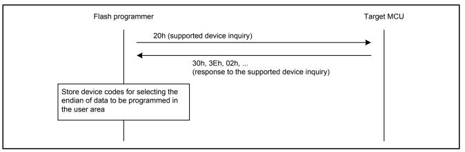
Figure 5.5 Procedure to Store Device Codes
