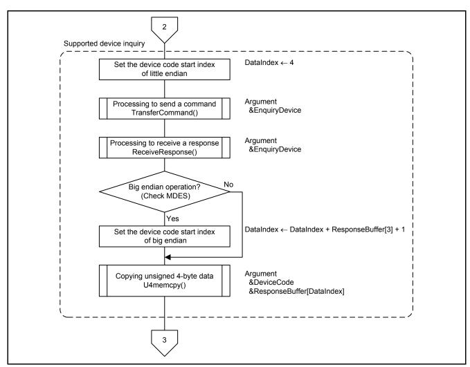
Figure 5.18 Main Processing and Communication Protocol Control (3/13)
