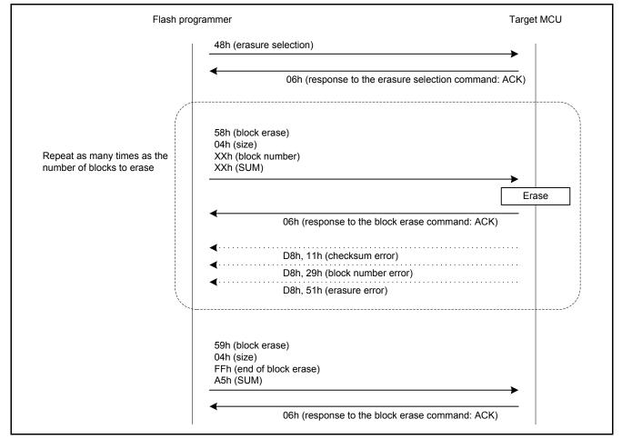
Figure 5.11 shows the Procedure to Erase the Flash Memory of the Target MCU.
