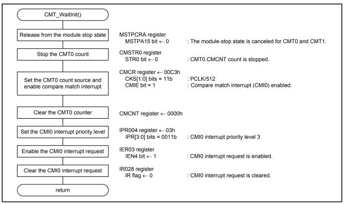
Figure 5.30 Initialization of the Timer for Wait Time with the CMT
