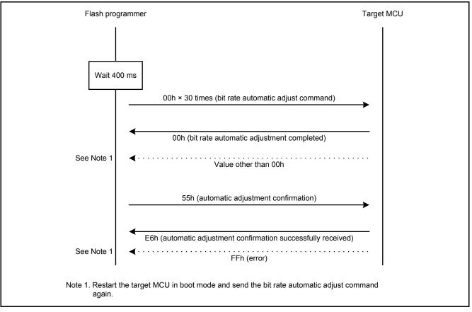
Figure 5.4 Bit Rate Automatic Adjustment Procedure
