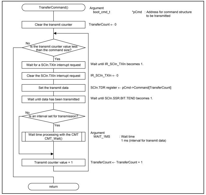
Figure 5.39 Processing to Send a Command
