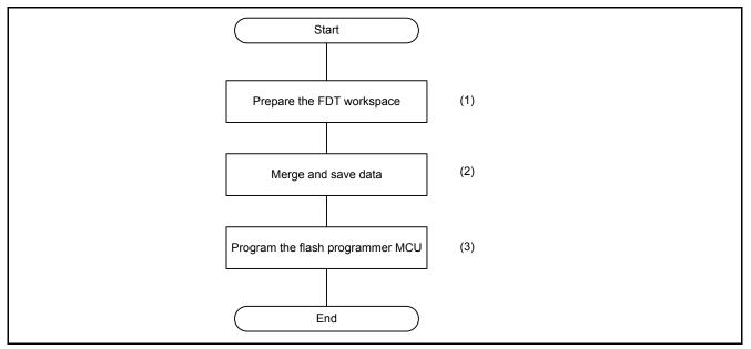
Figure 5.1 Flow of Programming the RSK+RX63N
