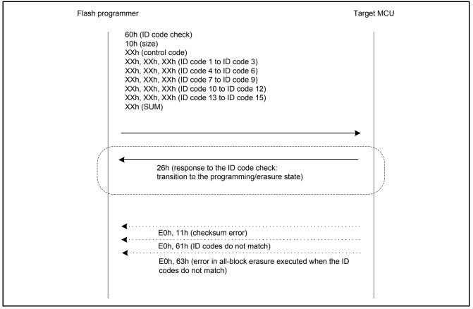
Figure 5.10 Procedure to Check ID Code Protection by the ID Code Check Command
