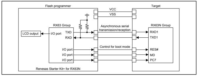
Figure 1.1 Flash Programmer Usage Example
