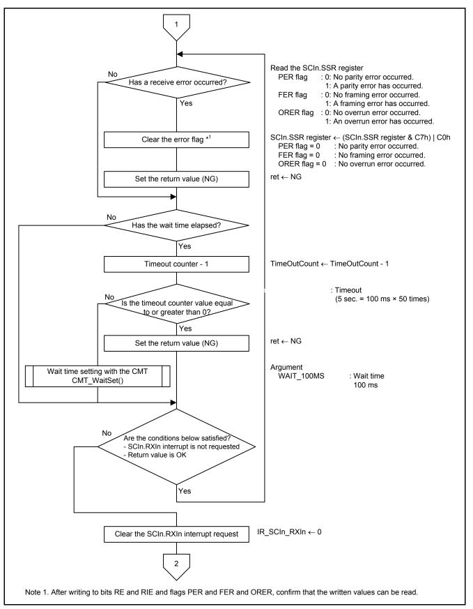
Figure 5.41 Processing to Receive a Response
