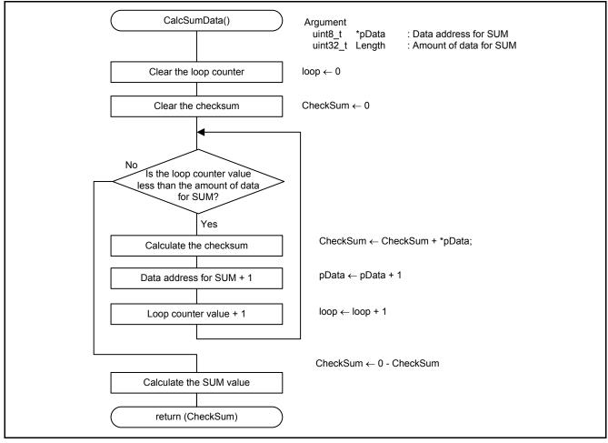
Figure 5.36 Processing to Calculate the SUM Data
