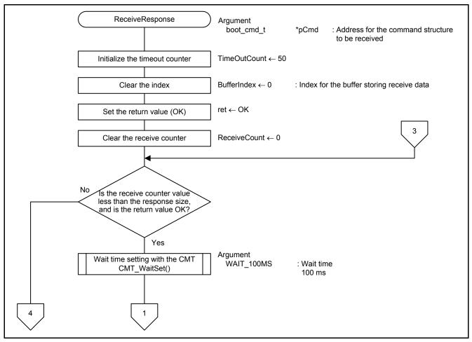
Figure 5.40 Processing to Receive a Response
