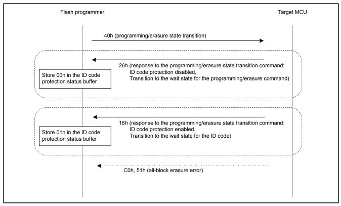
Figure 5.9 Procedure to Check ID Code Protection by the Programming/Erasure State Transition Command
