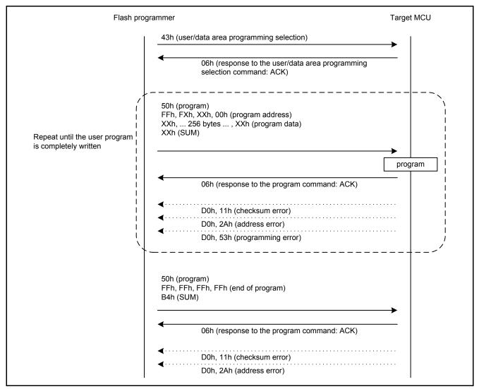
Figure 5.12 Procedure to Program the User Area
