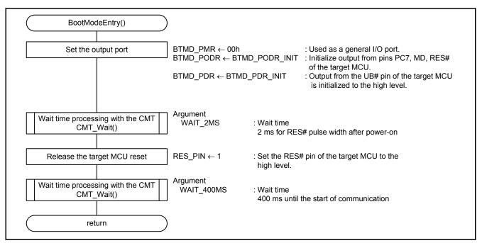
Figure 5.37 Processing to Start the Target MCU in Boot Mode
