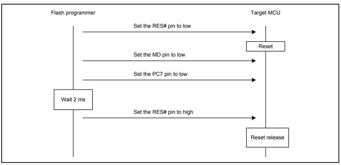
Figure 5.3 Start Procedure in Boot Mode
