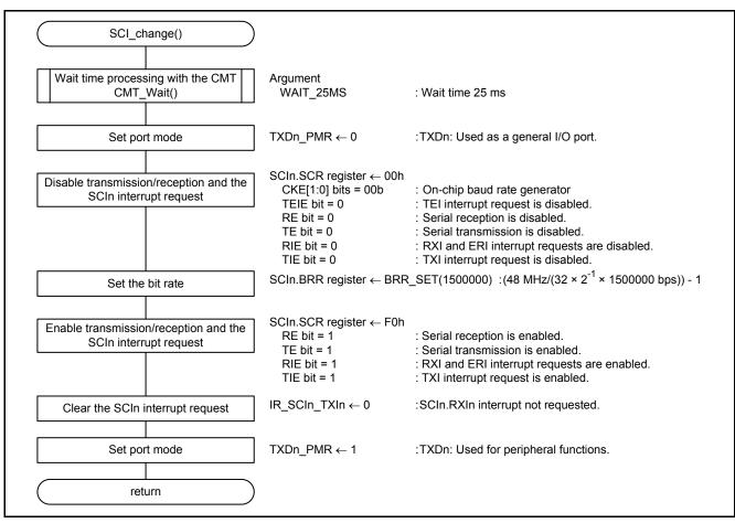
Figure 5.35 Processing to Change the SCI Bit Rate
