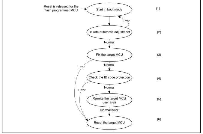
Figure 5.2 Flash Programmer State Transition
