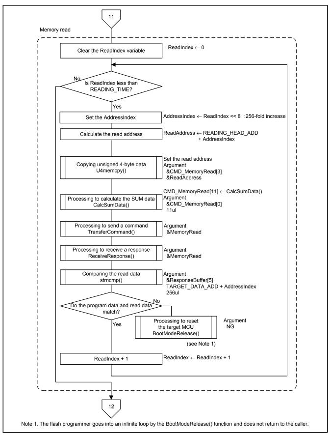
Figure 5.27 Main Processing and Communication Protocol Control (12/13)
