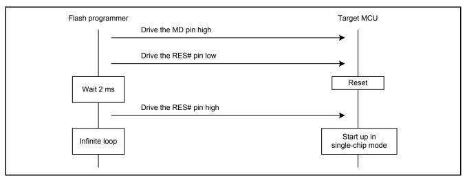
Figure 5.14 Procedure to Reset the Target MCU
