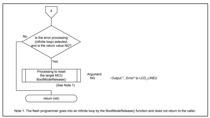
Figure 5.43 Processing to Receive a Response
