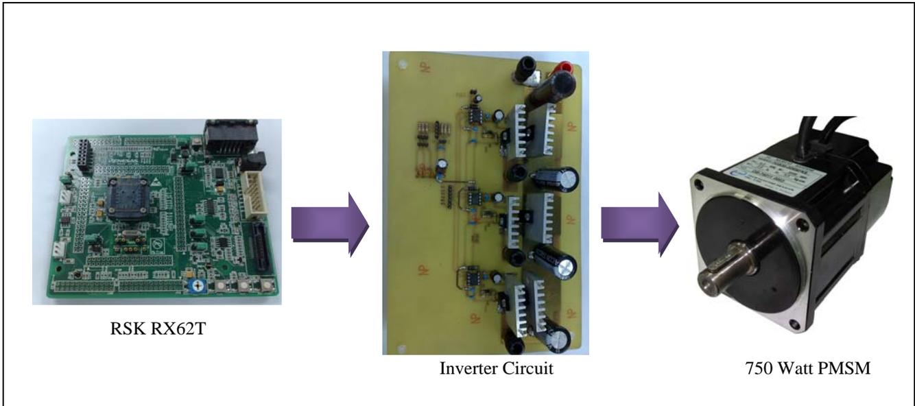
Figure 1-1 System Configuration
