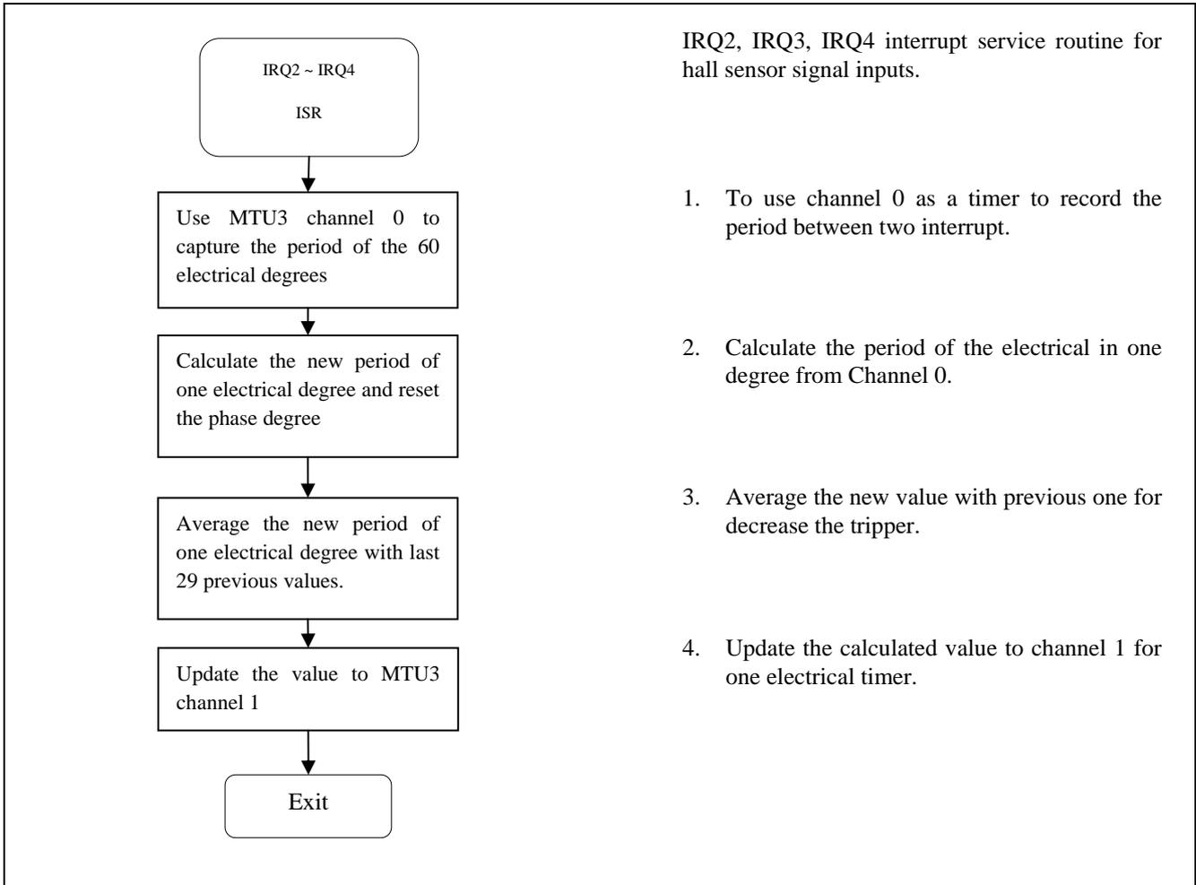
Figure 3-1 ISR of Hall Sensor Signal Input
