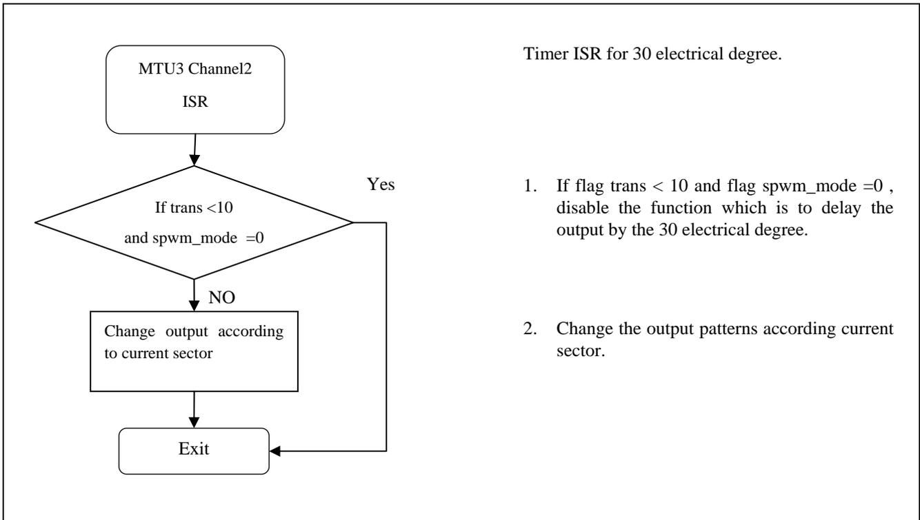
Figure 3-3 ISR for 30 Electrical Degrees in MTU3 Channel 2
