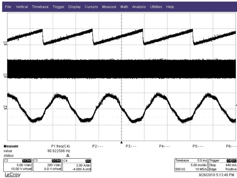
( a )  $V_{DC} = 200 \text{ V}$ ,  $f_{sw} = 20 \text{ kHz}$ ,  $M = 0.4 \text{ p.u.}$  for SPWM
