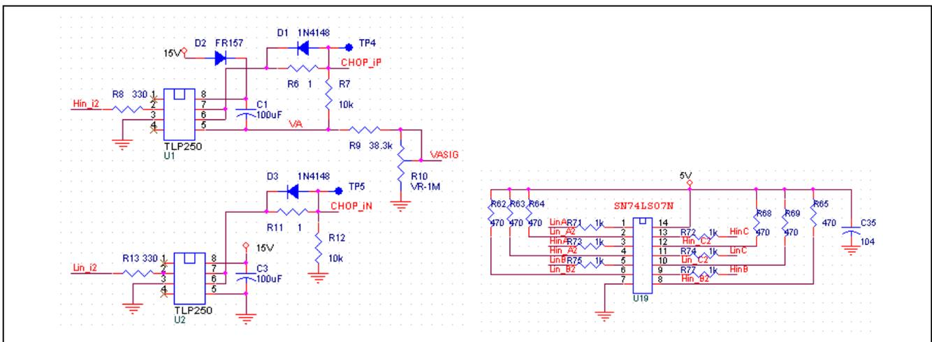
Figure 1-2 Inverter Driver (Left) and buffer stage (Right)
