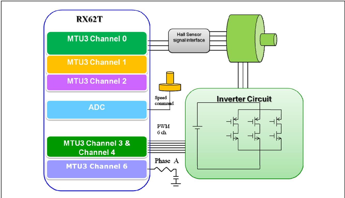
Figure 2-1 Block Diagram
