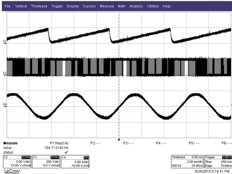
( b )  $V_{DC} = 200 \text{ V}$ ,  $f_{sw} = 20 \text{ kHz}$ ,  $M = 0.9 \text{ p.u.}$  for SPWM
