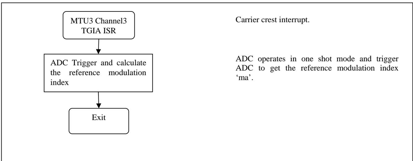
Figure 3-2 Carrier Interrupts (MTU3 channel3 TGIA)
