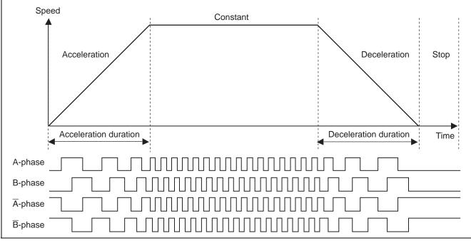
Figure 4.3 Stepping Motor Speed Control
