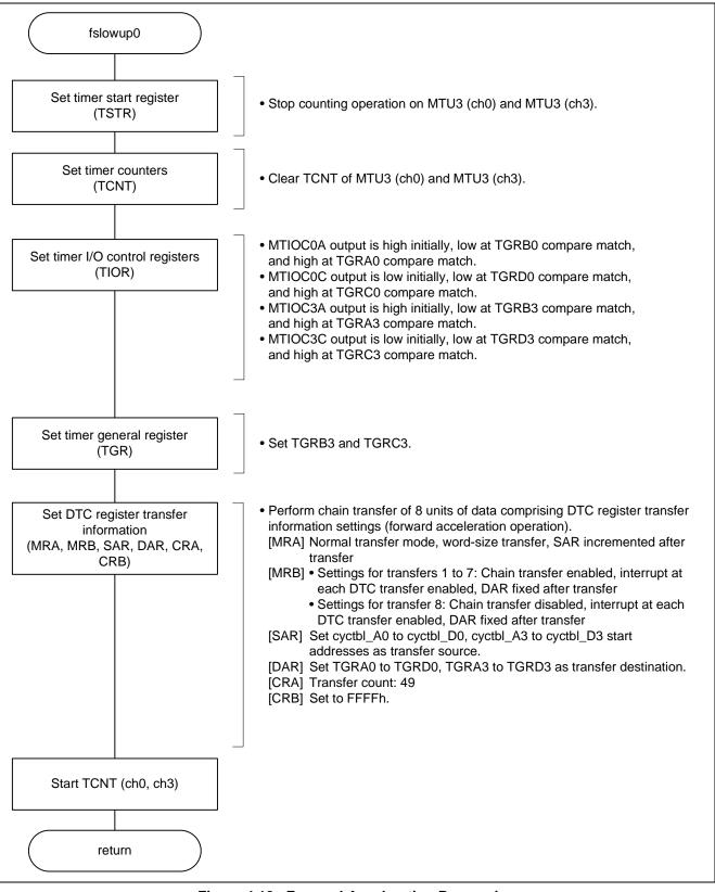
Figure 4.18 Forward Acceleration Processing
