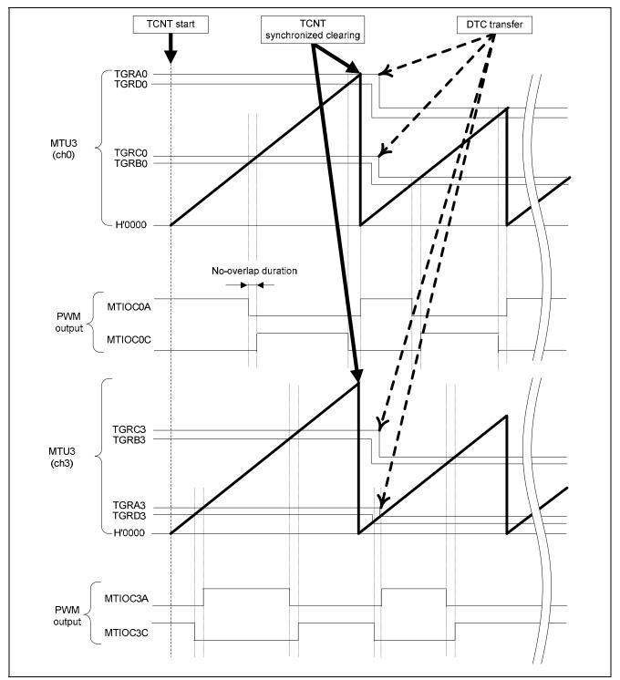
Figure 4.4 shows an example of pulse output during stepping motor acceleration control.
