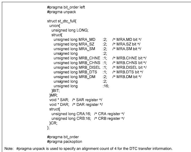
Figure 4.6 Structures and Unions Used in Sample Code (DTC Transfer Information)
