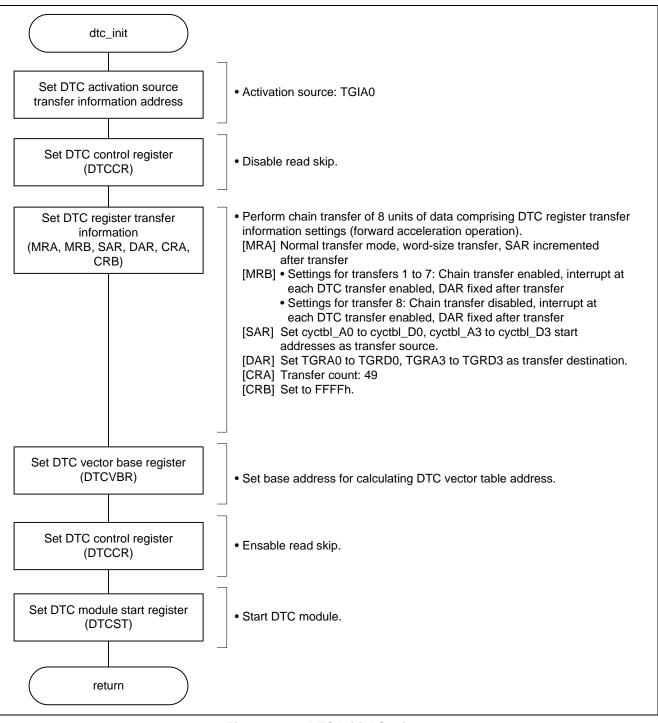
Figure 4.13 DTC Initial Settings
