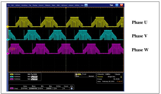
Figure 5-3 Three Phase BEMF Signal
