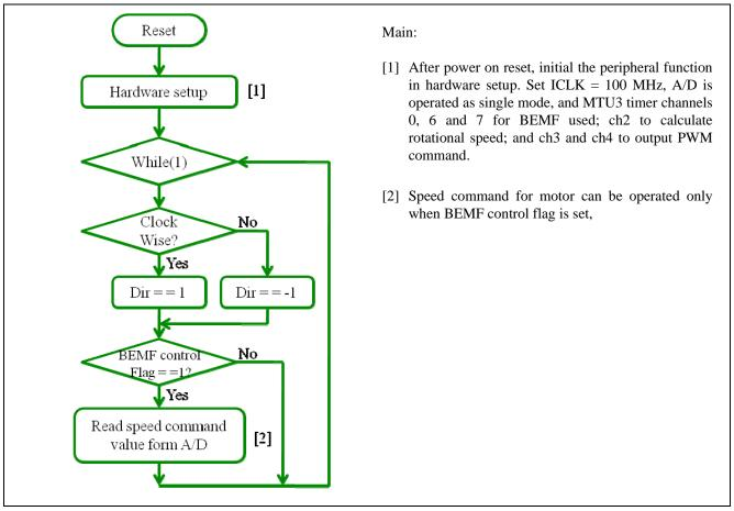
Figure 4-1 Main Function Control Procedure
