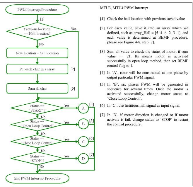
Figure 4-3 PWM Control Procedure
