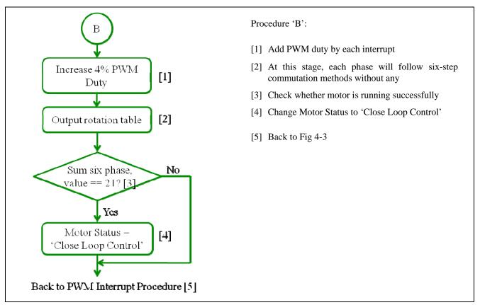
Figure 4-5 Motor Status is 'Open Loop Control' in PWM Control Procedure
