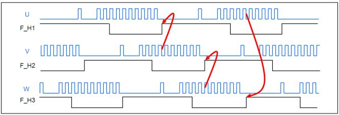
Figure 3-3 Relation between 3 Phase BEMF signal and Fictitious Signal
