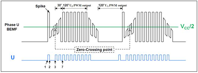
Figure 3-1 Zero-crossing Point Calculation
