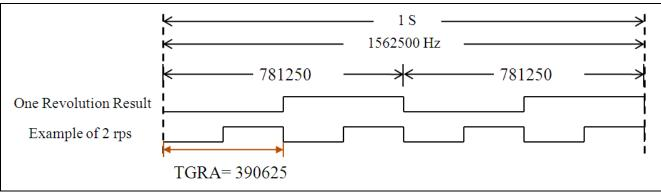
Figure 4-2 Example of Speed Calculation
