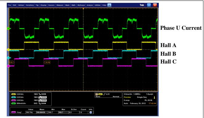
Figure 5-2 Phase U Current with Loading
