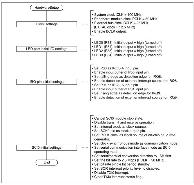
Figure 13 Flowchart (HardwareSetup) (Master)
