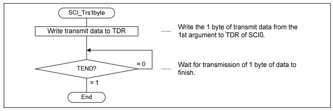
Figure 17 Flowchart (SCI\_Trs1byte) (Master)
