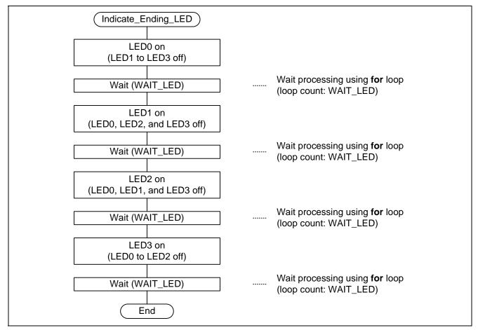
Figure 16 Flowchart (Indicate Ending LED) (Master)
