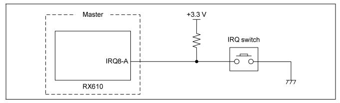
Figure 10 Master IRQ Switch Connection Diagram
