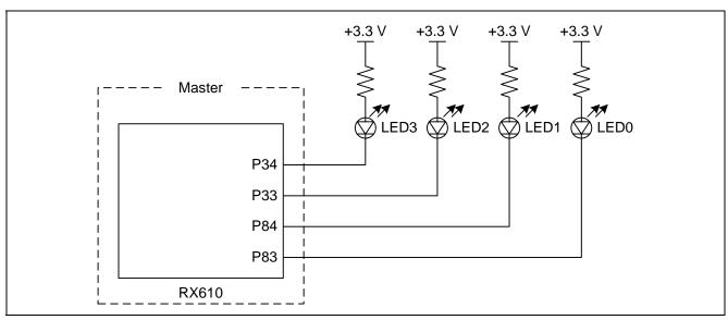
Figure 9 Master Device LED Connection Diagram
