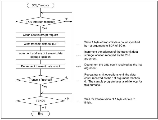
Figure 18 Flowchart (SCI\_Trsnbyte) (Master)
