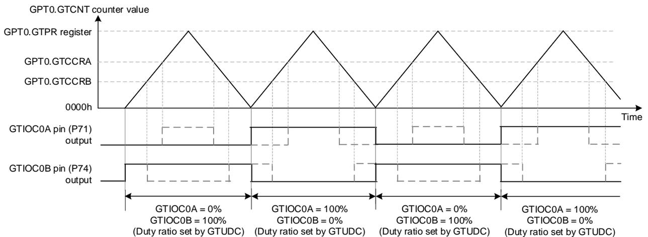
Figure 1.2 PWM Output Produced by rx24u\_gpt\_sample2
