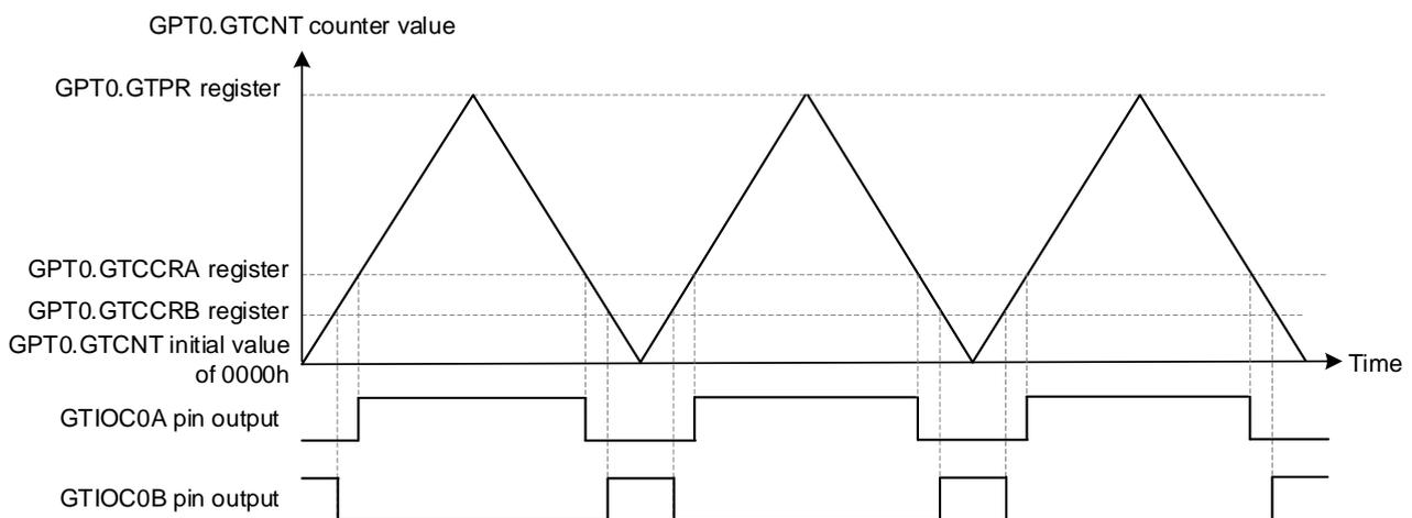
**Figure 4.1 Triangle-Wave Complementary PWM Mode 1 Signal Generation Example
