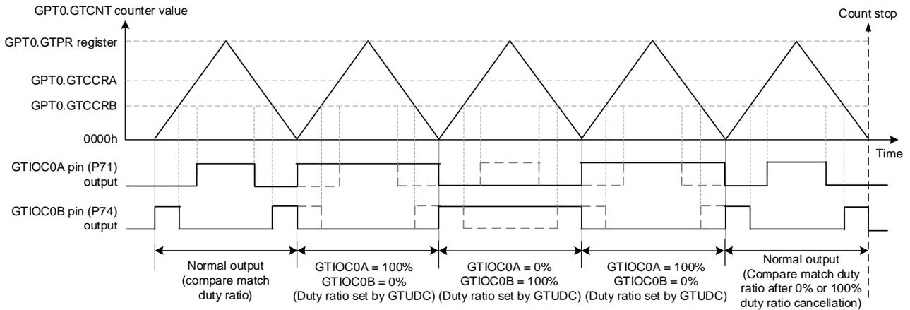
Figure 1.1 PWM Output Produced by rx24u\_gpt\_sample1
