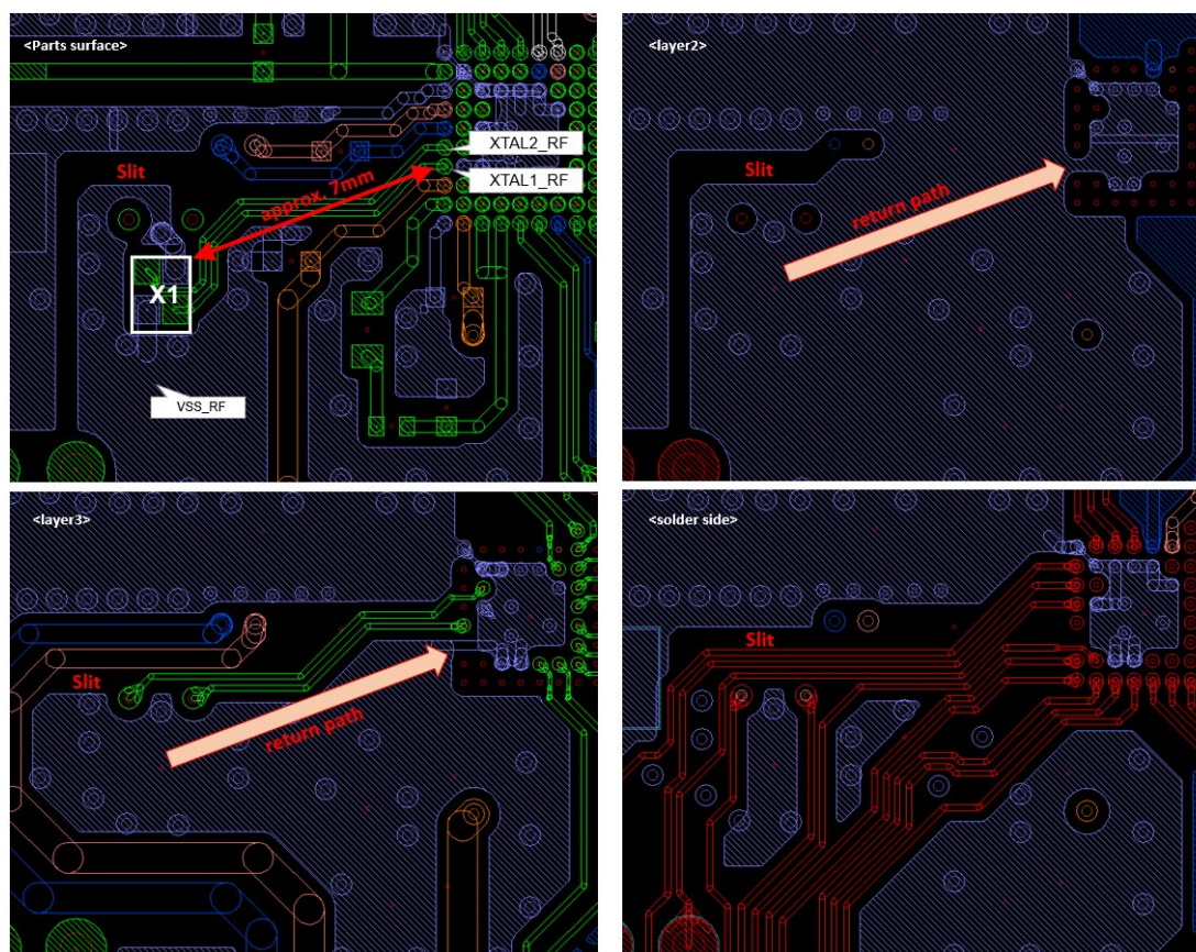
Figure 3-2 Example of the pattern around the crystal resonator
