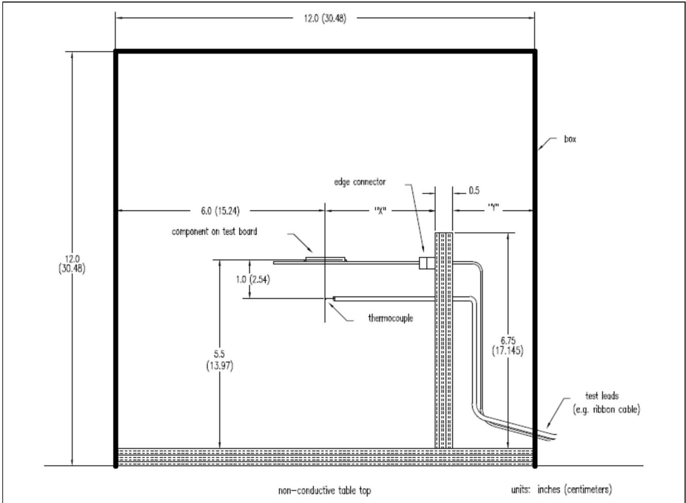
Figure 2.1 T<sub>a</sub> Measurement Position (From the EIA/JEDEC 51-2 Standard)
