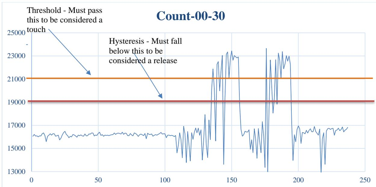
**Figure 3: Example graph showing threshold lines (in orange) and the hysteresis threshold (in red)**
