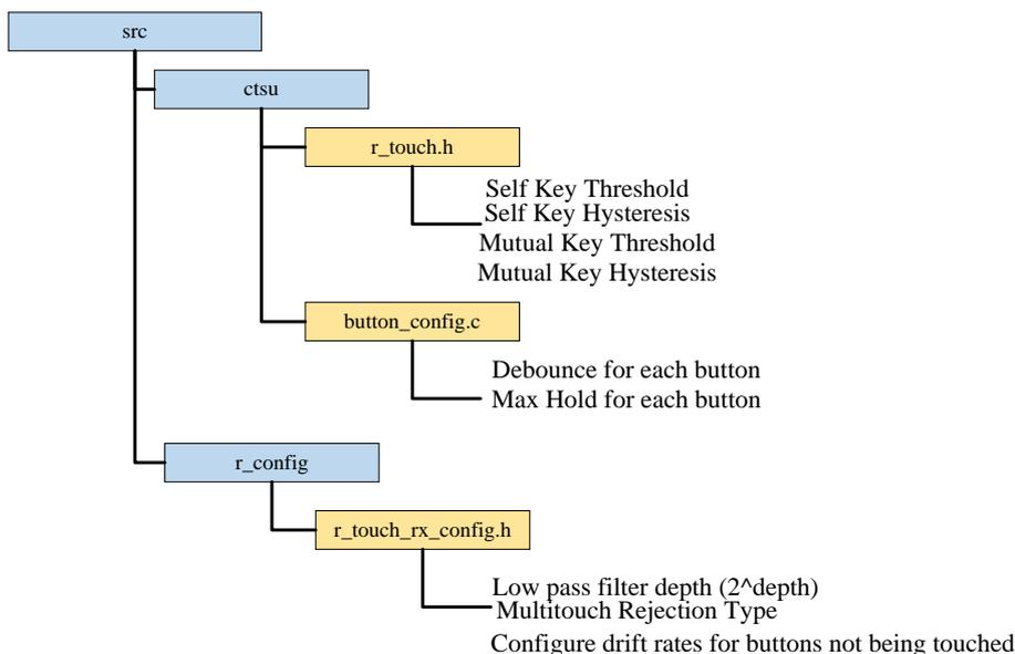
**Figure 1: File structure of the Base\_Project\_RX**
