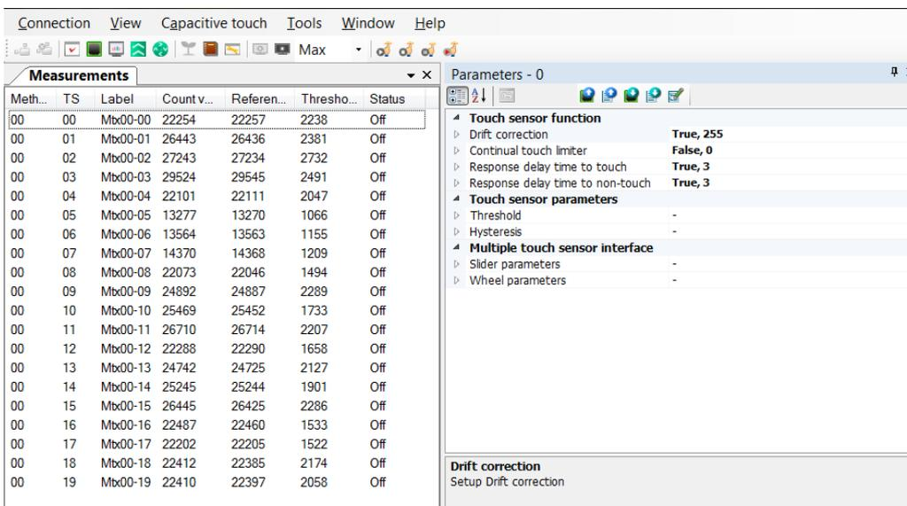
Figure 6: Workbench showing the measurement and parameter window
