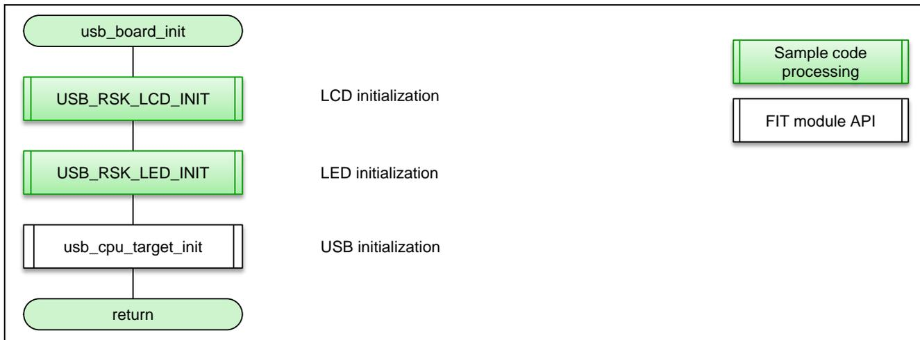
Figure 6-5 Initialization of LCD driver, LED driver and USB driver
