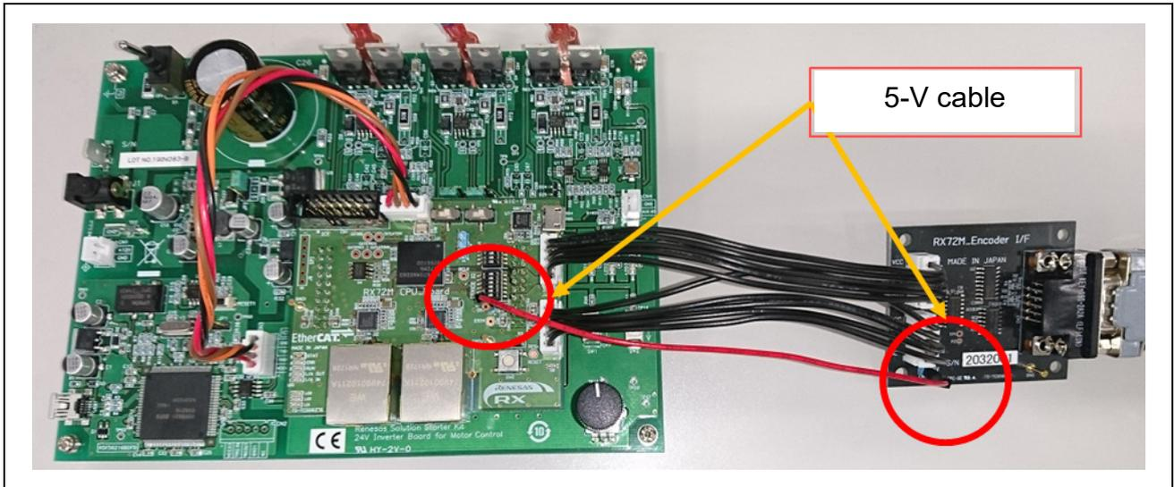
**Figure 6-3 Connection of the 5-V Power Supply**
