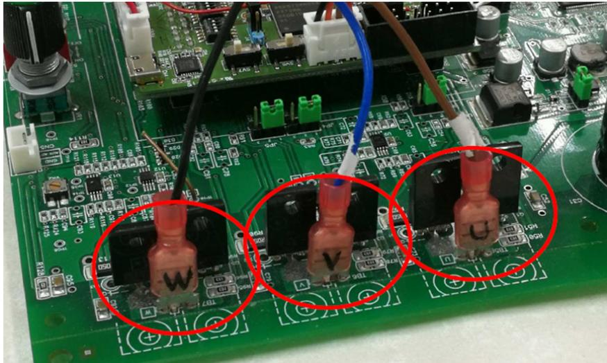
**Figure 6-1 Connection of the Three-Phase Power Lines**
