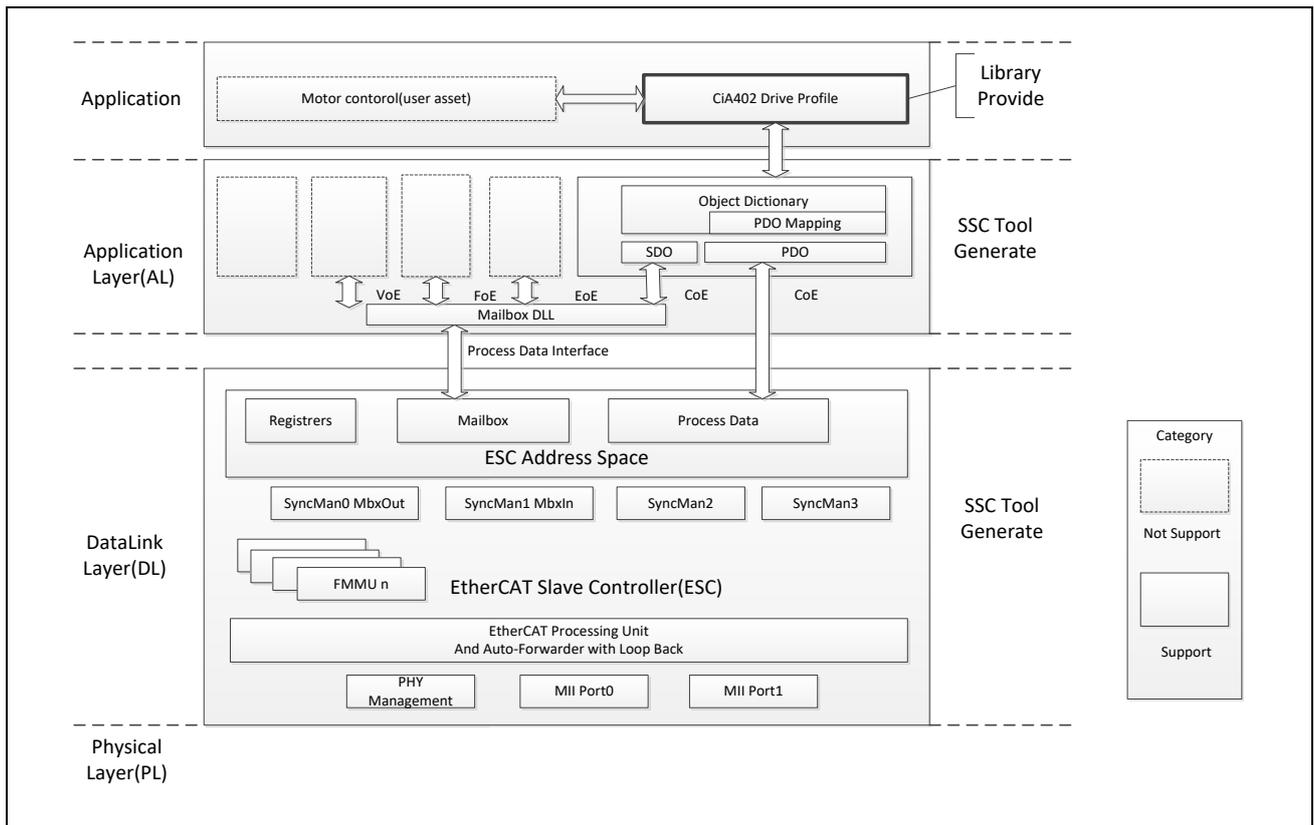
**Figure 2-3 Module Configuration of the EtherCAT Communications Program**
