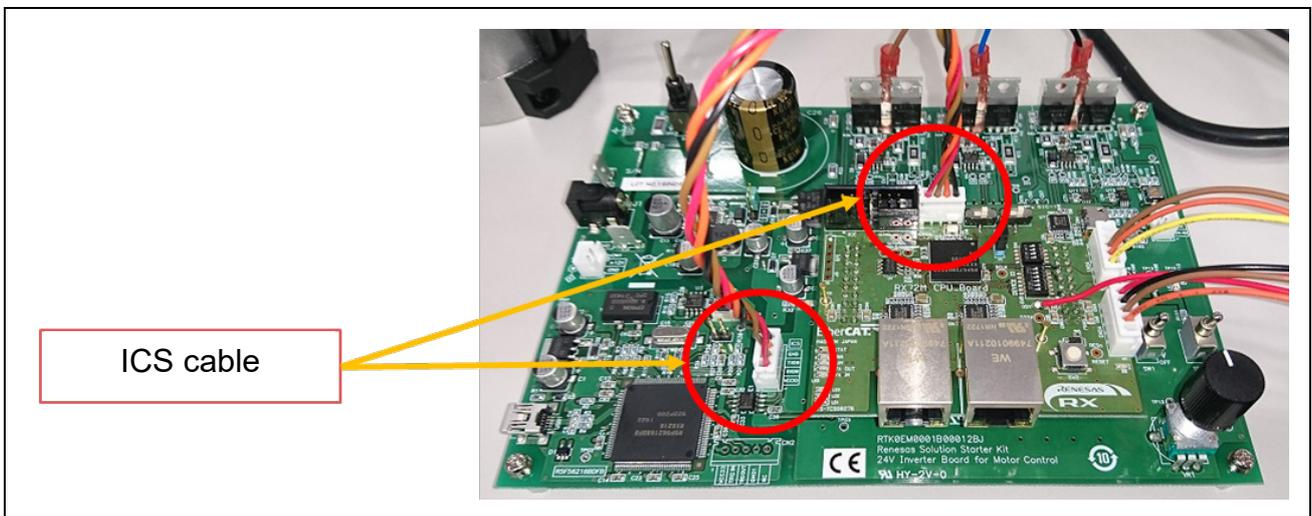
**Figure 6-4 Connection of the CPU Board and Inverter Board**
