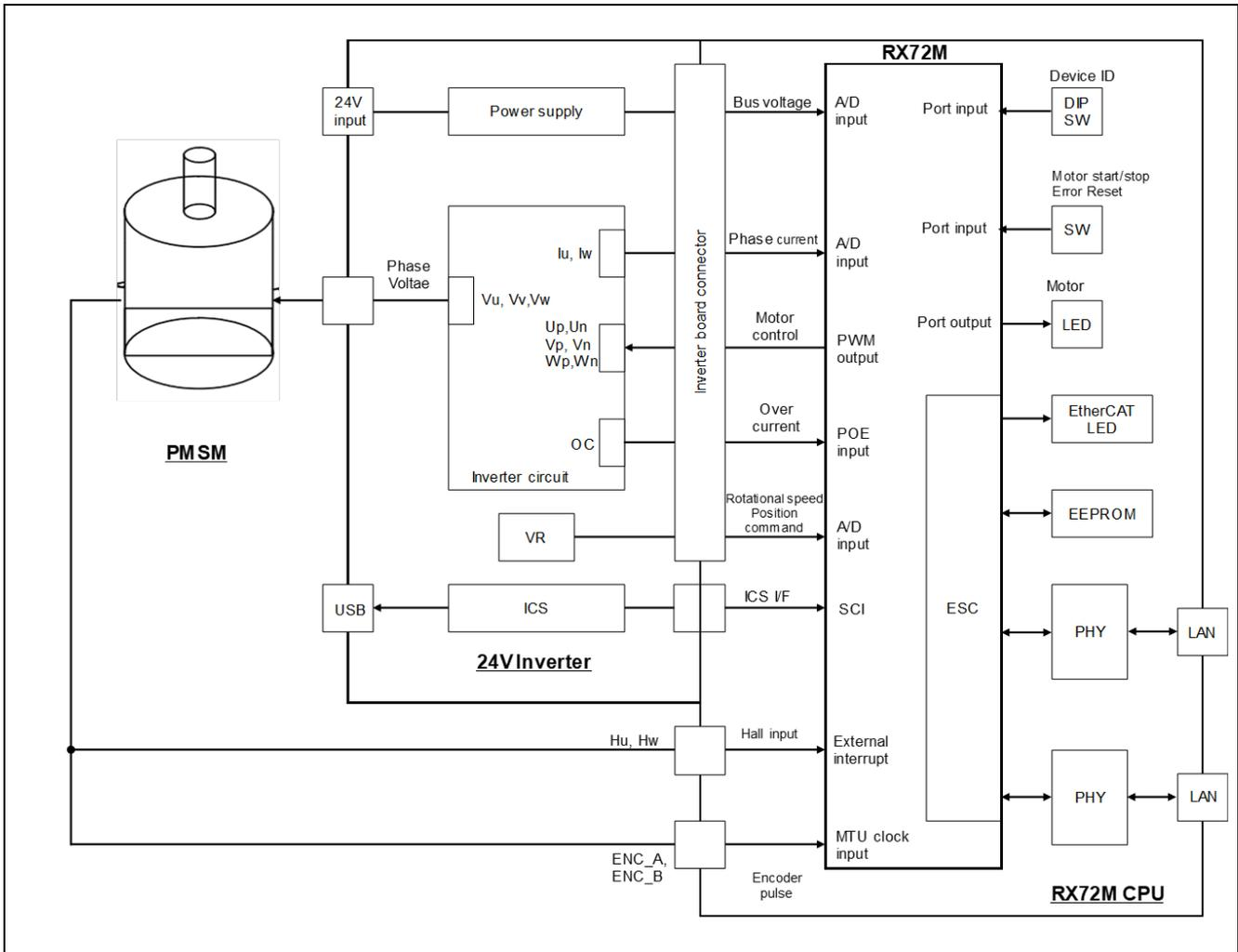
Figure 2-1 Hardware Configuration
