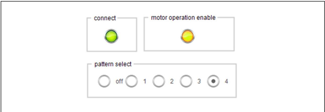
Pattern select is used to change the type of motor rotation operation.
