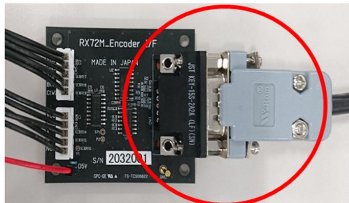
**Figure 6-2 Connection of the Encoder I/F Board**
