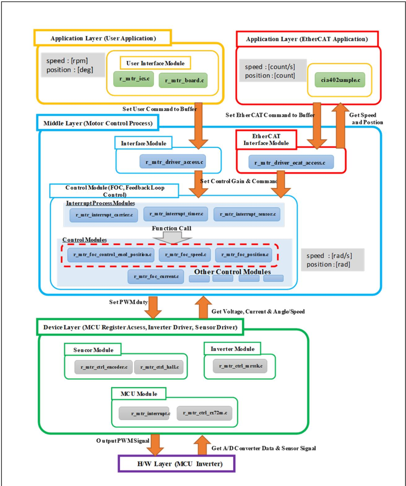
Figure 2-2 Module Configuration of the Motor Control Program
