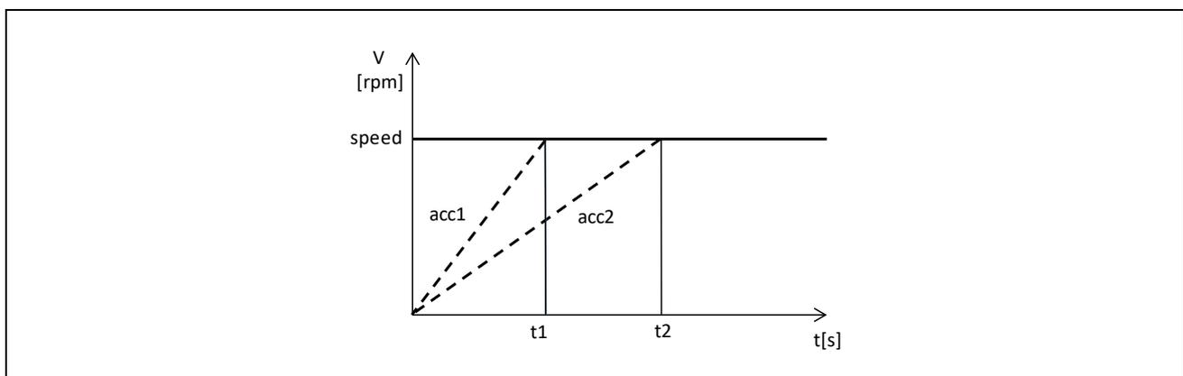
**Figure 4-1 Acceleration Times and Acceleration**
