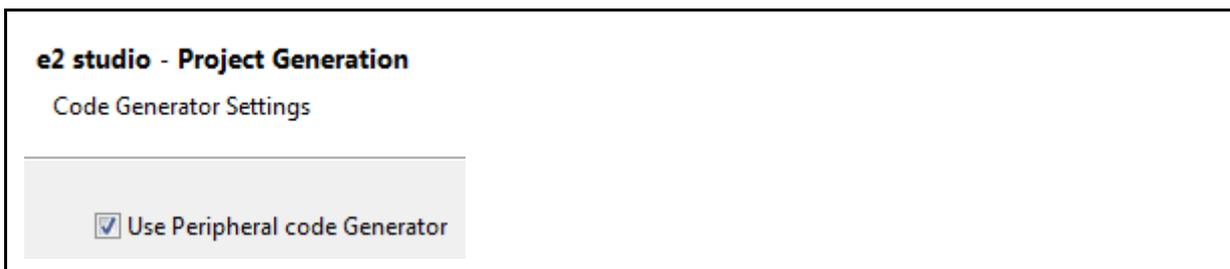
**Note:** When creating a project only for use with FIT, the box does not need to be checked, but in this case the code generator is used for the peripheral functions, so the box needs to be checked.
