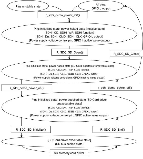
Figure 5.1 State Transition Diagram
