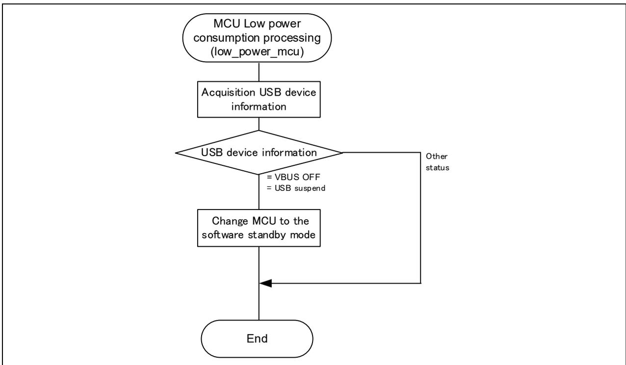
Figure 4-6 Flowchart of MCU Low Power Consumption Processing
