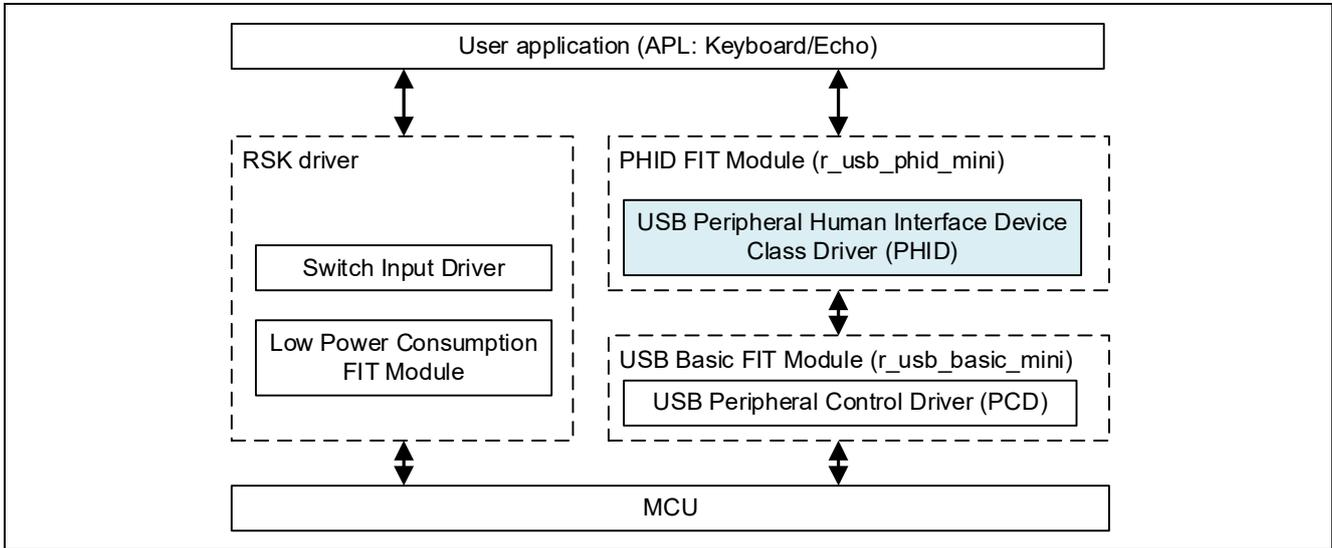
**Figure 2-1 Module Configuration**
