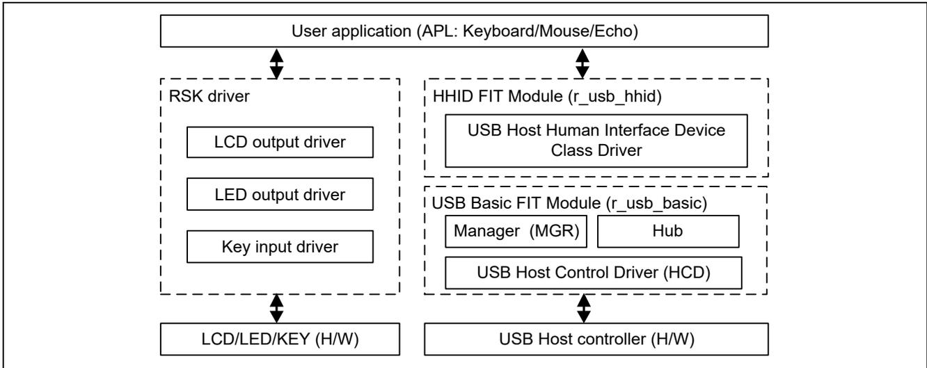
**Figure 2-1 Module Configuration**
