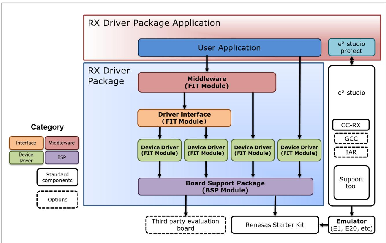
Figure 2-1 System Structure
