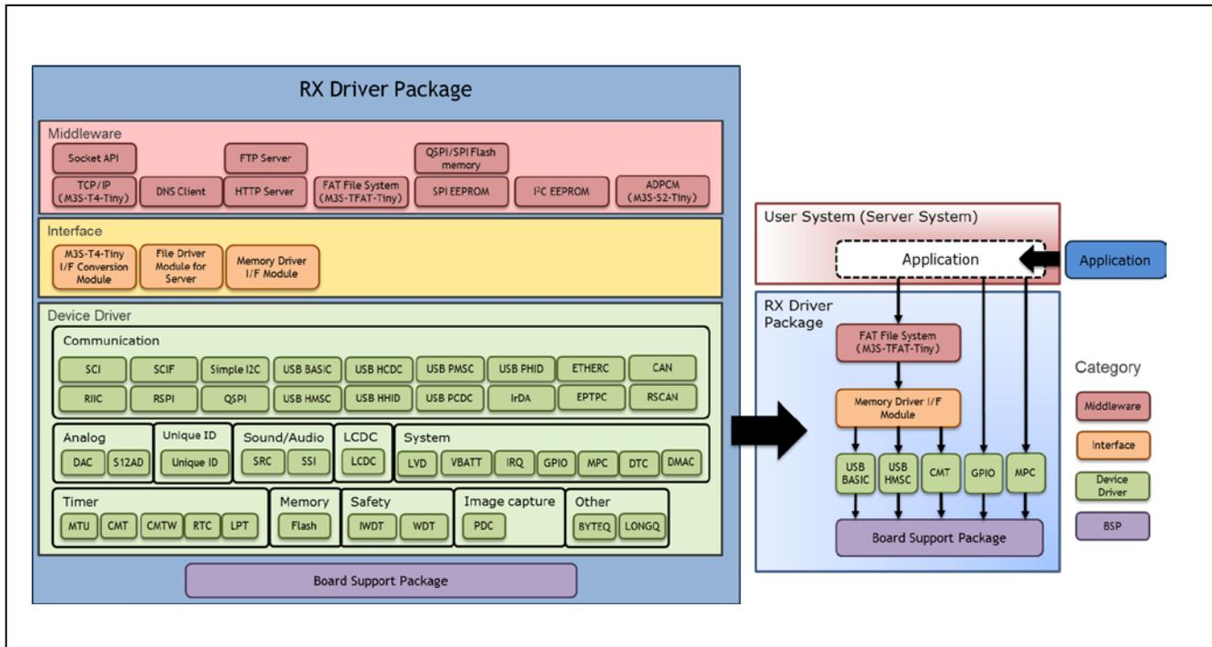
Figure 2-2 An example of system build
