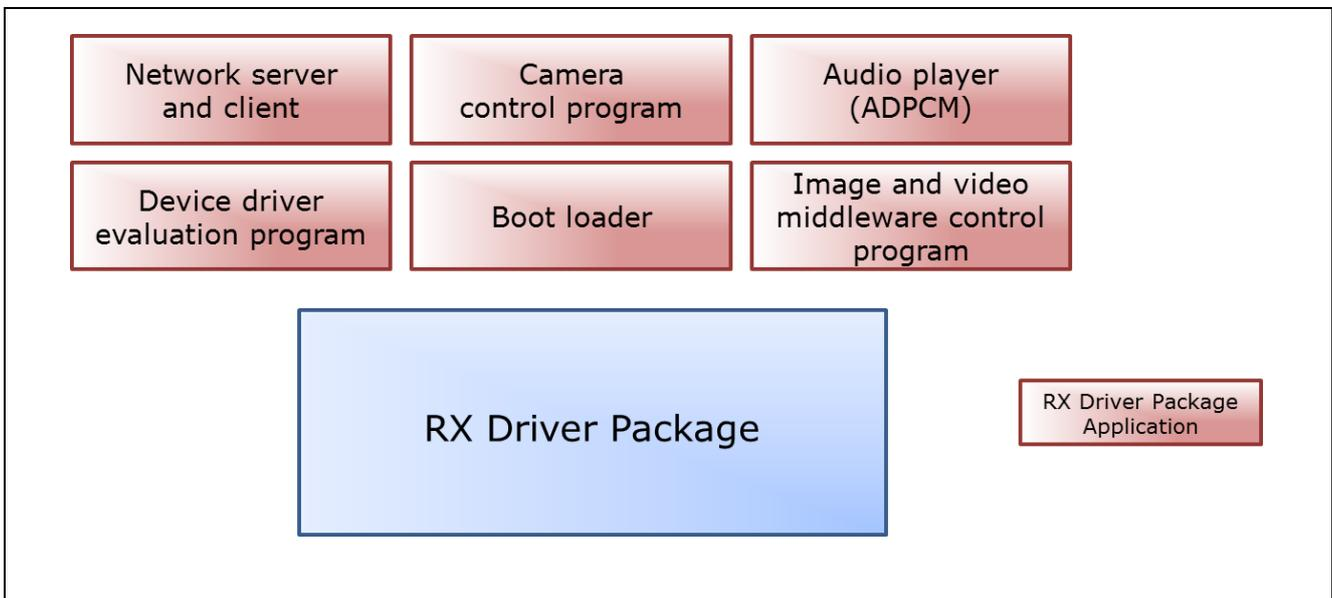
Figure 5-2 Types of RX Driver Package Application
