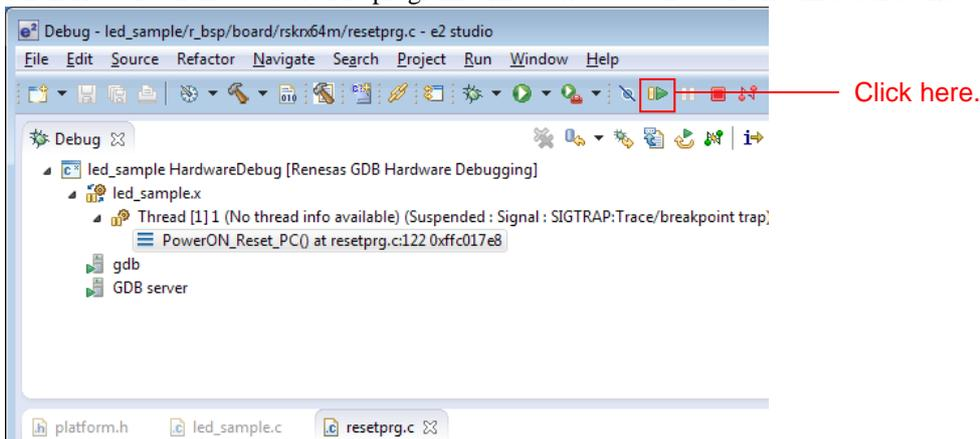
8. After the break at the start of the main function, click **Restart** on the tool bar again. The project will be run and the program will iterate toggling LED0 with a period of 0.5 seconds.
