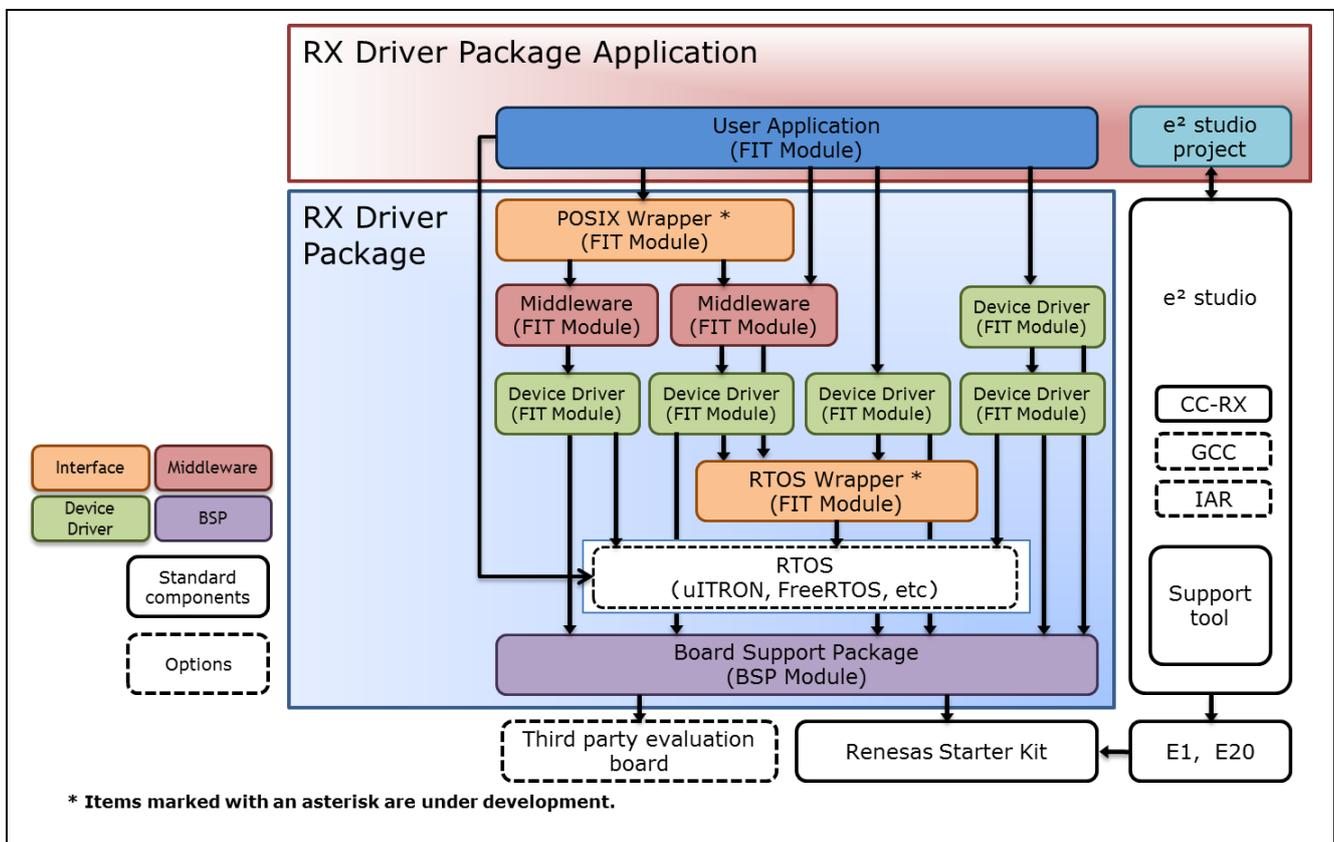
Figure 2-1 System Structure
