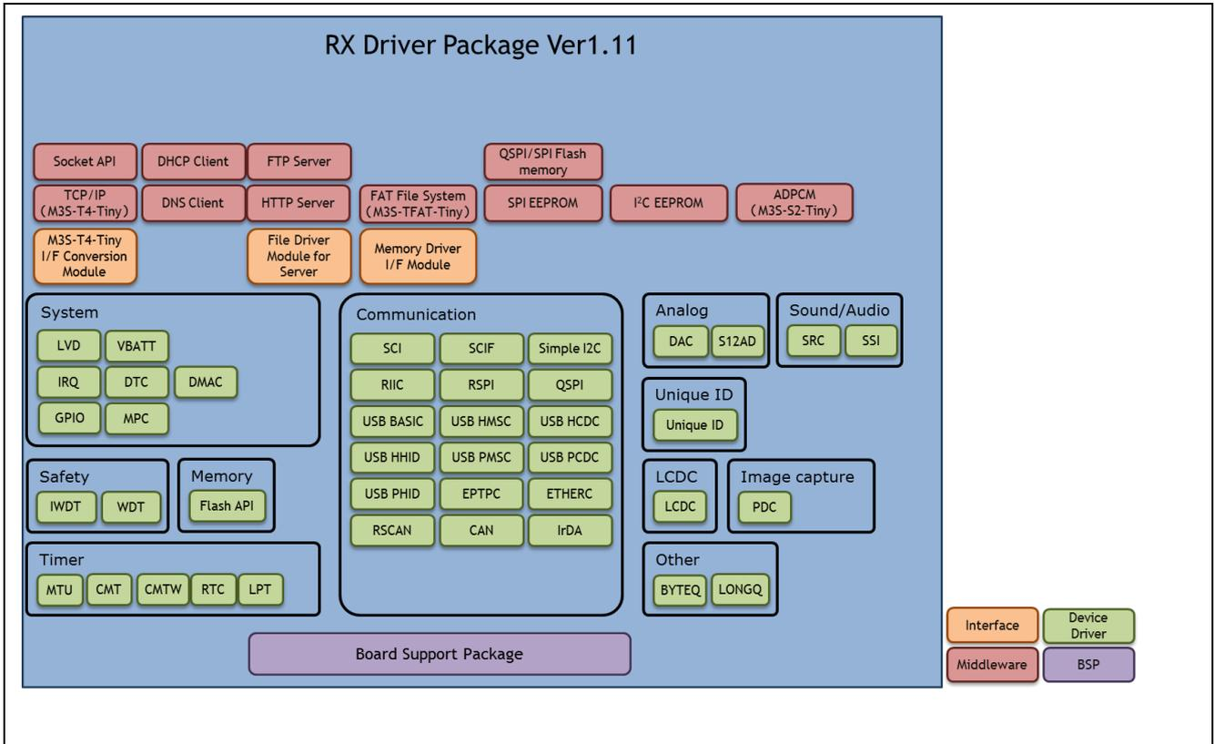
Figure 3-2 RX Family RX Driver Package FIT Module Structure
