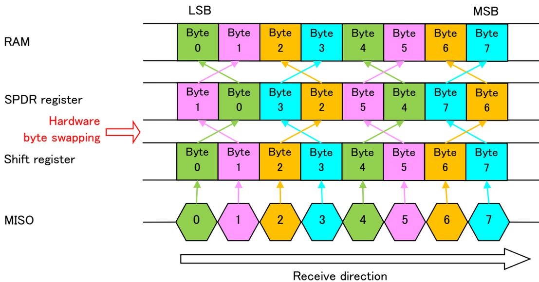
Figure 1-12 : Receiving Data 16-bit type[Little endian]hardware byte swapping
