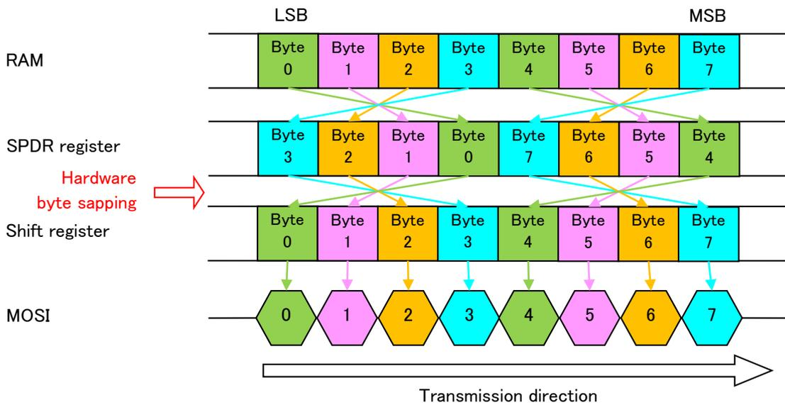
Figure 1-9 : Transmitting Data 32-bit type[Little endian]hardware byte swapping
