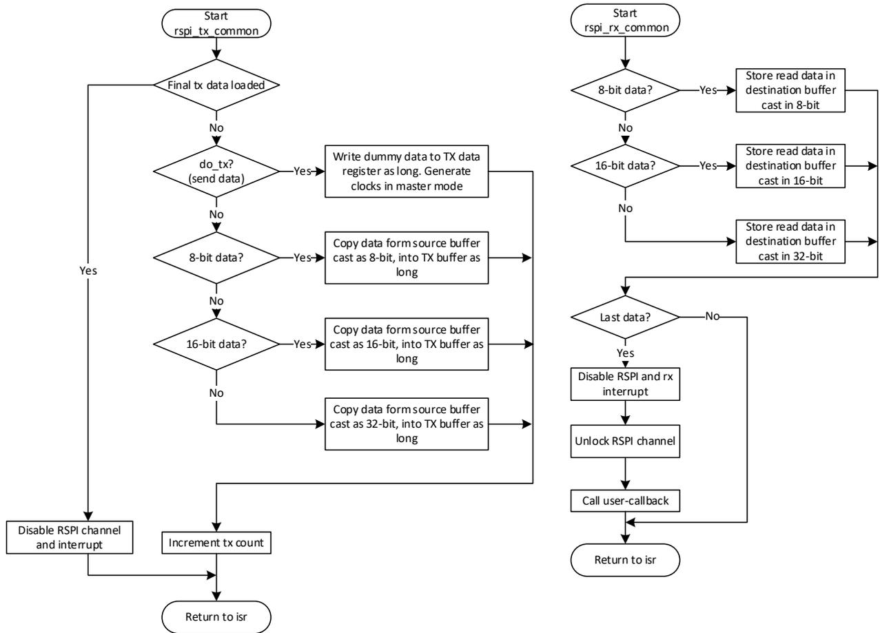
Figure 1-5 common data transmit and receive handle
