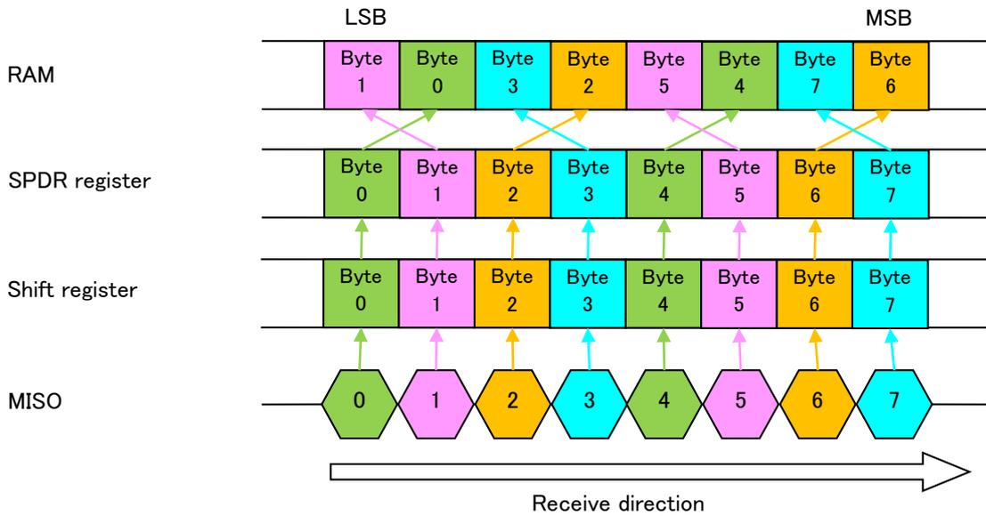
Figure 1-11 : Receiving Data 16-bit type[Little endian]No byte swapping
