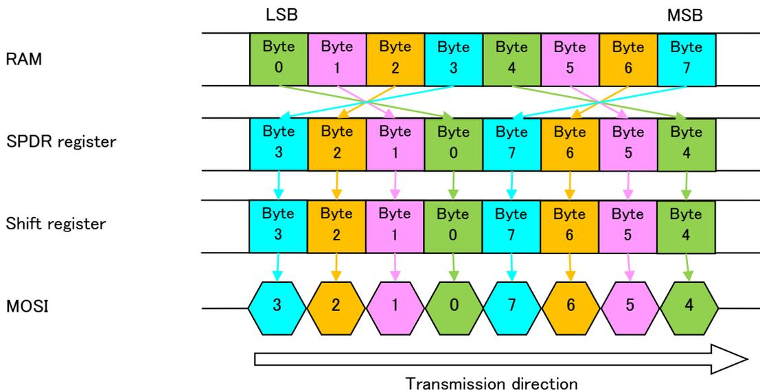
Figure 1-8 : Transmitting Data 32-bit type[Little endian]No byte swapping
