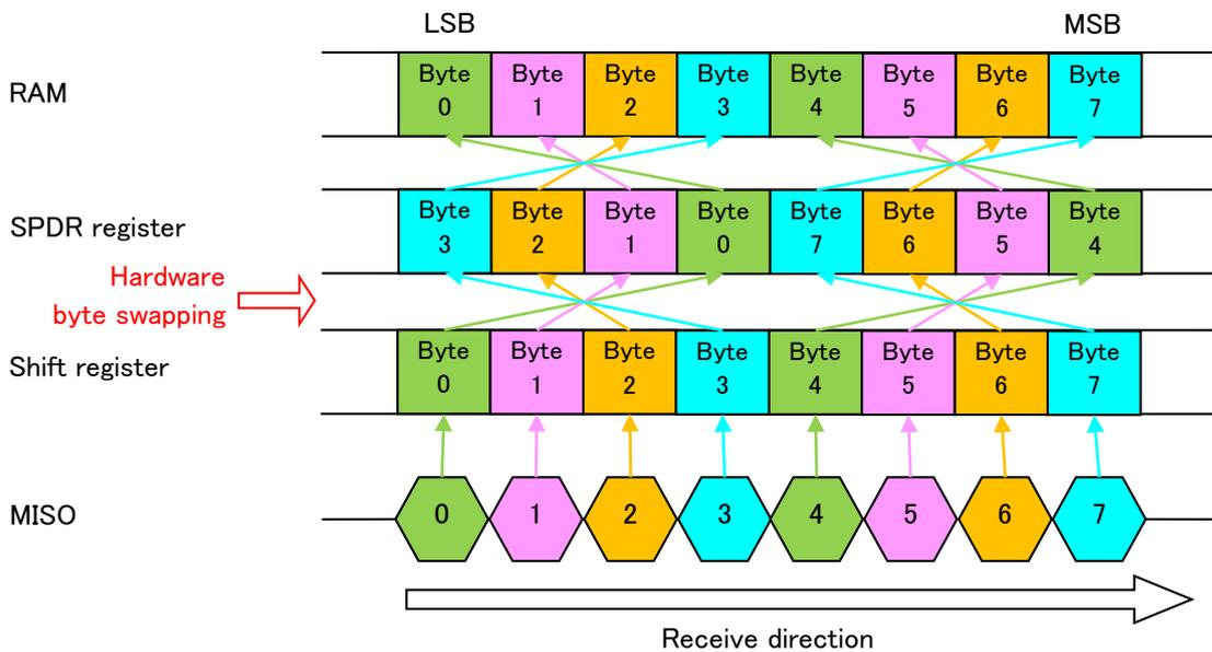
Figure 1-14 : Receiving Data 32-bit type[Little endian]Hardware byte swapping
