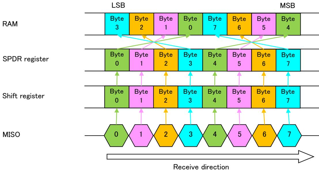
Figure 1-13 : Receiving Data 32-bit type[Little endian]No byte swapping
