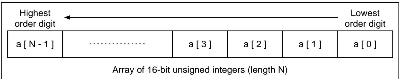
**Figure 1 Data Representation of a Multiple precision Number Using an Array of 16-bit Unsigned Integers**
