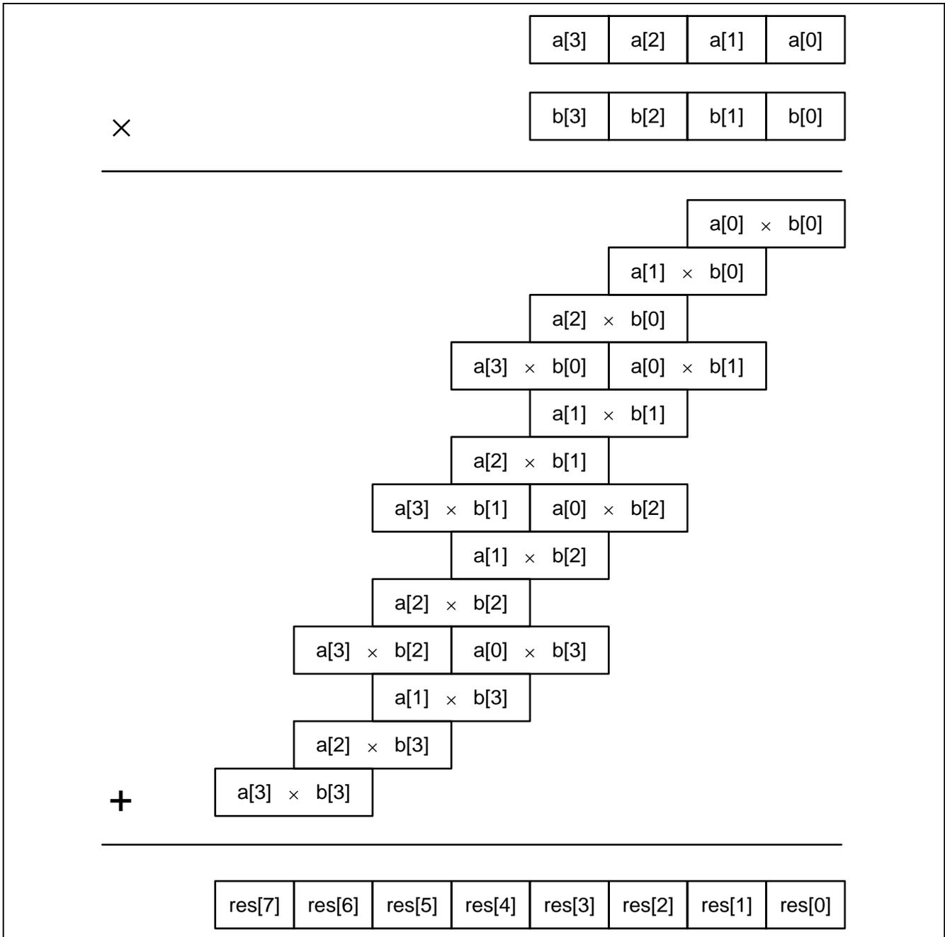
**Figure 3 Example of Multiple precision Multiplication on Paper (4 Digits × 4 Digits)**
