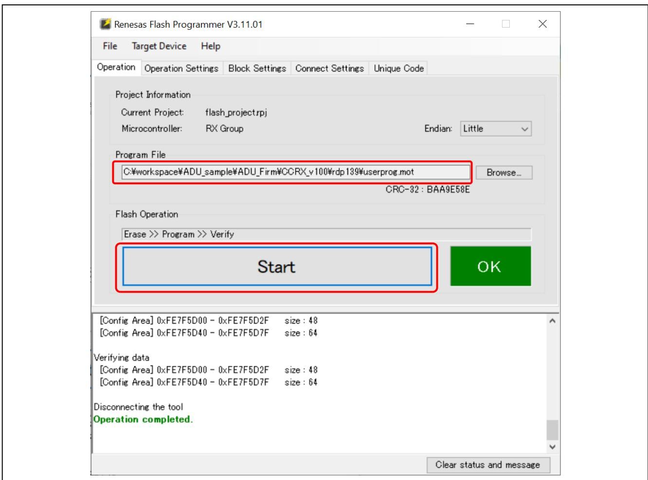
Figure 2.33 Programming the Initial Firmware to the Device
