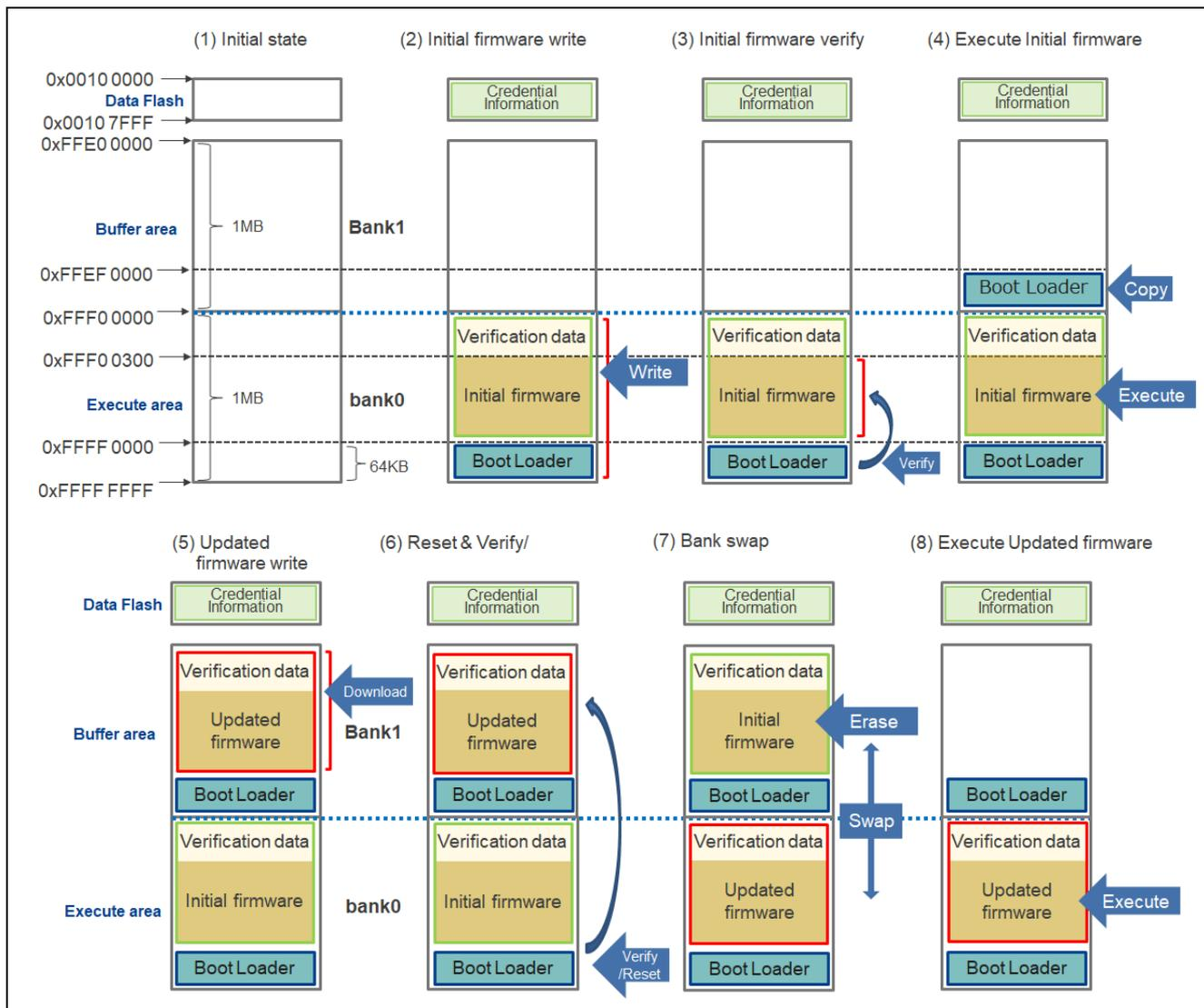
**Figure 1.1 Memory Allocation for ADU (If the Version is v1)**
