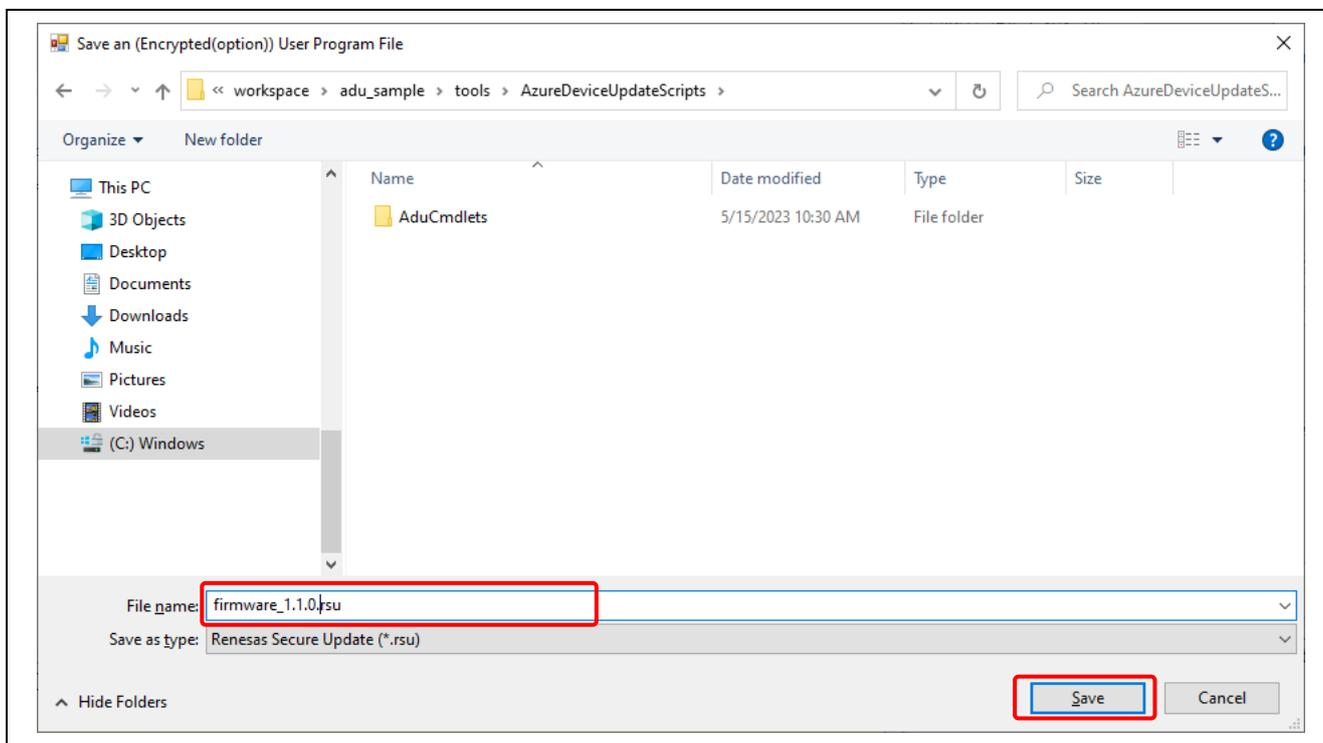
**Figure 2.39** Outputting an RSU File of the Update Firmware
