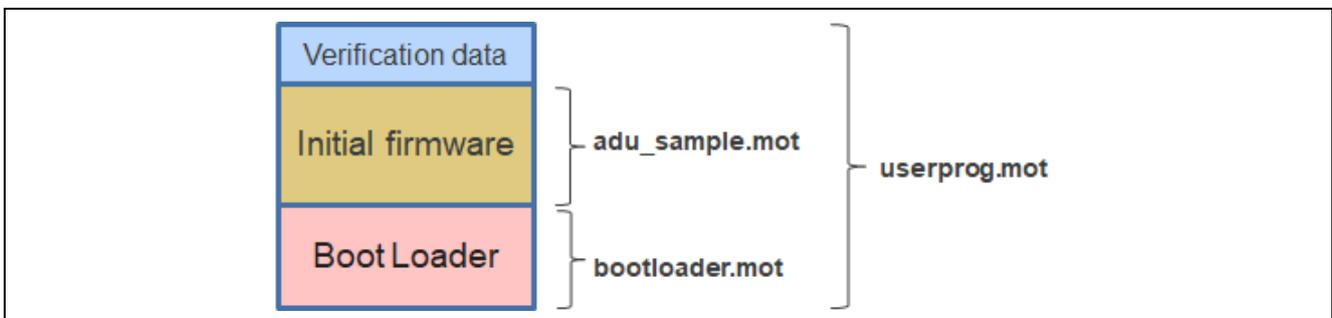
**Figure 2.31** File Configuration of userprog.mot (for Firmware Update Module v1)
