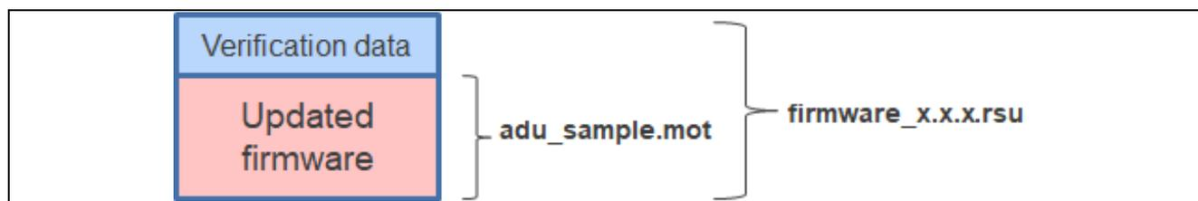
**Figure 2.40** Configuration of the RSU File of the Update Firmware (for Firmware Update Module v1)
