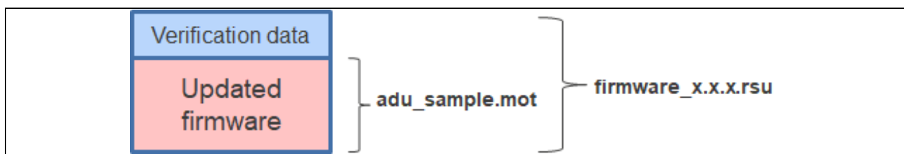
Figure 2.40 Configuration of the RSU File of the Update Firmware (for Firmware Update Module v1)
