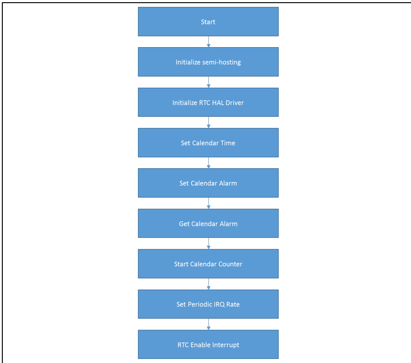
Figure 5 RTC Application Project Flow Diagram
