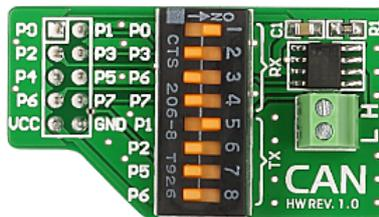
It is recommended to solder a 2x3 header across J2 pins 15-20 on the RSKRX24T. Dip switch lines 1 and 5 should be in the ON position on the CAN-1 board. Connect the boards in the following manner:
